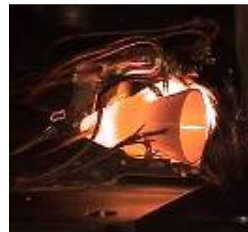
Kill Vehicle Hot Fire Test
