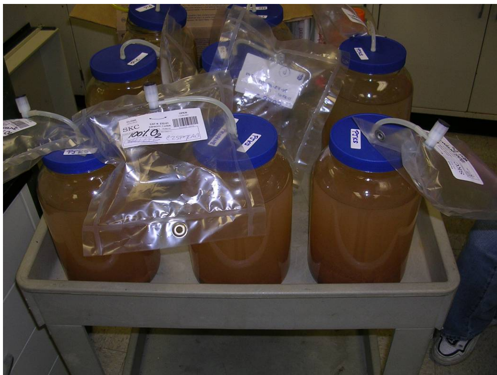
Figure 60. Photograph of large-scale microcosms. Tedlar bags contain oxygen or a mixture of oxygen and propane gas.
