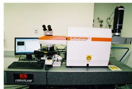
Figure 5.8. Photograph of the new Renishaw Reflex Invia micro-Raman spectrometer commissioned in 2008.
