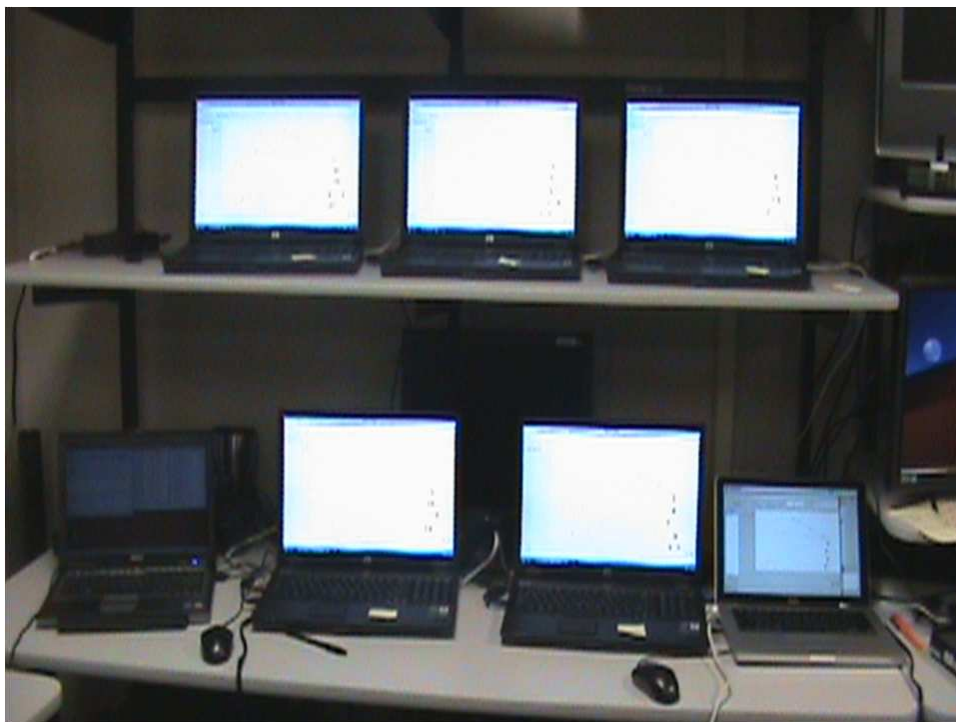
Figure 4.20: Actual picture of the second execution scenario which is composed of NS-2 running on linux operating system, the mediator , five NetViz clients running on windows operating system and one NetViz client running on Mac operating system.
