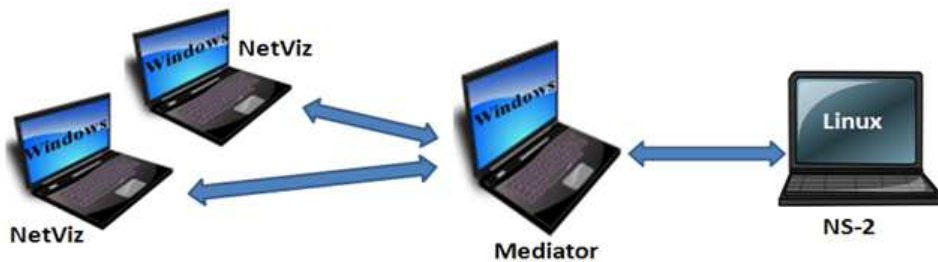
Figure 3.22: An illustration of the execution scenario which is composed of NS-2 running on linux operating system, the mediator , and two NetViz clients running on windows operating system.
