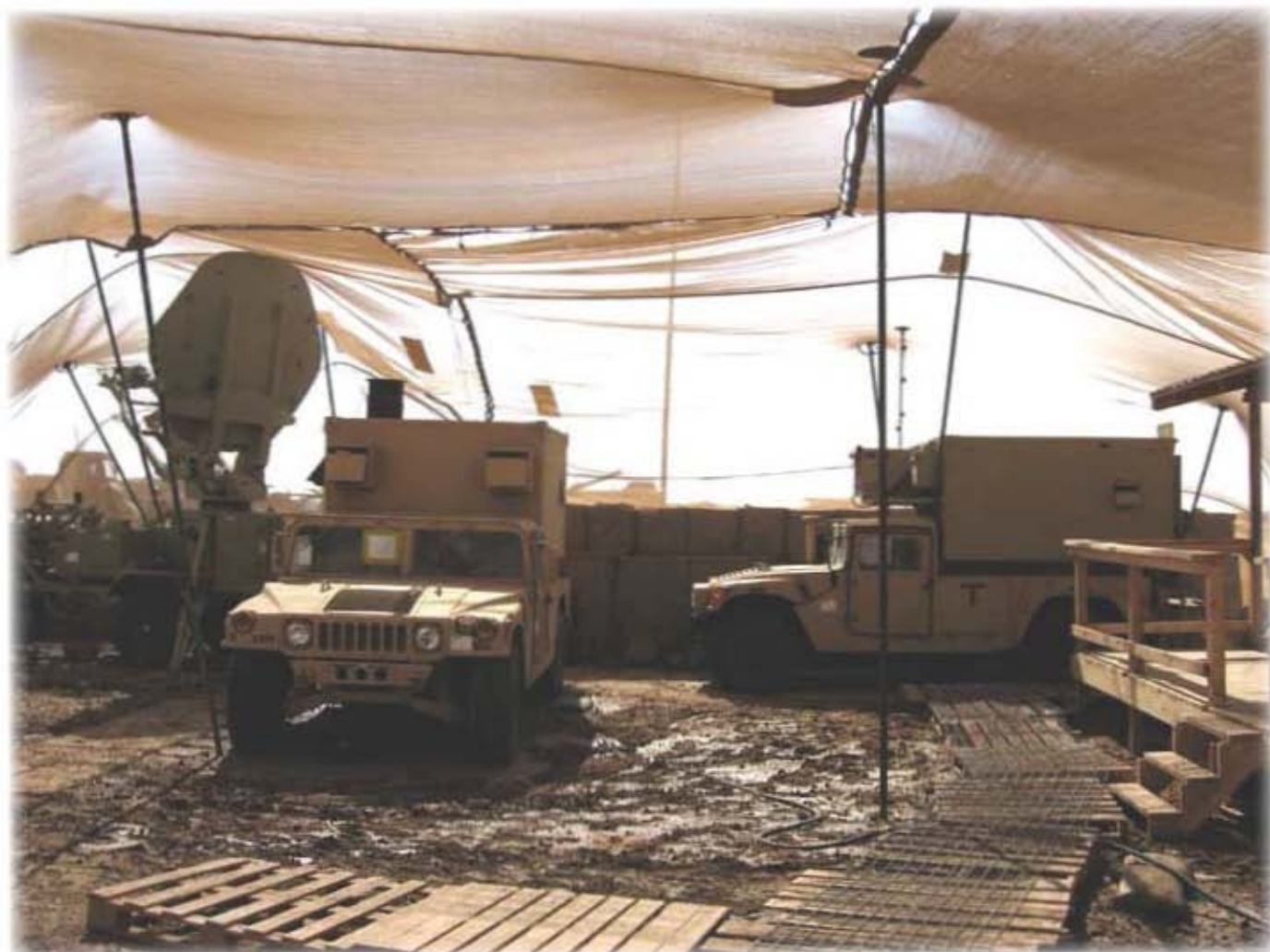
Solar shades were used to mitigate heat around the equipment. Wooden pallets were necessary to prevent the mud buildup in traffic areas.
