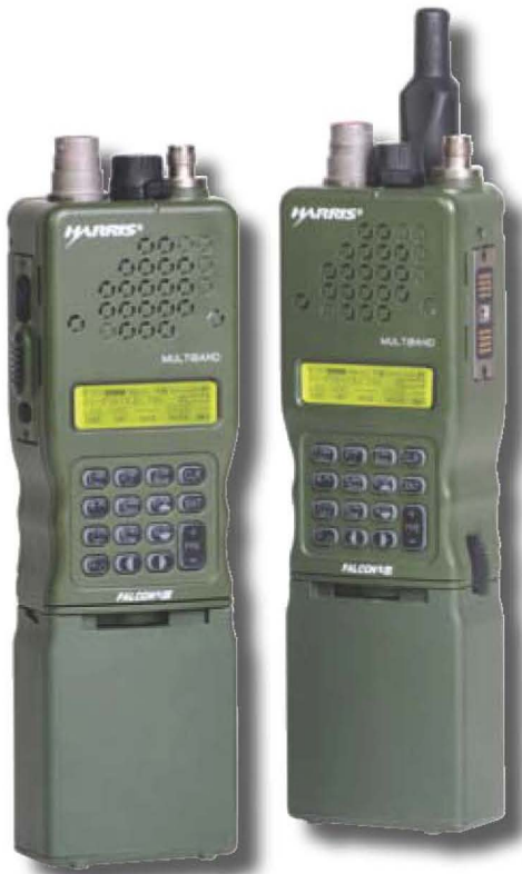
Figure 1. AN/PRC-152 Multi-Band hand-held radio is shown. AN/PRC-152 Multi-Mode Multi-Band hand-held radio is also selected as part of the Consolidated Interim Single-Channel Hand-held Radio family.
