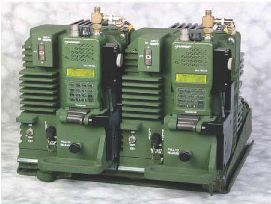
Figure 5. AN/VRC-110 consisting of 2 AN/PRC-152s on a dual vehicular mount. Frequency range 30-512MHz, maximum power out 50 watts.
