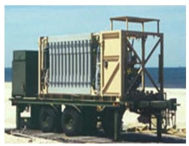
This Army-managed system (B2605) is replacing the old system. It is a self-contained and mobile system capable of producing 1,500 gallons of potable water per hour from fresh, brackish, salt, and nuclear, biological, and chemical contaminated fresh water.
