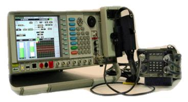
This test set (A7082) is used at fixed facilities, such as repair depots and intermediate maintenance facilities.
