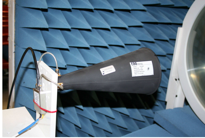
Figure 3.8: Two ports for orthogonal polarization connected to routing switch.
