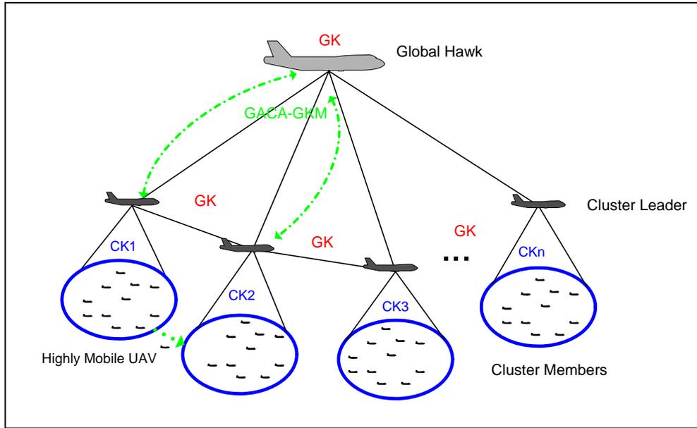
Figure 8. Hubenko Architecture Applied to UAV Swarm [Phi08]
