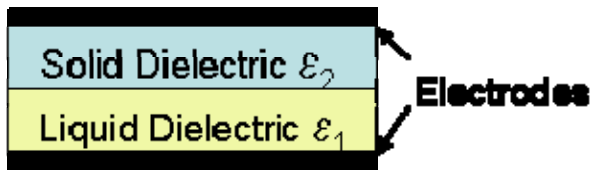
Figure 5: Parallel plates separated by two dielectric layers.
