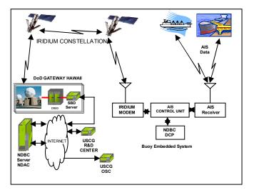
Figure 1. Block Diagram of Buoy AIS system
