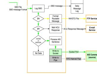
Figure 2. Shore-side Data Processing Flow
