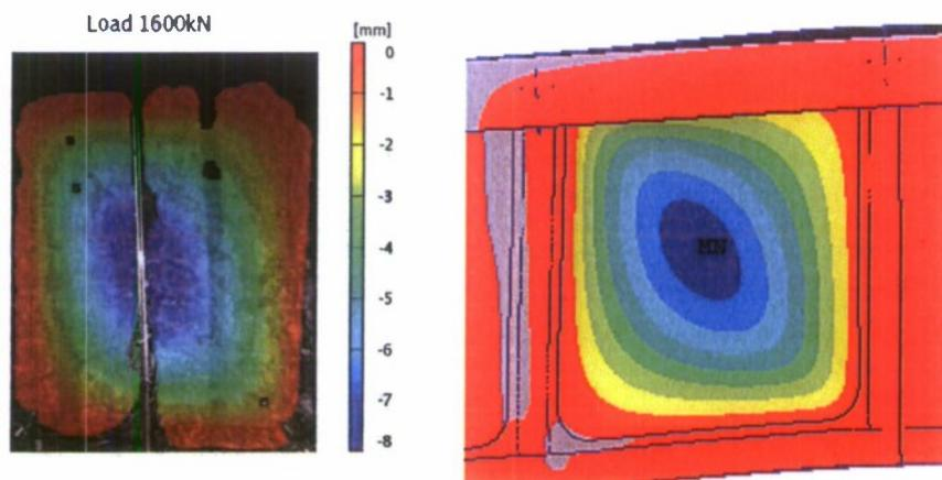
**Fig. 8.** Comparison between measured (left) and calculated (right) out-of-plane deformations.
