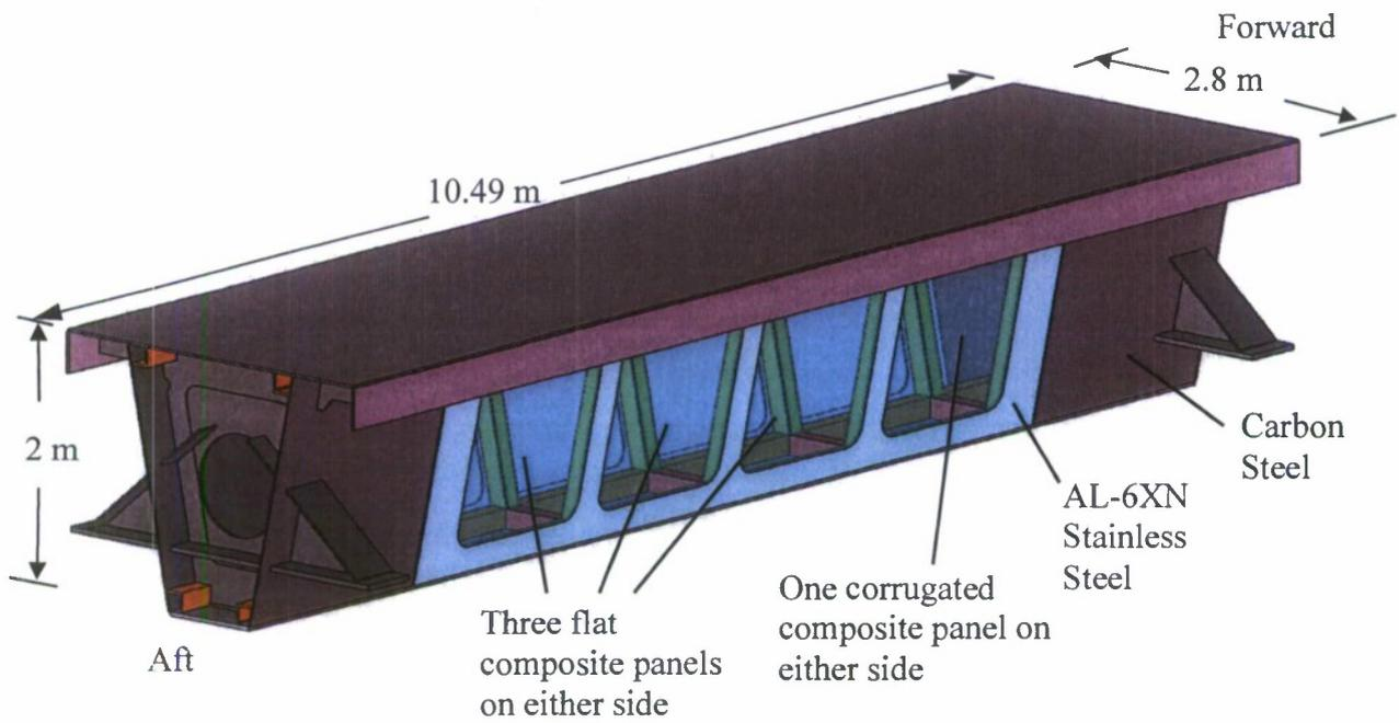
**Fig. 2.** CAD model of hybrid girder.
