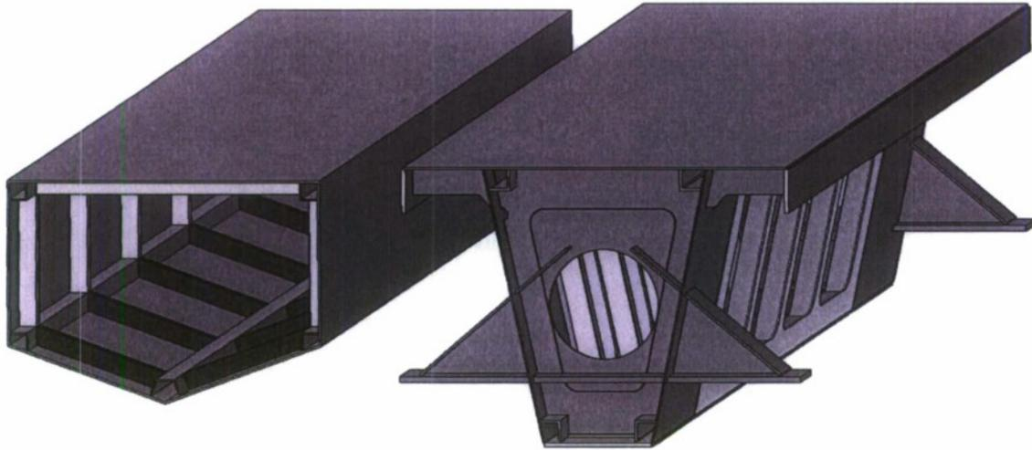
**Fig. 4.** Scaled down (1:8) destroyer (left) next to the presently studied girder (right).
