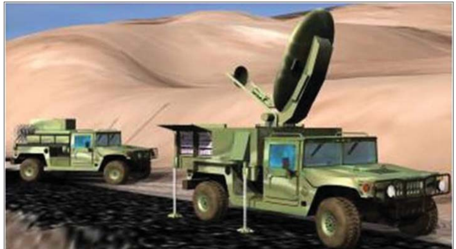
The Phoenix, an SHF Tri-Band SATCOM terminal, was introduced in the Summer 2003 Army Communicator TSM Update.
