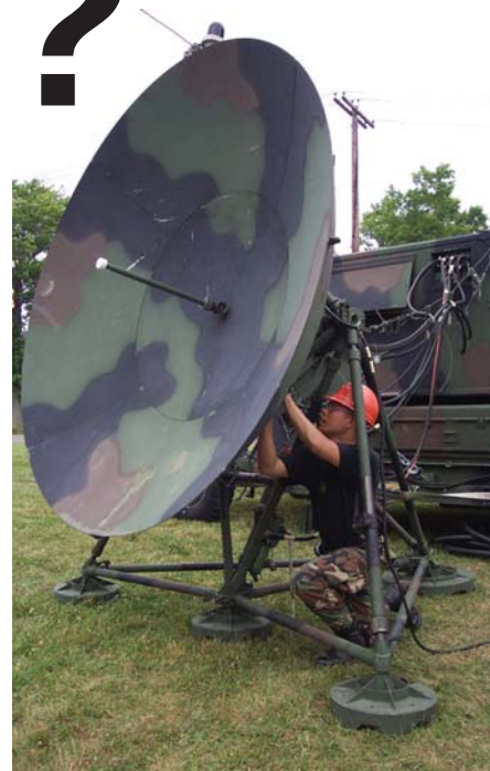
SSG Rachapreuk J. Schmidt, 103rd Air Control Squadron, Connecticut Air National Guard, performs some quick troubleshooting and manually adjusts a satellite antenna with a malfunction in its motor control.
