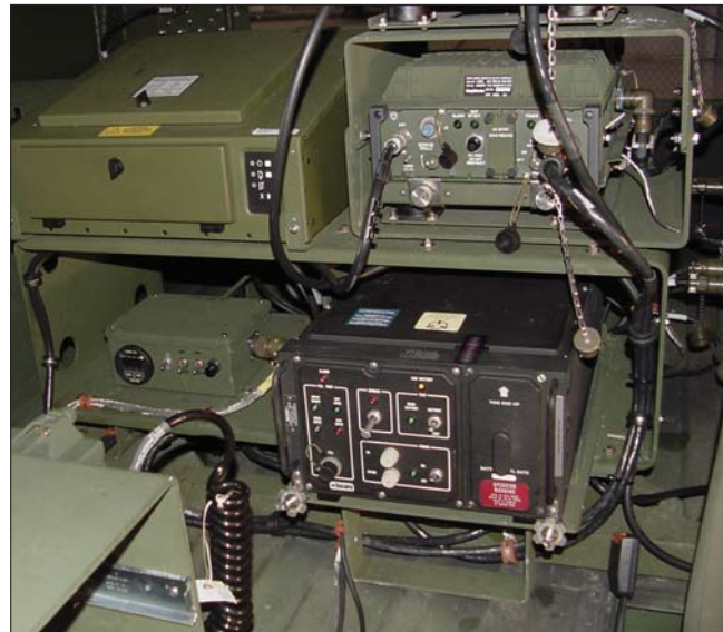
Top shelf left to right: printer and EPLRS RT. Lower shelf right side: KOK13.
