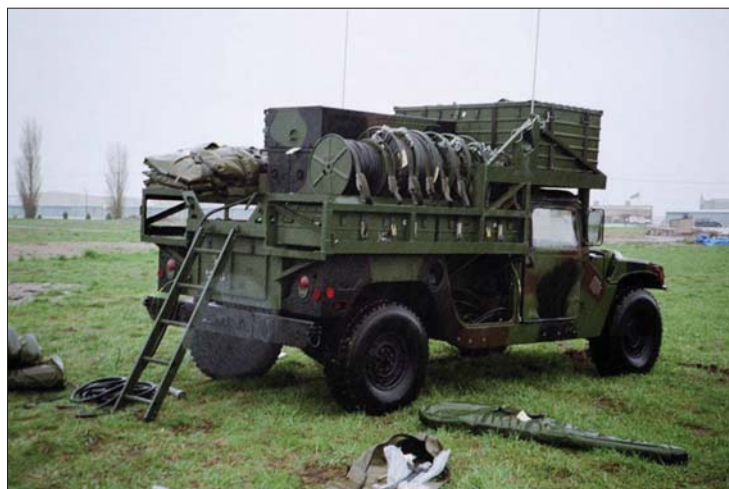
Phoenix, Block 1 Mobile Power Unit carries a 10 kW Tactical Quiet Generator. above.
