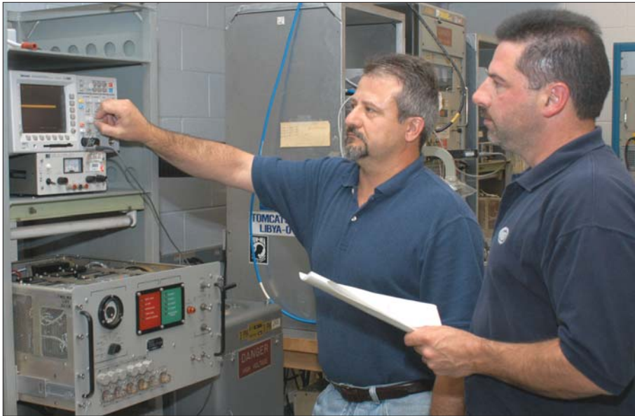
Mark Williams and Tom Ondrey test a modified power supply for the AN/TSC-100A tactical satellite terminal at Tobyhanna Army Depot. Their modification allows the transistors to work properly in the power supply, significantly reduces the amount of time required for individual transistor testing and improves the performance of the power supply. Williams is an electronics mechanic in the depot's Satellite Communications Directorate and Ondrey is an electronics engineer in the Production Engineering Directorate.
