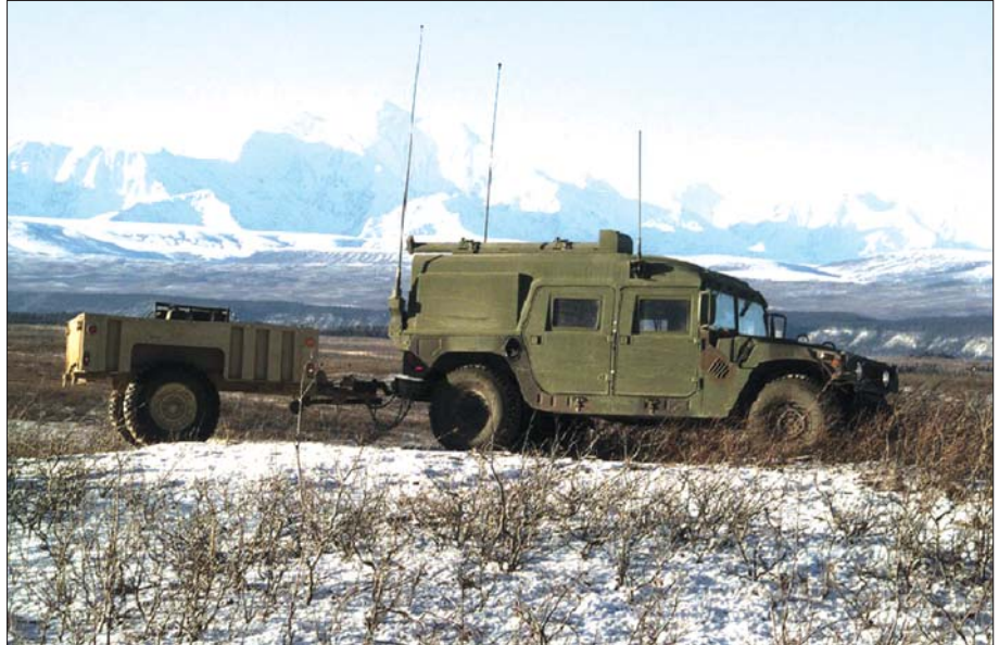
The EPLRS Manager vehicle is a humvee modified to support the EPLRS ENM mission.
