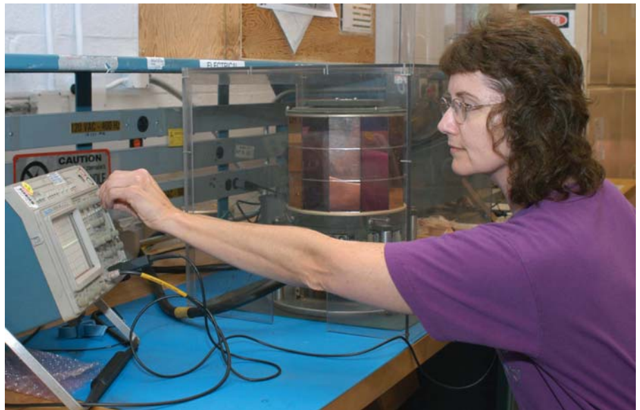
Rosalie DelJanovan carries out a final electrical test on an AN/ALQ-144 Infrared Jamming System. She is one of 47 personnel in Tobyhanna Army Depot's Aircraft Survivability Equipment Division, Avionics-Intelligence Electronics Warfare Directorate, who repair and test the system. Depot technicians have reduced cost while meeting significantly increased workload for the aircraft defense system. DelJanovan is an electronics worker.
