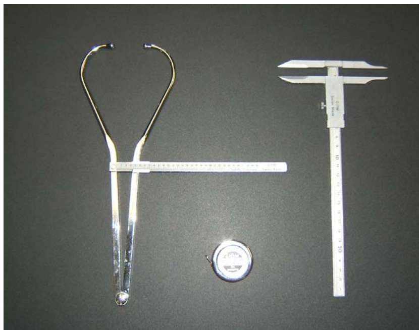
Figure 2. GPM sliding caliper, Lufkin steel tape, and GPM spreading caliper.
