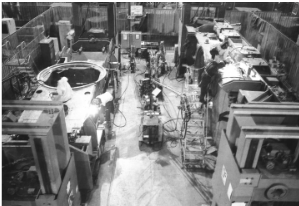
Egyptian workers perform welding operations on two M1A1 tank hulls. Under this coproduction program, all operations necessary to complete the vehicles are performed by trained Egyptian tank plant workers.
