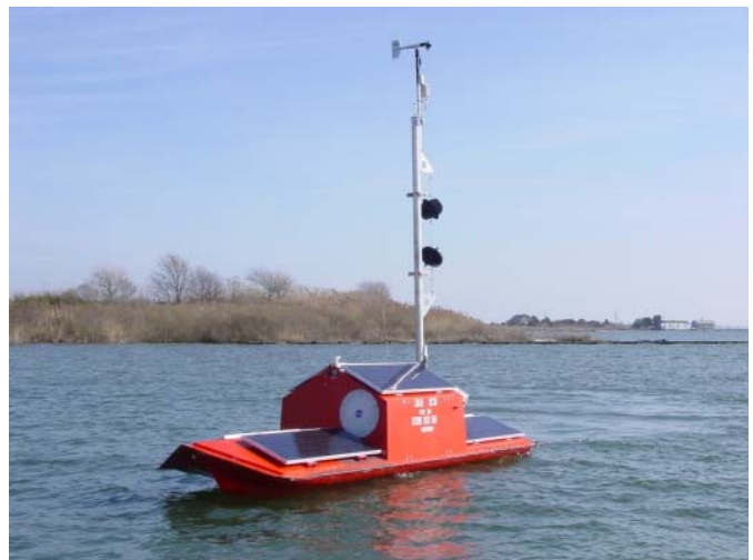
Figure 1. The Ocean Atmosphere Sensor Integration System (OASIS) ASV.
