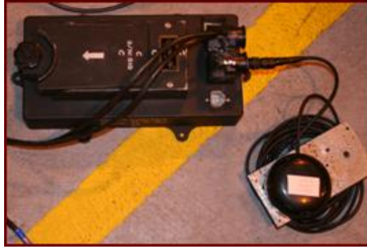
Figure 9. Computer Aided Central Timing Unit system (CACTUs)(From Pierce, 2008)
