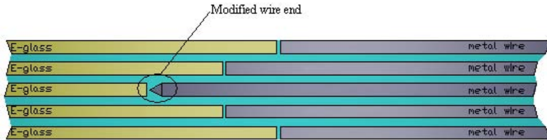
Figure 48. Design Modification for Symmetric Stepped-Lap Joint.
