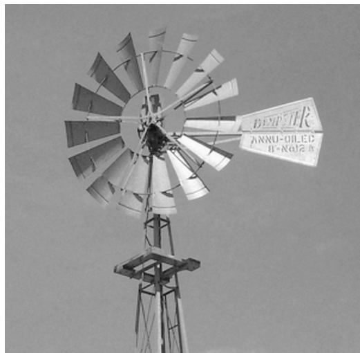
Figure 4. Multi-Blade HAWT (From Kreith 2007)
