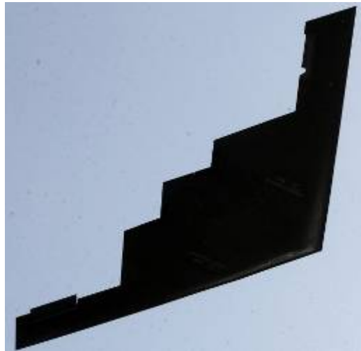
Figure 50. The Engine Nozzles of B-2 are Concealed to be Seen from Below (From [76])
