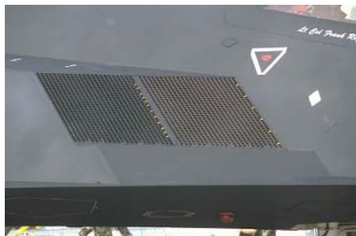
Figure 56. Thin Mesh Grids, at the Engine Intakes of F-117 (From [81])
