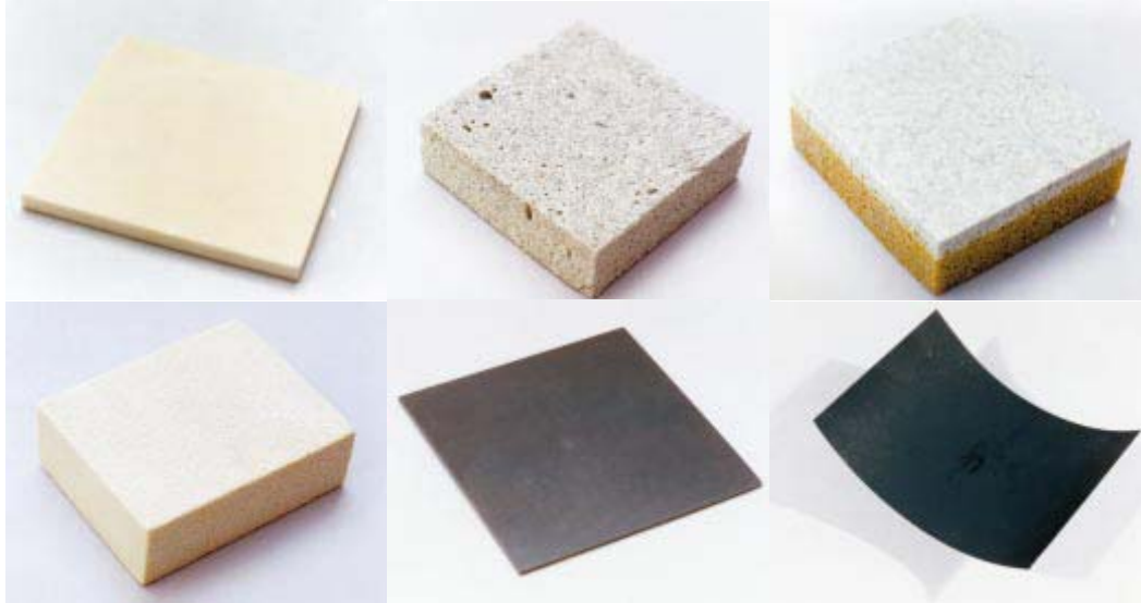
Figure 38. Four Thick Radar Absorbing Material Foams and Two Samples of Thin Radar Absorbent Sheets (After [61])
