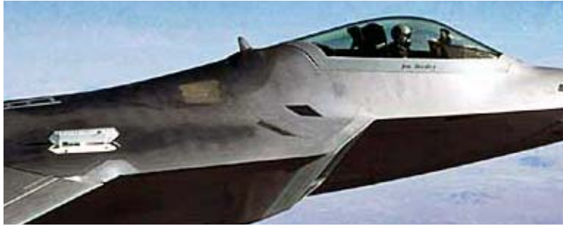
Figure 32. An Opening Door Covers the Muzzle to Preserve the F-22 Raptor's Stealth Qualities (From [58])
