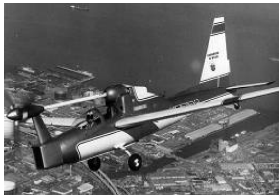
Figure 47. Q-Star with Novel Engine Propeller Design to Reduce the Noise (From [71])
