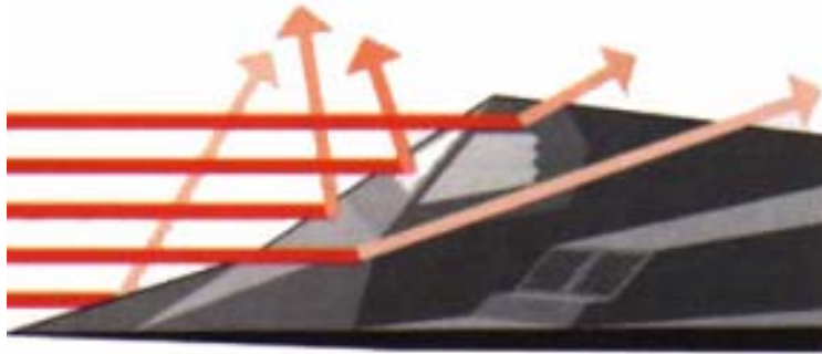
Figure 34. F-117 Nighthawk's RCS by Scattering the Incoming Signals Nearly Every Direction (From [49])
