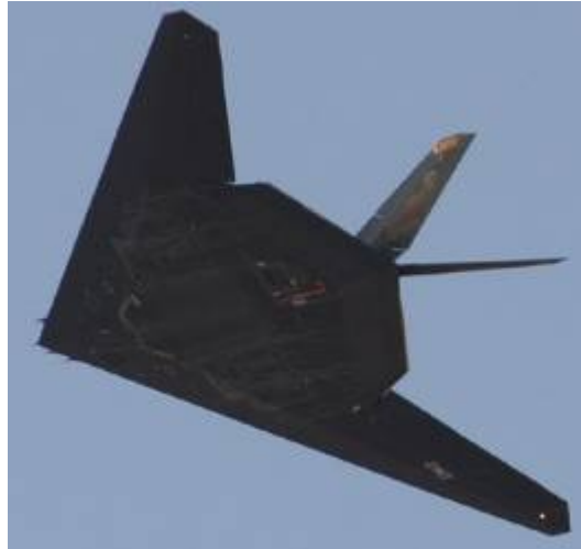
Figure 49. The Body of the F-117 is Designed to Mask IR Emission from Engines (From [75])
