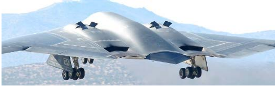
Figure 60. Auxiliary Air Intake Doors are Required for B-2's Take Off (From [82])
