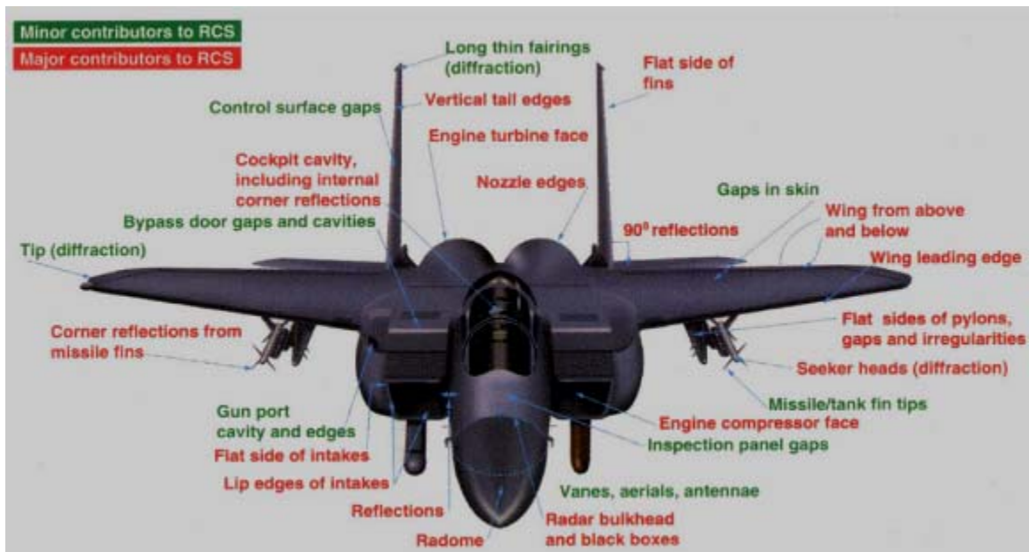
Figure 29. The Minor and Major Contributors to RCS of a Fighter Aircraft (From [49])
