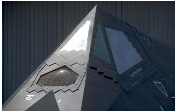
Figure 57. F-117's Fine Wire Mesh of FLIR Aperture, and Faceted-serrated Shape of its Canopy (From [81])
