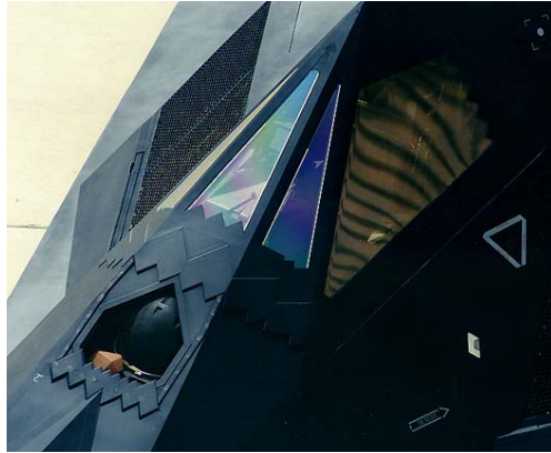
Figure 55. Reflection of F-117's Cockpit Coating (From [80])
