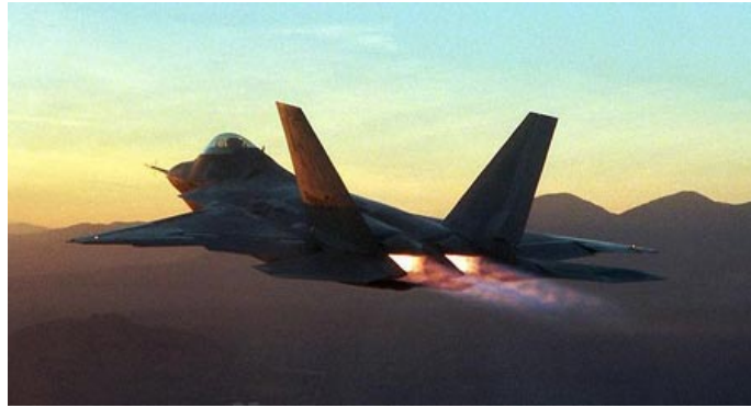
Figure 51. F-22 Raptor's Saw Toothed, Wide and Flat Shaped Nozzles to Reduce Both Radar and IR Signatures (From [77])
