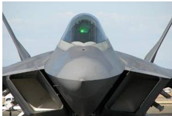
Figure 64. F-22's Radar is Fitted Inside the Nose Radome (From [89])
