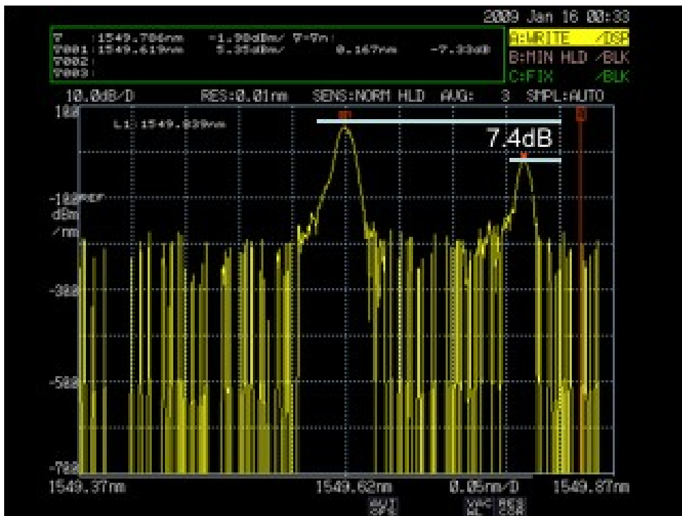
Figure 6.7: The same tone and carrier, with the FBG in place to filter all but the upper sideband. Note that the carrier-sideband ratio has changed by only 5 dB, although the lower sideband is not measurable.
