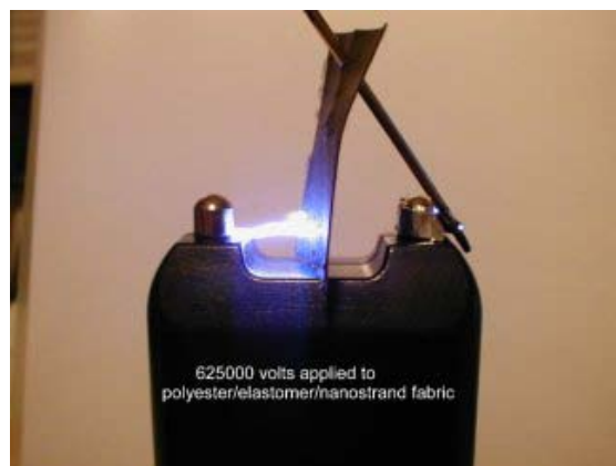
Figure 8. Controlled Electrostatic Discharge with 5% volume Ni Nanostrands™
