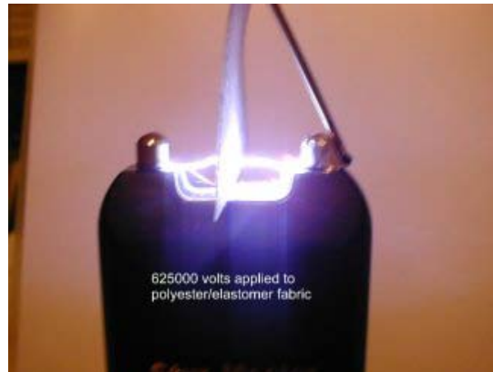
Figure 7. 625,000 Volt Discharge without Ni Nanostrands™
