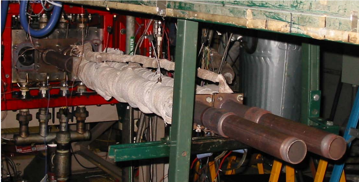
Figure 21. Photograph of the PDE with heat exchanger thrust tubes installed in positions 2 and 3
