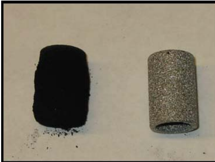
Figure 36. Photograph of carbon build up on a filter after one run next to a new filter
