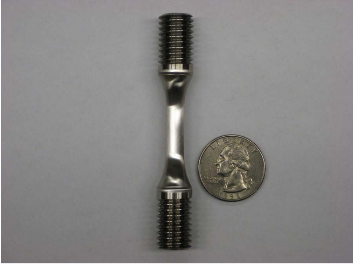
Figure 14: PWA1484 Test Specimen
