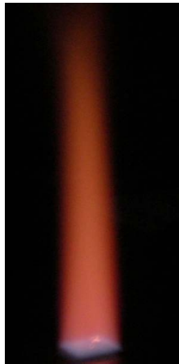
Figure 6: Laminar Hydrogen-air flame from Hencken burner
