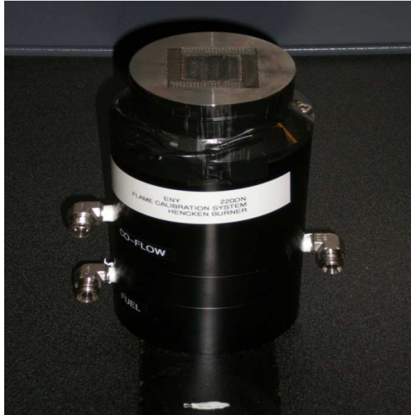
Figure 25: Hencken burner utilized for calibration of the TDLAS system in the AFIT COAL Laboratory
