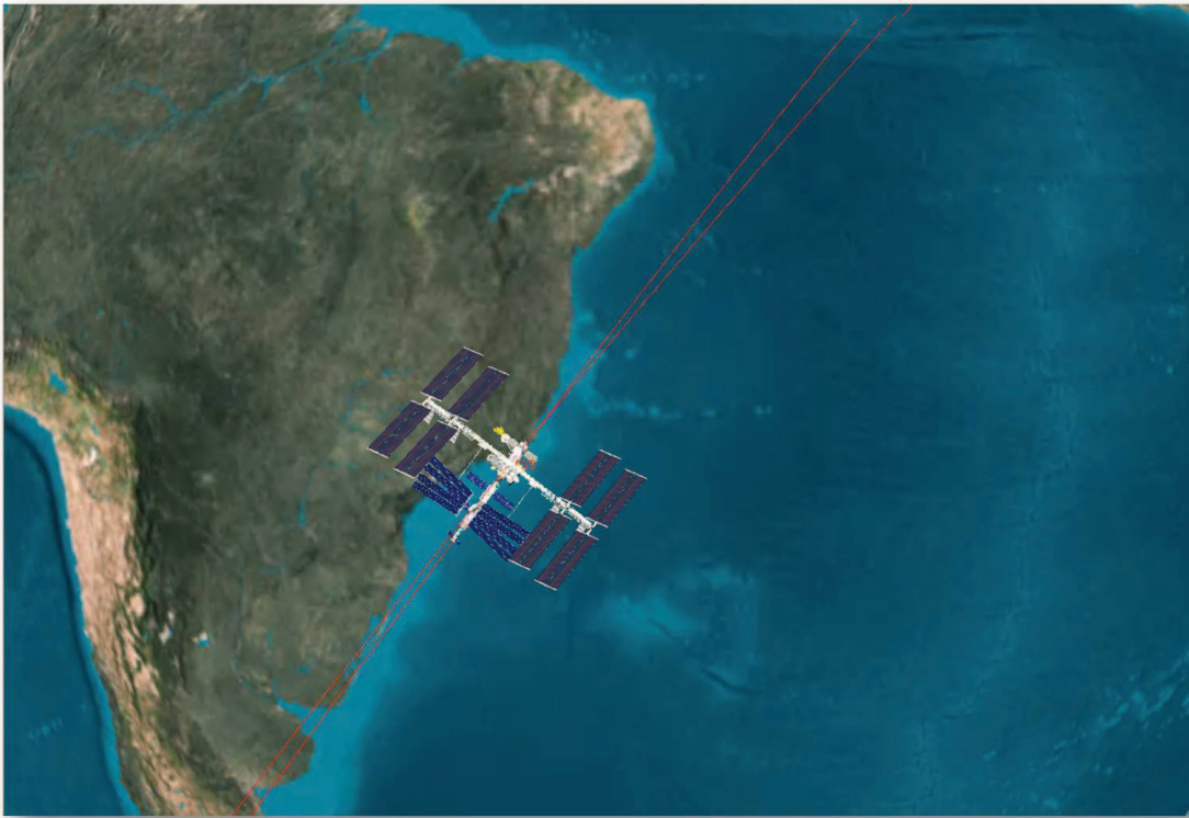
Figure 4.7: The ISS regularly passes through the South Atlantic Anomaly in its orbit. A higher chance of SEUs results. [12]
