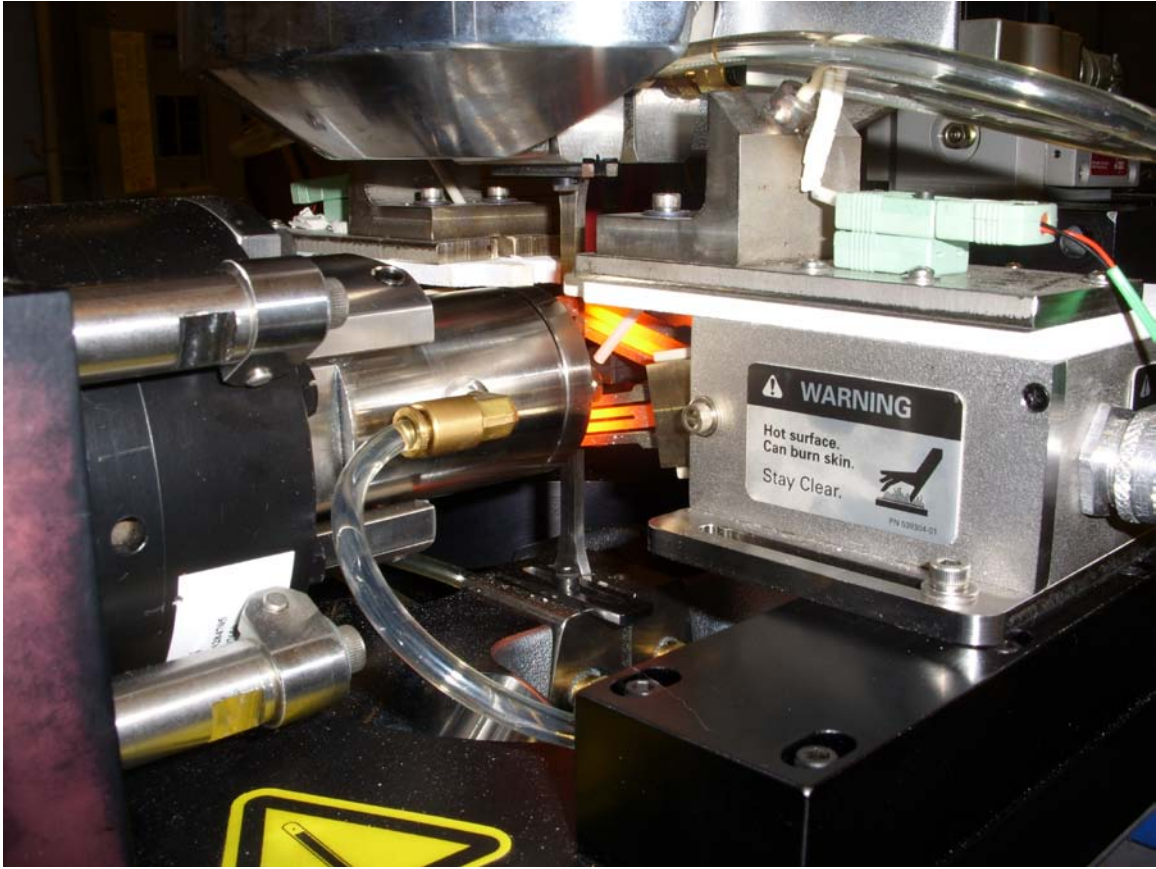
Figure 3.5 – Heating element/thermocouple apparatus
