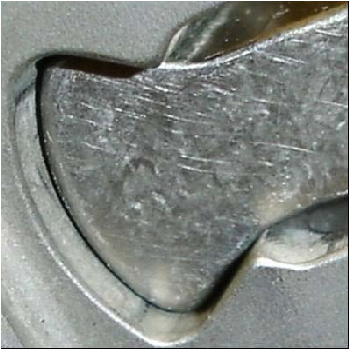
Figure 1.2 – Photograph of a turbine dovetail joint [13]
