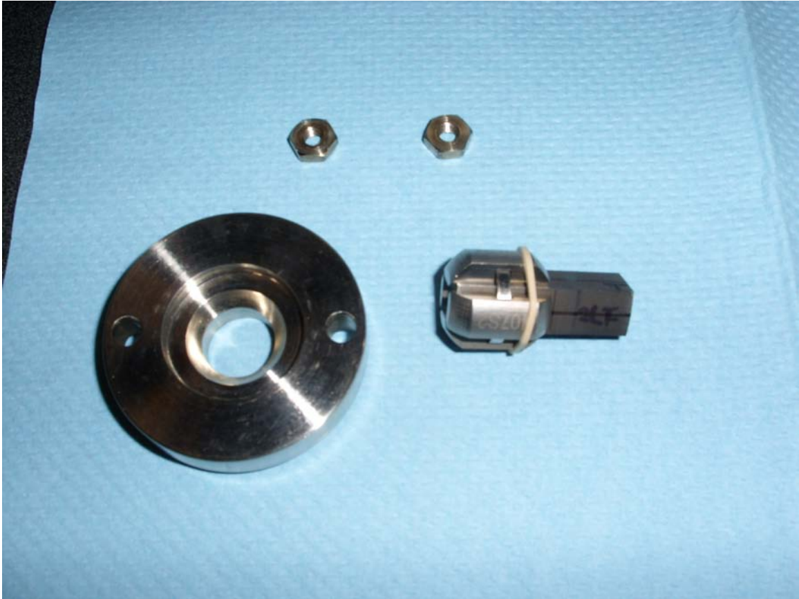
Figure 3.6 – Fretting pad collar assembly
