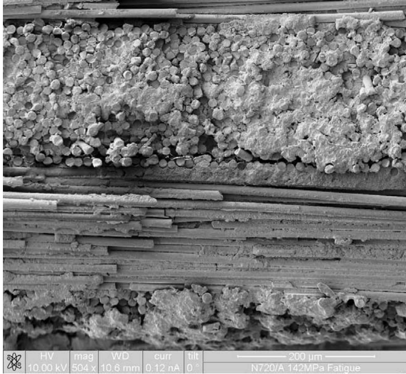
Figure 80. 142 MPa Side Fracture Back Fiber-Matrix, 504x
