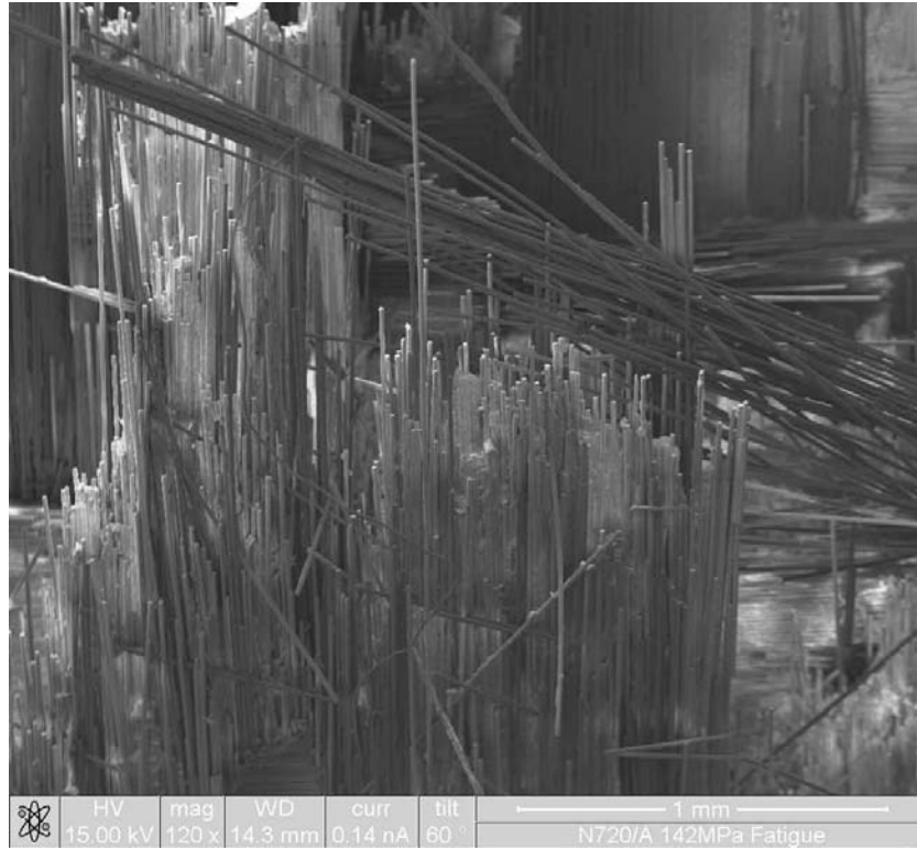
Figure 98. 142 MPa Fracture Surface, Rear Left Fiber Pullout, 120x
