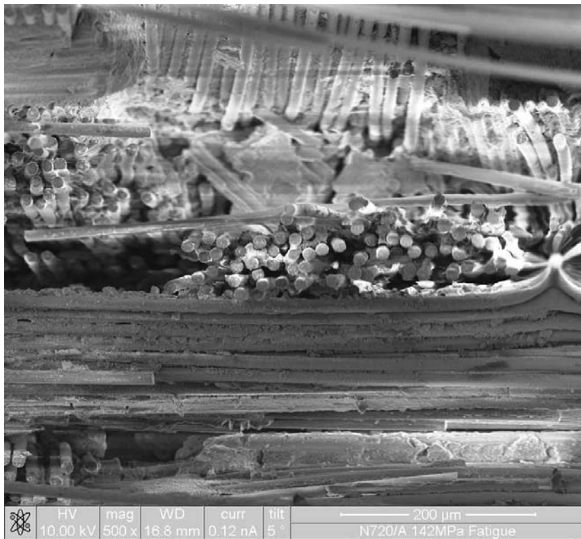
Figure 93. 142 MPa Fracture Surface, Rear Left Fiber Pullout, 500x
