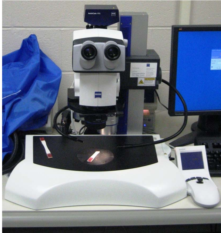
Figure 20. Zeiss Discovery V12 Optical Microscope
