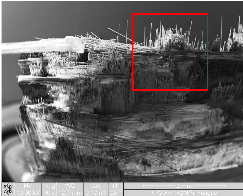
Figure 62. Front Left Edge Fracture Surface (Flame Side at Top)
