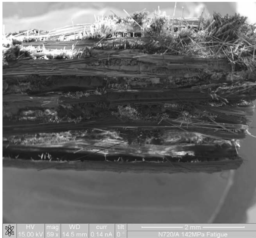
Figure 83. 142 MPa Fracture Surface, Overhead Right View, 59x
