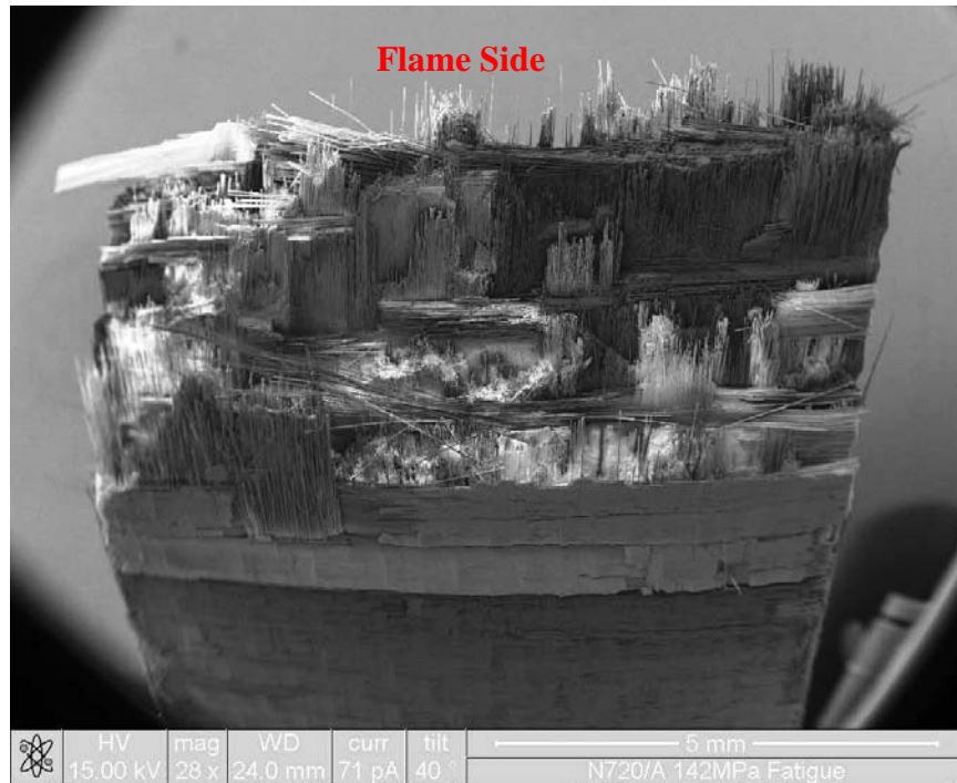
Figure 54. 142 MPa Fracture Surface (Rear Looking Towards Flame Side)
