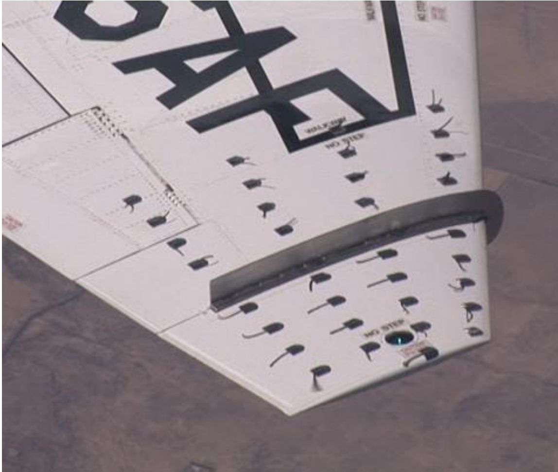
Figure 176. Fence Tufted Wing at 8.6^\circ AOA (0.58 normalized) and 179 KCAS
