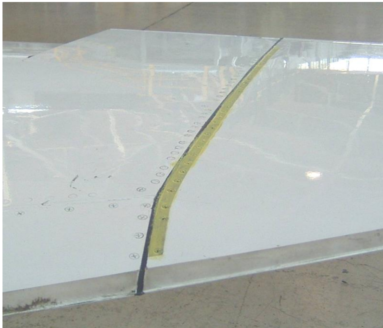
Figure 27. Jink in Wing Tip Seam
