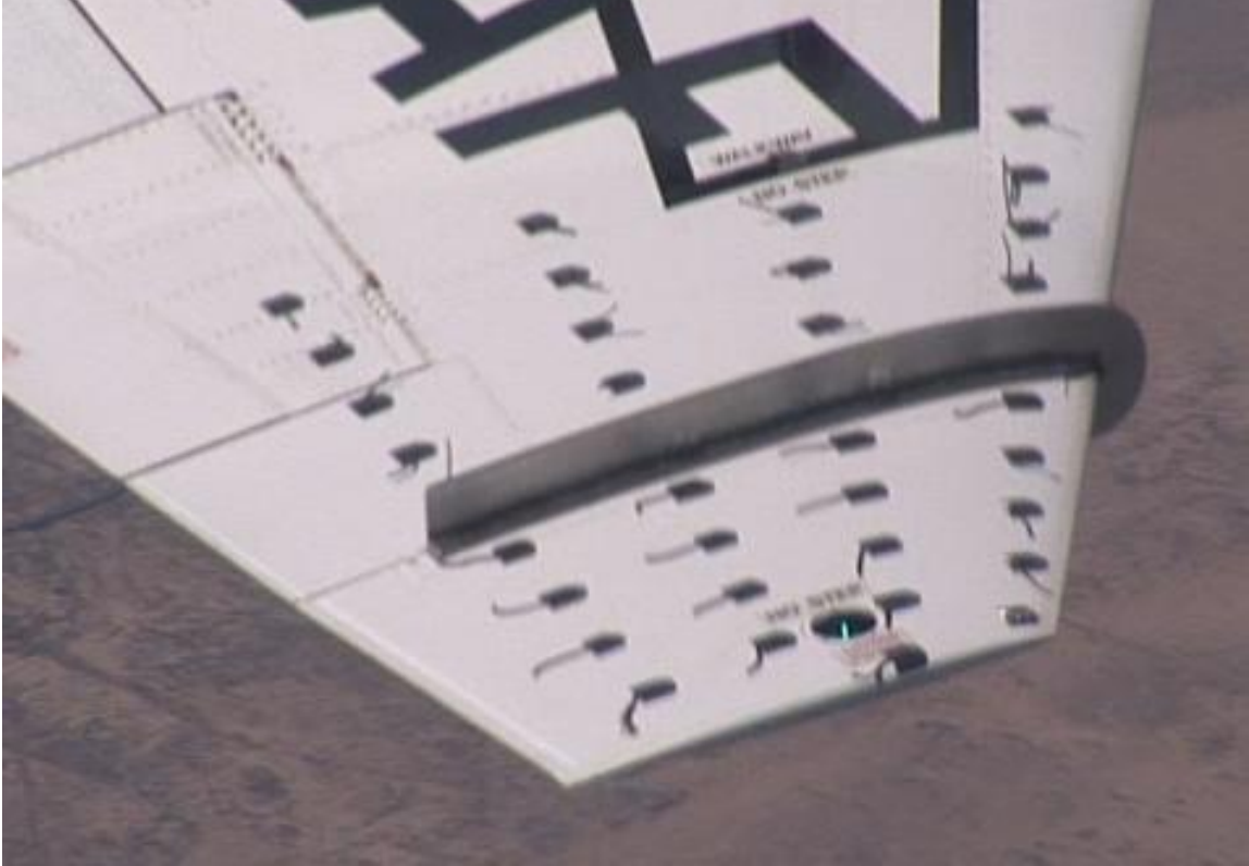
Figure 182. Fence Tufted Wing at 9.6° AOA (0.65 normalized) and 174 KIAS
