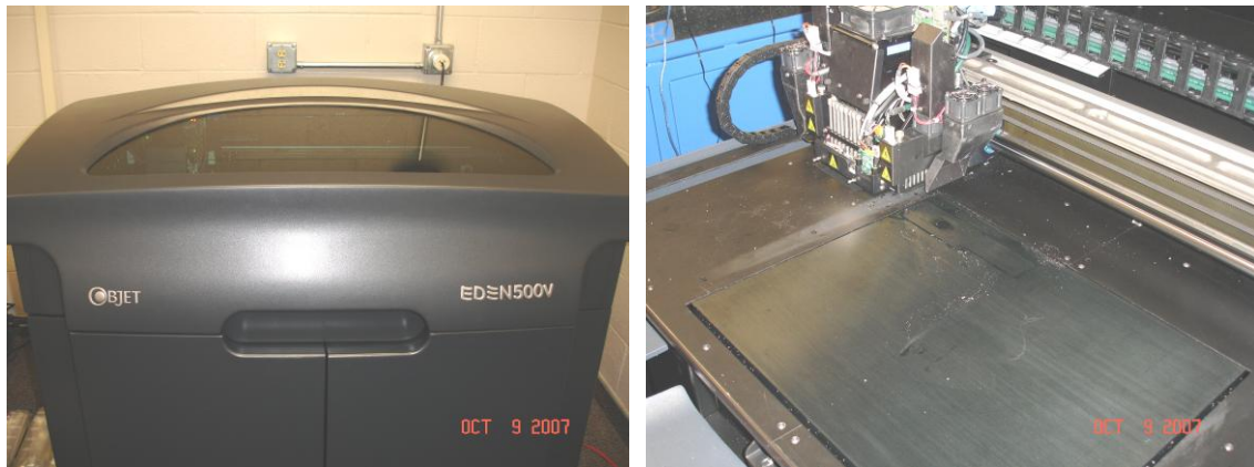
Figure 31. The Objet Eden™ 500V Printer, Printer Head, and Tray
