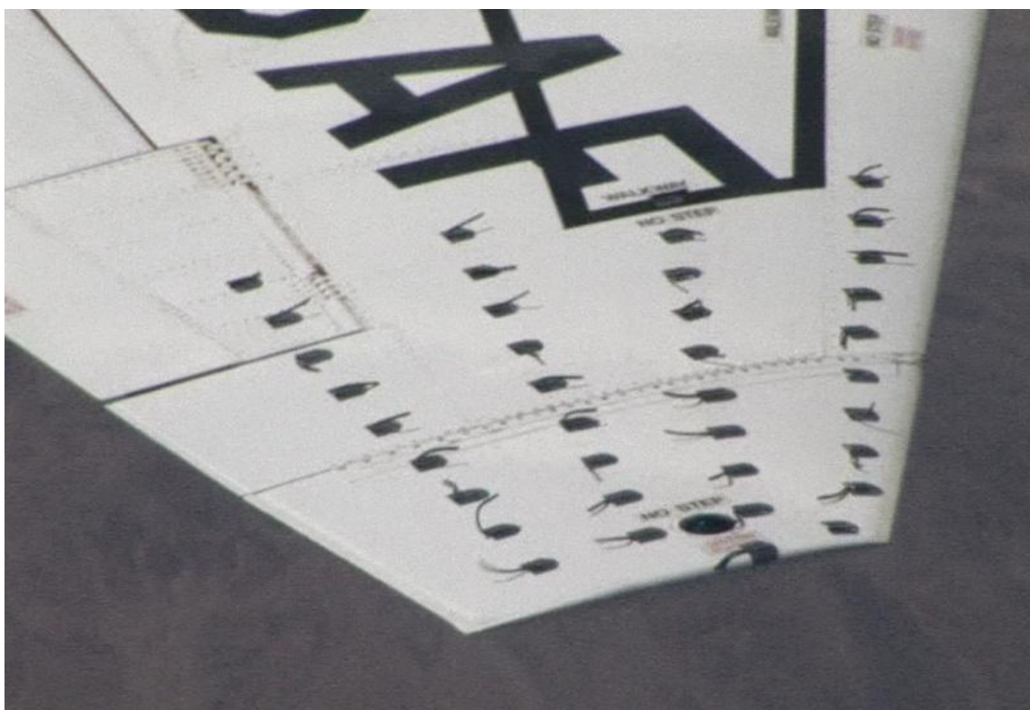
Figure 203. Clean Tufted Wing at 14.2^\circ AOA (0.94 normalized) and 152 KCAS
