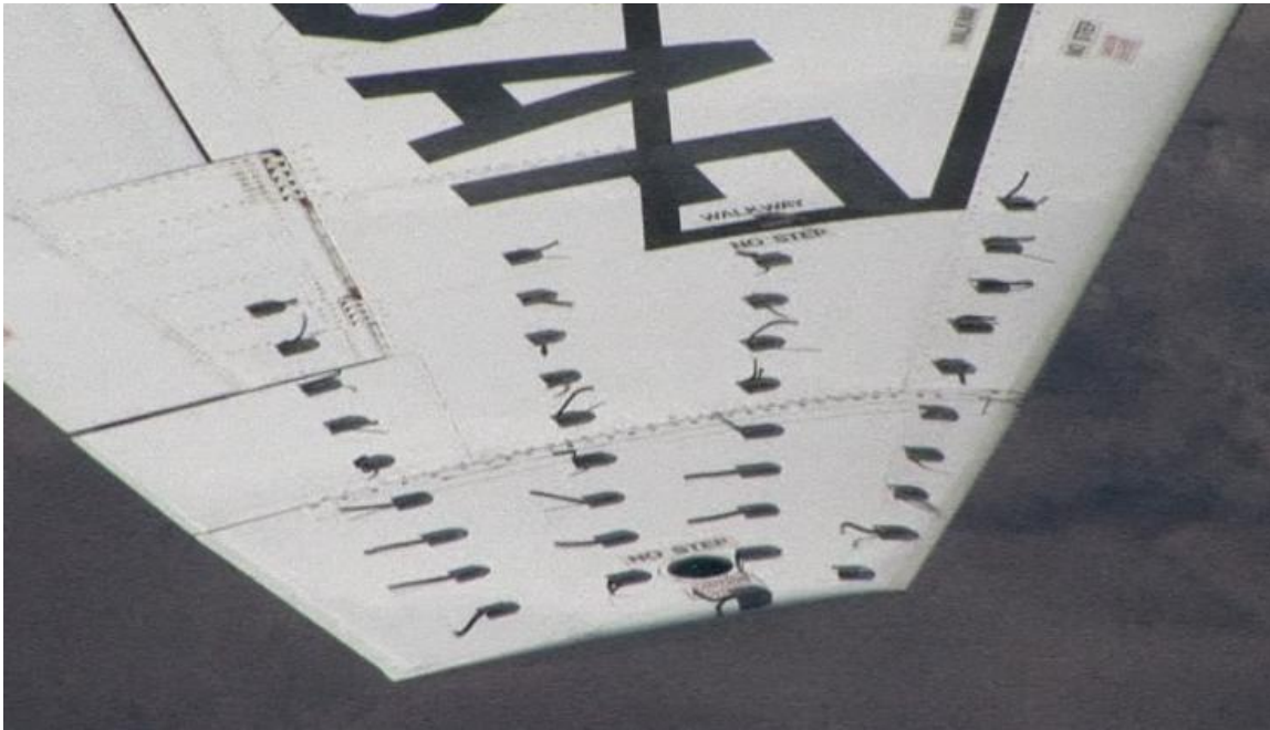
Figure 190. Fence Tufted Wing at 11.4^\circ AOA (0.77 normalized) and 159 KCAS
