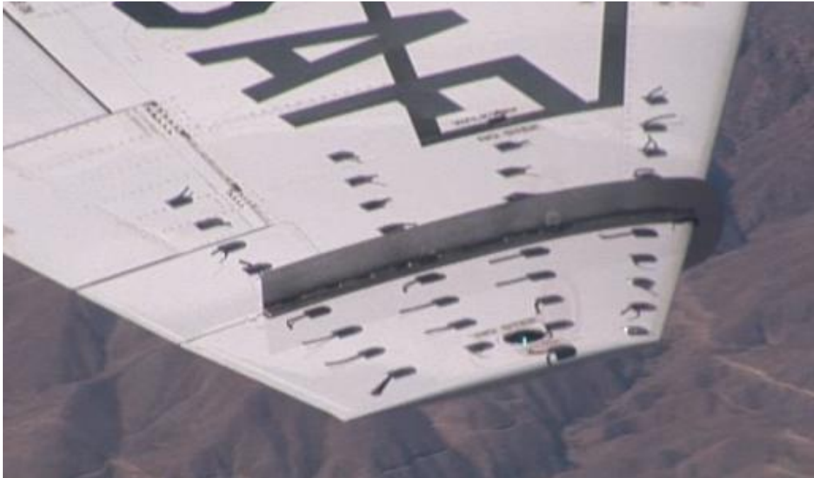
Figure 204. Fence Tufted Wings at 14.9^\circ (1.0 normalized) AOA and 153 KCAS
