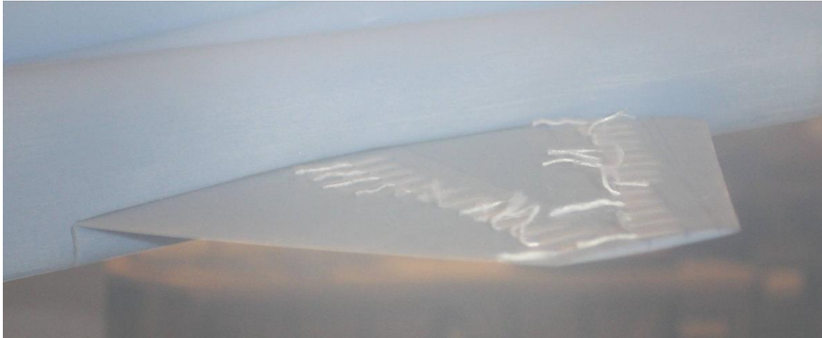
Figure 115. Clean Tufts 10 Degrees – Right Wing Side View (90 mph)
