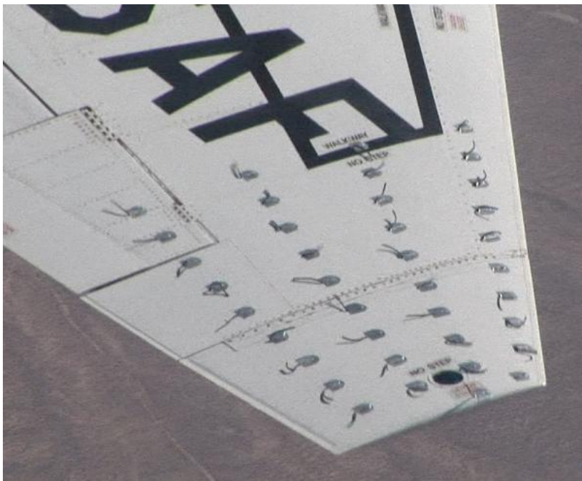
Figure 193. Clean Tufted Wing at 11.9^\circ AOA (0.80 normalized) and 164 KIAS
