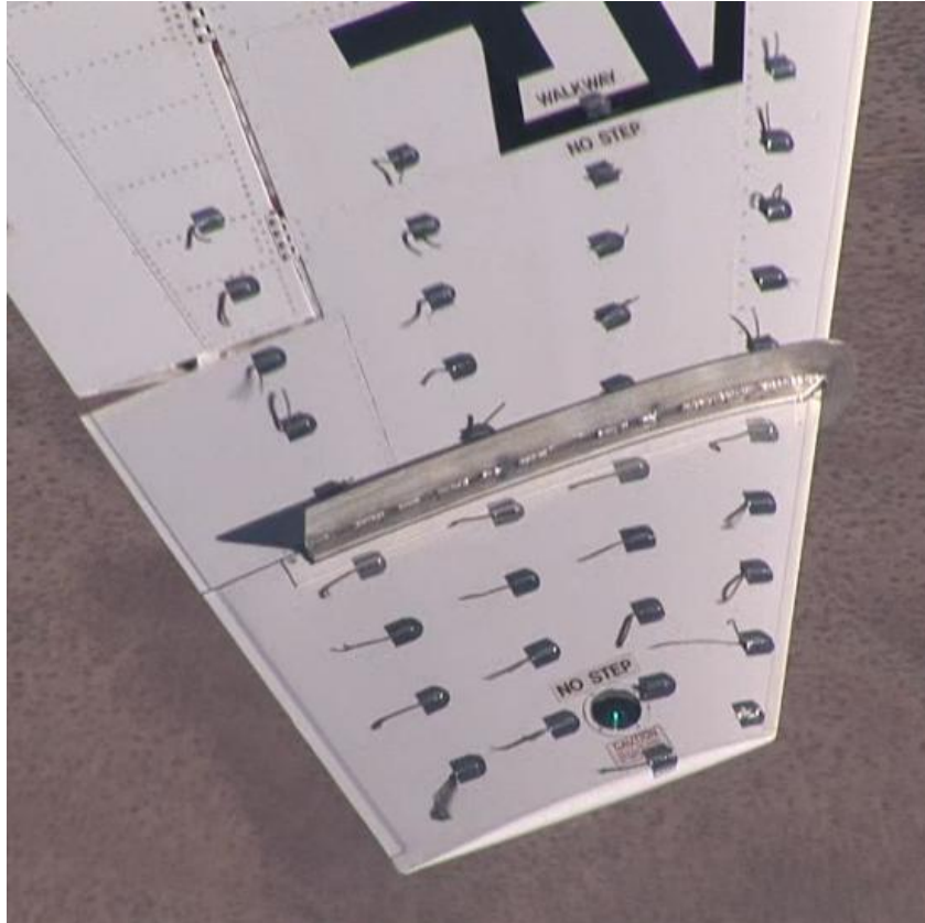
Figure 186. Fence Tufted Wing at 10.7^\circ AOA (0.72 normalized) and 169 KCAS
