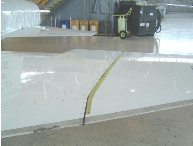
Figure 4. T-38 Wing Seam Located 26.5 Inches from Wingtip
