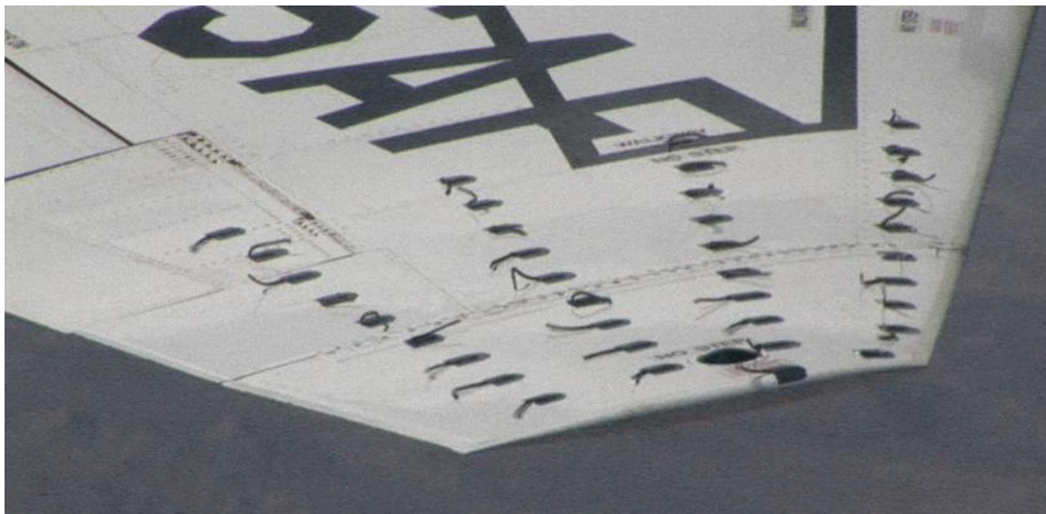
Figure 175. Clean Tufted Wing at 8.4^\circ AOA (0.56 normalized) and 188 KCAS
