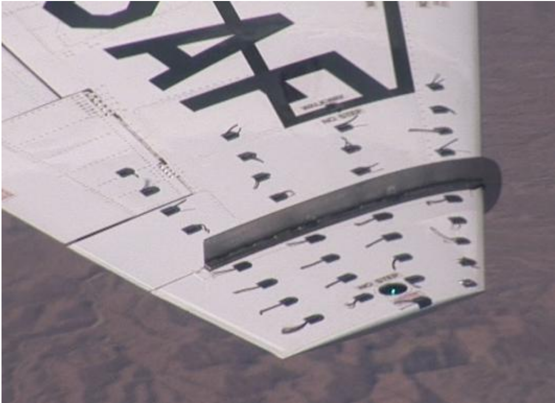
Figure 188. Fence Tufted Wings at 10.7^\circ AOA (0.72 normalized) and 164 KCAS
