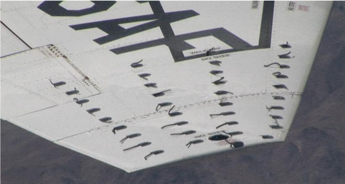
Figure 183. Clean Tufted Wing at 9.6° AOA (0.65 normalized) and 175 KCAS
