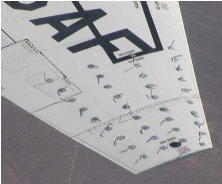
Figure 187. Clean Tufted Wing at 10.7^\circ AOA (0.72 normalized) and 169 KCAS
