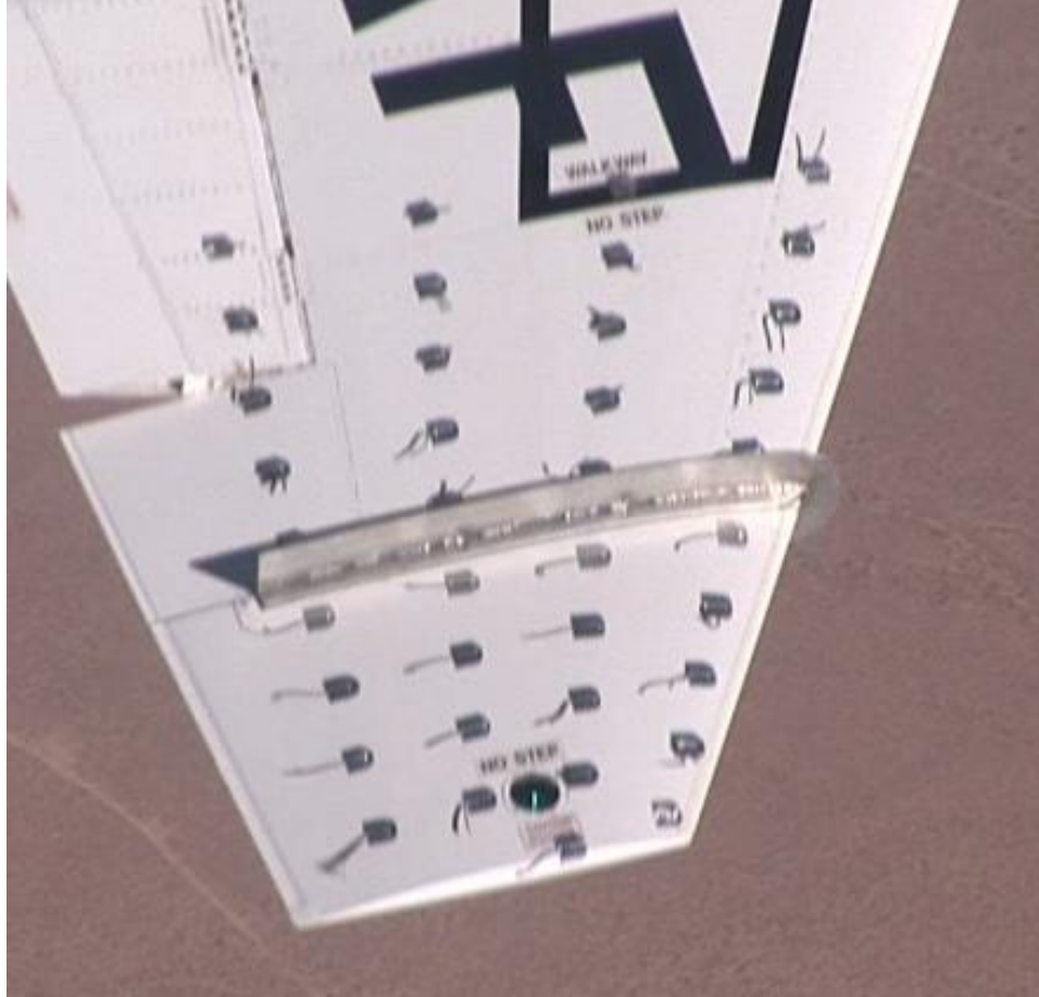
Figure 198. Fence Tufted Wings at 13.4^\circ AOA (0.90 normalized) and 154 KCAS
