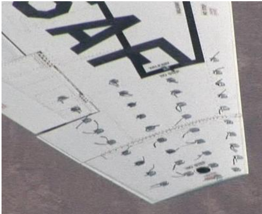
Figure 201. Clean Tufted Wing at 13.9^\circ AOA (0.92 normalized) and 153 KCAS
