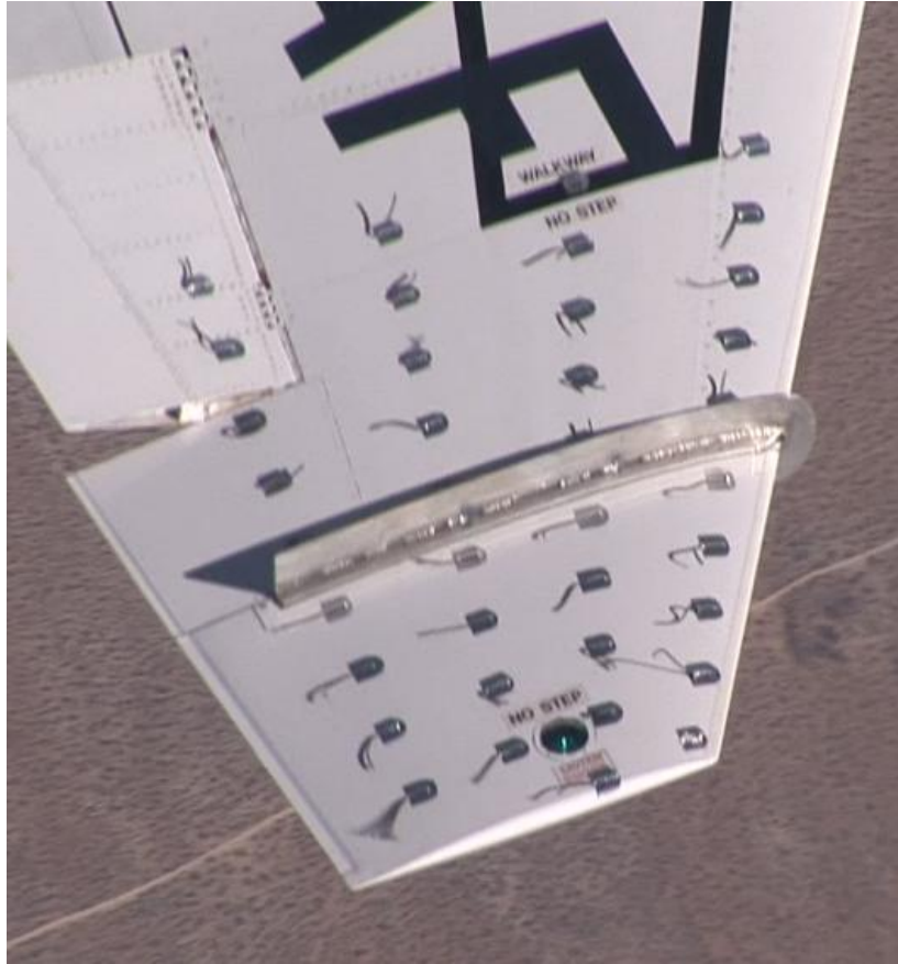
Figure 194. Fence Tufted Wings at 12.4^\circ AOA (0.83 normalized) and 159 KCAS
