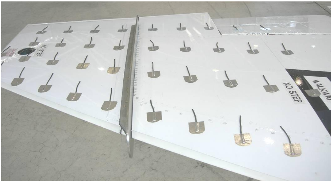
Figure 65. Flight Test Installed Tufts (Front View)
