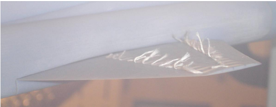
Figure 120. Clean Tufts 15 Degrees – Right Wing Side View (90 mph)
