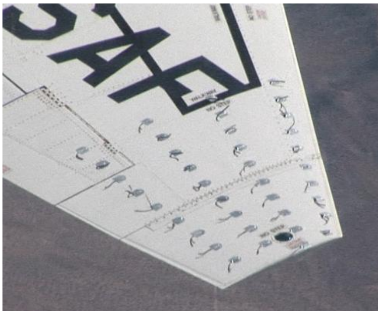
Figure 173. Clean Tufted Wing at 8.1^\circ AOA (0.53 normalized) and 192 KCAS
