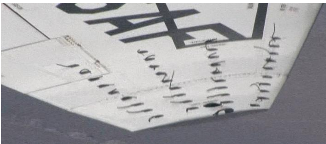
Figure 185. Clean Tufted Wing at 10.3^\circ AOA (0.69 normalized) and 170 KCAS
