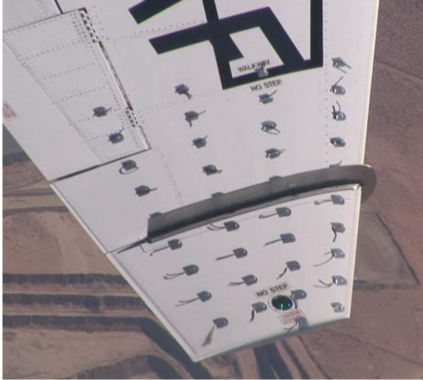
Figure 200. Fence Tufted Wings at 13.9^\circ AOA (0.92 normalized) and 149 KIAS
