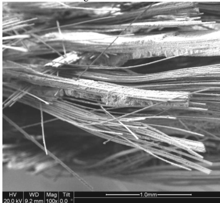
Figure 63. SEM micrograph of the fracture surface of the N720/AM specimen subjected to tensile test to failure following 100 h at 13 MPa at 1200°C in laboratory air.
