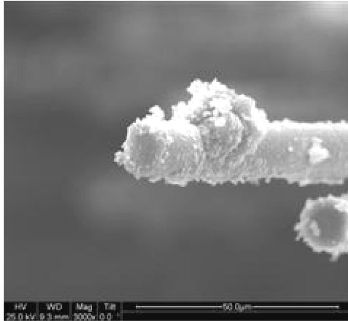
Figure 344. SEM micrograph of the fracture surface of the N720/AM specimen subjected to tensile test to failure following 100 h at 20 MPa at 1200°C in argon.
