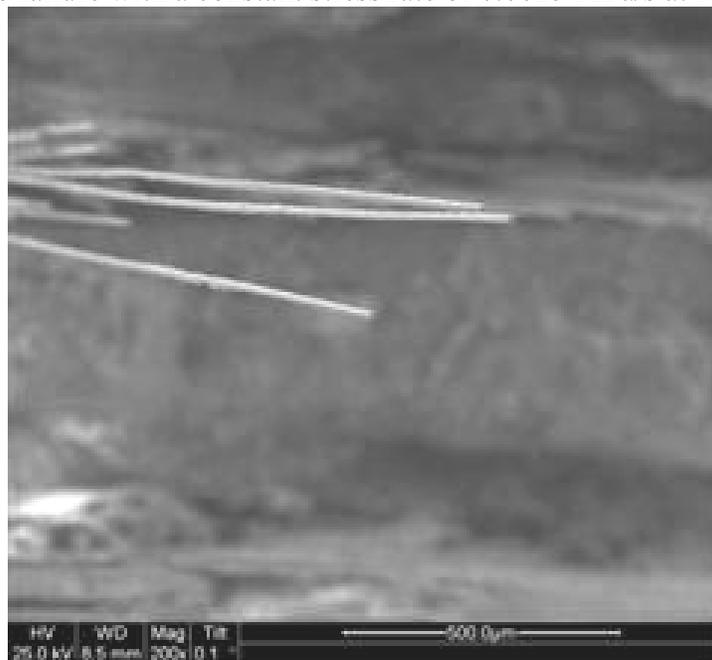
Figure 553. SEM micrograph of the fracture surface of the N720/AM specimen subjected to tensile test to failure with a constant stress rate of 0.0025 MPa/s at 1200°C in steam.
