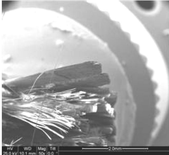
Figure 434. SEM micrograph of the fracture surface of the N720/AM specimen with  $\pm 45^\circ$  fiber orientation obtained in creep test conducted at 32 MPa at 1200°C in argon. Creep lifetime  $t_f = 0.08$  h.
