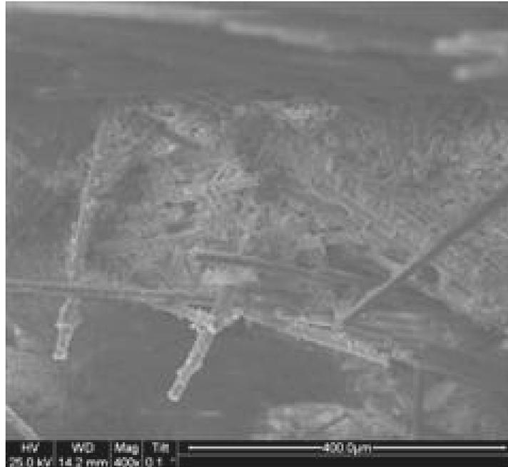
Figure 506. SEM micrograph of the fracture surface of the N720/AM specimen subjected to tensile test to failure with a constant stress rate of 0.0025 MPa/s at 1200°C in laboratory air.
