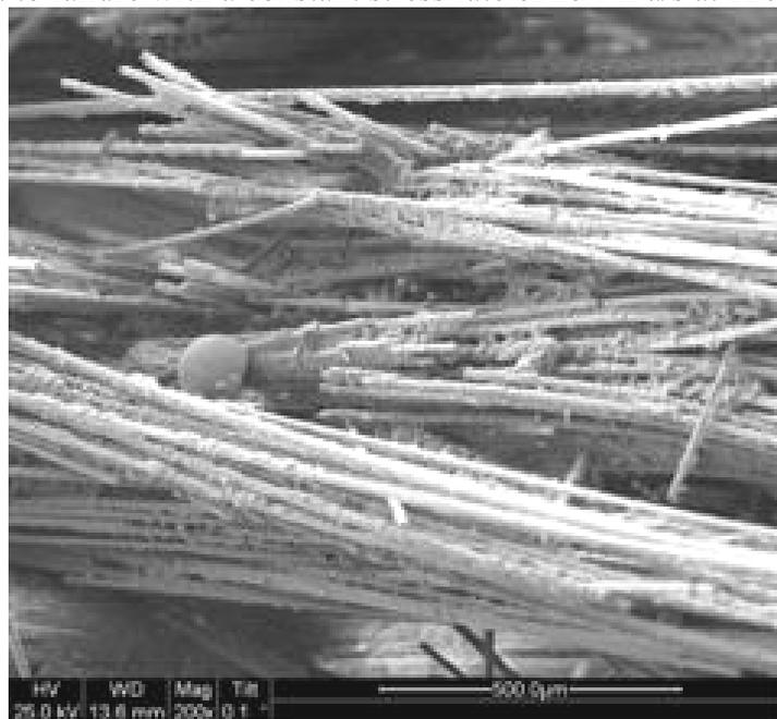
Figure 627. SEM micrograph of the fracture surface of the N720/AM specimen subjected to tensile test to failure with a constant stress rate of 25 MPa/s at 1200°C in steam.
