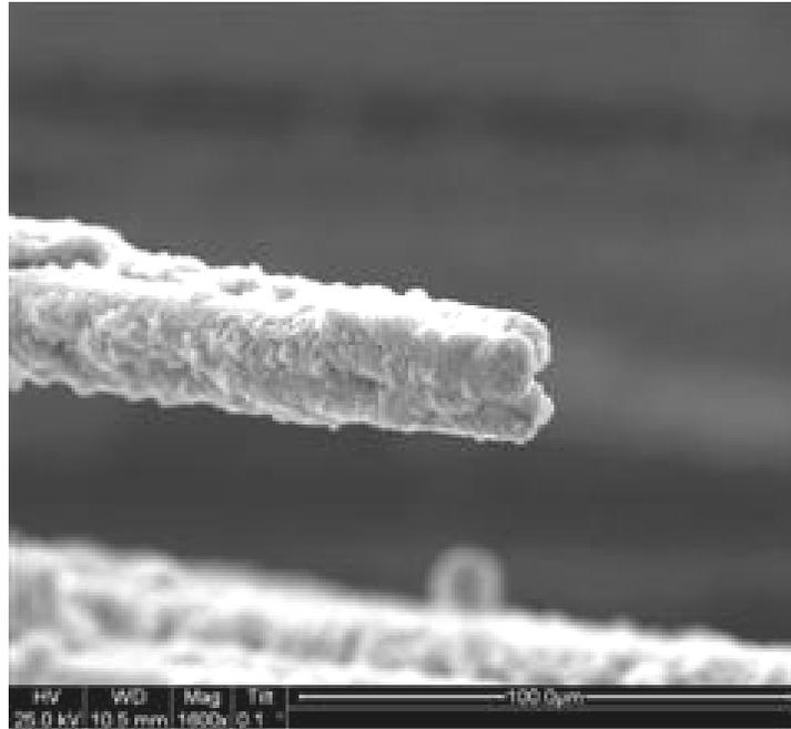
Figure 610. SEM micrograph of the fracture surface of the N720/AM specimen subjected to tensile test to failure with a constant stress rate of 25 MPa/s at 1200°C in steam.
