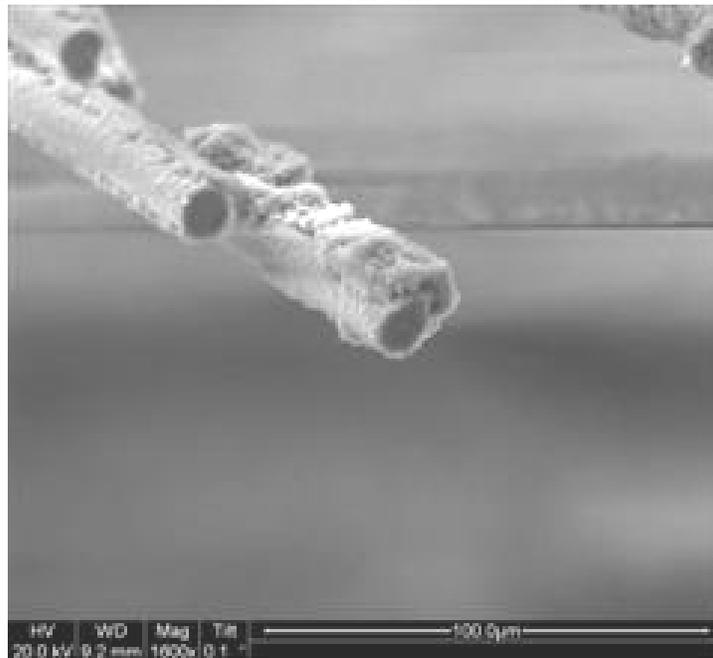
Figure 519. SEM micrograph of the fracture surface of the N720/AM specimen subjected to tensile test to failure with a constant stress rate of 0.0025 MPa/s at 1200°C in steam.
