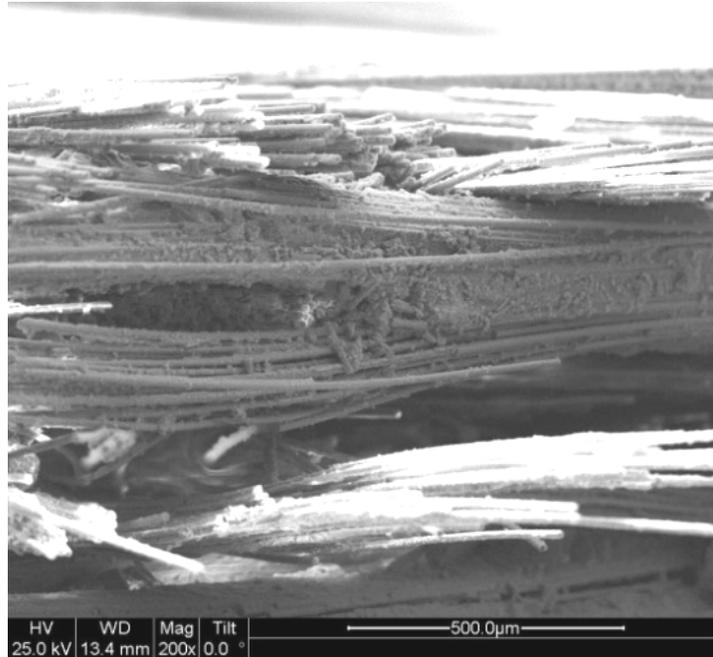
Figure 102. SEM micrograph of the fracture surface of the N720/AM specimen subjected to tensile test to failure following 100 h at 30 MPa at 1200°C in laboratory air.
