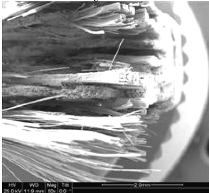
Figure 187. SEM micrograph of the fracture surface of the N720/AM specimen subjected to tensile test to failure following 100 h at 13 MPa at 1200°C in steam.
