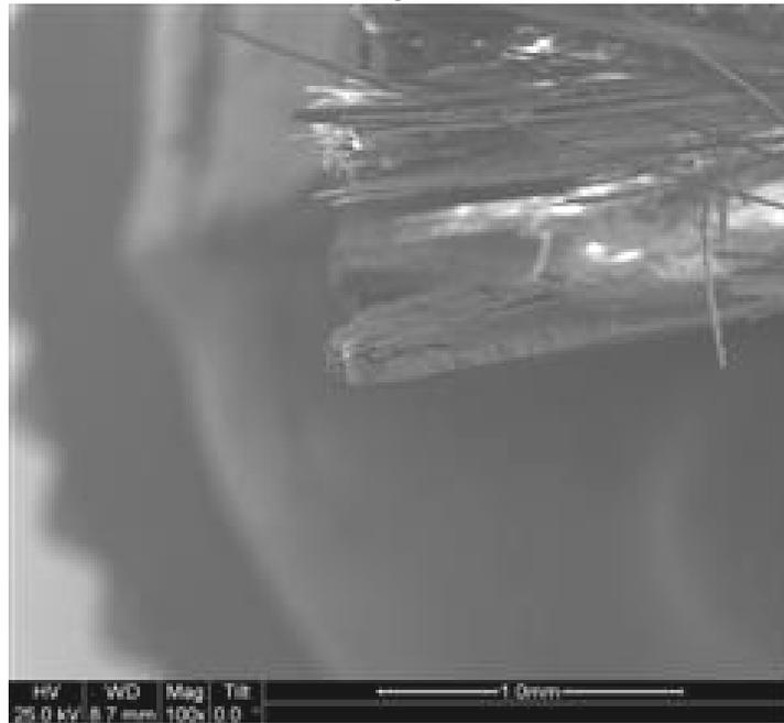
Figure 257. SEM micrograph of the fracture surface of the N720/AM specimen with  $\pm 45^\circ$  fiber orientation obtained in creep test conducted at 30 MPa at 1200°C in steam. Creep lifetime  $t_f = 1.08$  h.
