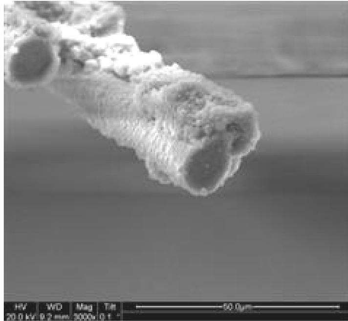
Figure 520. SEM micrograph of the fracture surface of the N720/AM specimen subjected to tensile test to failure with a constant stress rate of 0.0025 MPa/s at 1200°C in steam.
