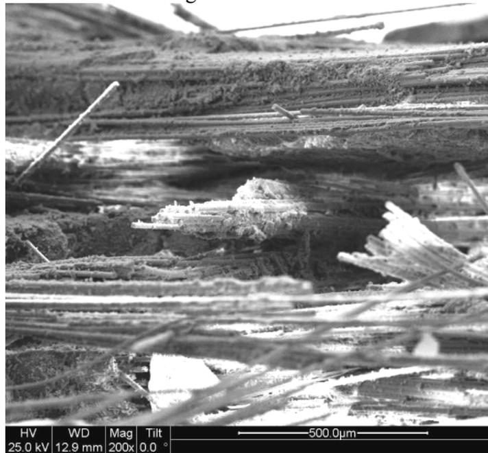
Figure 71. SEM micrograph of the fracture surface of the N720/AM specimen subjected to tensile test to failure following 100 h at 13 MPa at 1200°C in laboratory air.
