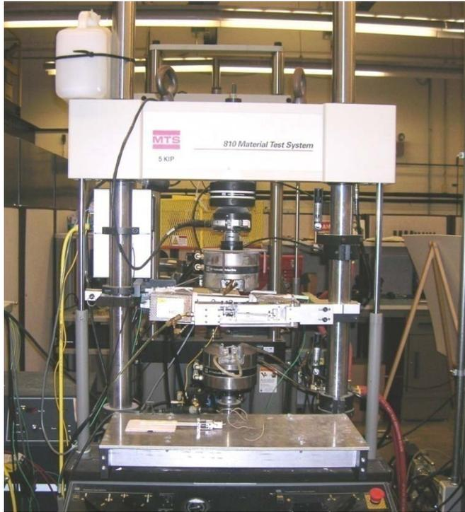
**Figure 4. MTS 5 kip mechanical testing machine**
