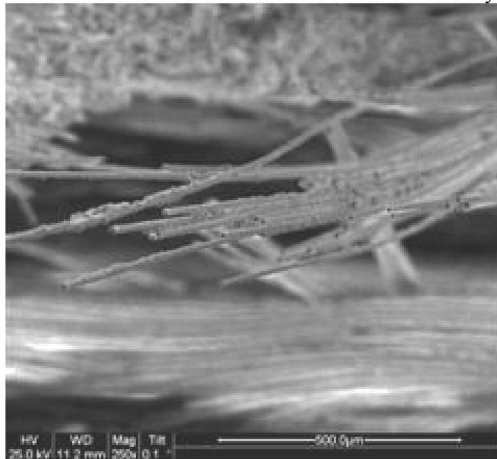
Figure 649. SEM micrograph of the fracture surface of the N720/AM specimen subjected to monotonic tensile test to failure at 1200°C in laboratory air.
