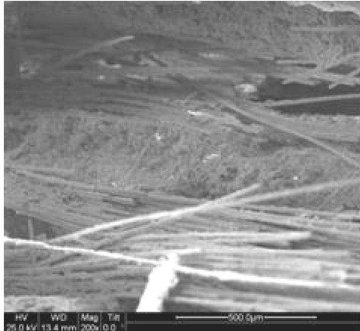
Figure 336. SEM micrograph of the fracture surface of the N720/AM specimen subjected to tensile test to failure following 100 h at 20 MPa at 1200°C in argon.
