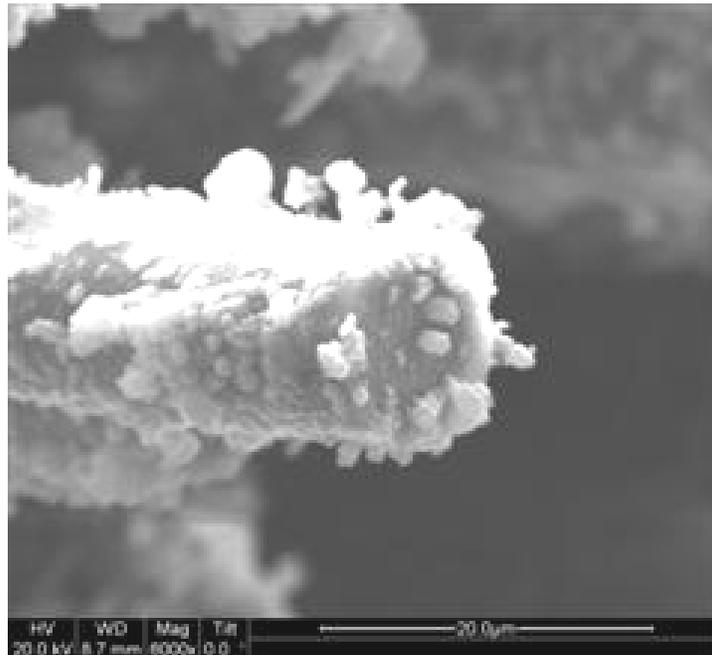
Figure 573. SEM micrograph of the fracture surface of the N720/AM specimen subjected to tensile test to failure with a constant stress rate of 25 MPa/s at 1200°C in laboratory air.
