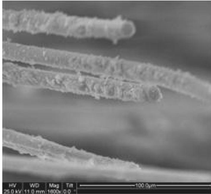
Figure 236. SEM micrograph of the fracture surface of the N720/AM specimen with  $\pm 45^\circ$  fiber orientation obtained in creep test conducted at 30 MPa at 1200°C in steam. Creep lifetime  $t_f = 1.08$  h.
