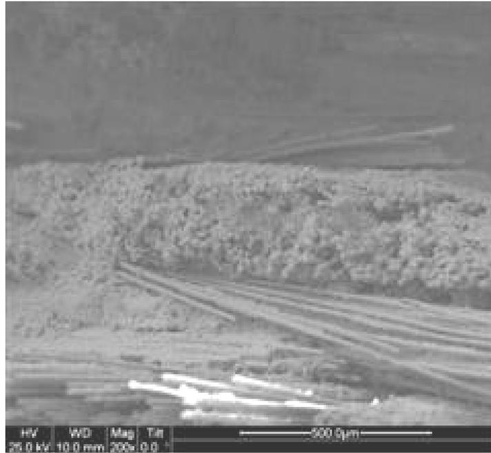
Figure 330. SEM micrograph of the fracture surface of the N720/AM specimen subjected to tensile test to failure following 100 h at 20 MPa at 1200°C in argon.
