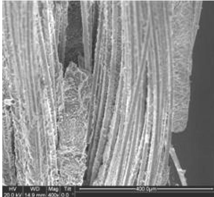
Figure 660. SEM micrograph of the fracture surface of the N720/AM specimen subjected to monotonic tensile test to failure at 1200°C in laboratory air.
