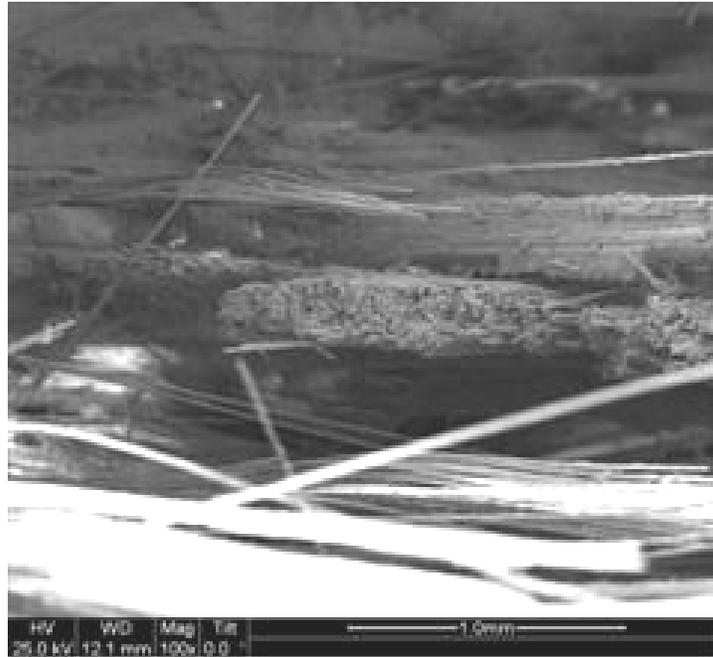
Figure 202. SEM micrograph of the fracture surface of the N720/AM specimen subjected to tensile test to failure following 100 h at 13 MPa at 1200°C in steam.
