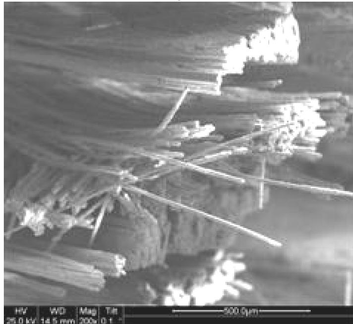
Figure 281. SEM micrograph of the fracture surface of the N720/AM specimen with  $\pm 45^\circ$  fiber orientation obtained in creep test conducted at 32 MPa at 1200°C in steam. Creep lifetime  $t_f = 0.02$  h.
