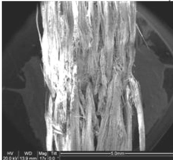
Figure 659. SEM micrograph of the fracture surface of the N720/AM specimen subjected to monotonic tensile test to failure at 1200°C in laboratory air.
