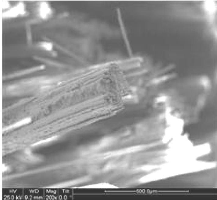
Figure 430. SEM micrograph of the fracture surface of the N720/AM specimen with  $\pm 45^\circ$  fiber orientation obtained in creep test conducted at 32 MPa at 1200°C in argon. Creep lifetime  $t_f = 0.08$  h.
