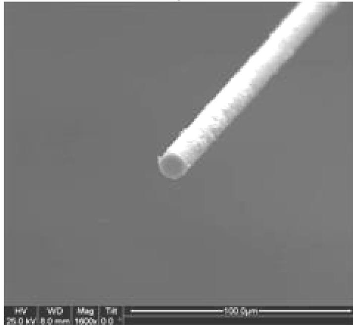
Figure 449. SEM micrograph of the fracture surface of the N720/AM specimen with  $\pm 45^\circ$  fiber orientation obtained in creep test conducted at 32 MPa at 1200°C in argon. Creep lifetime  $t_f = 0.08$  h.
