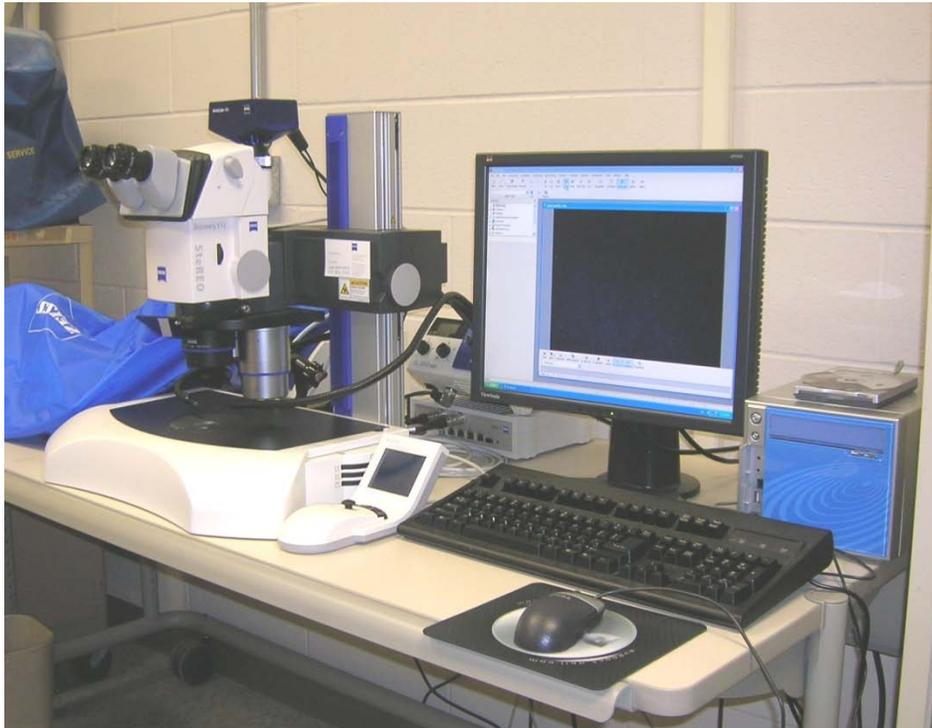
**Figure 9. Zeiss Stemi SV II optical microscope**
