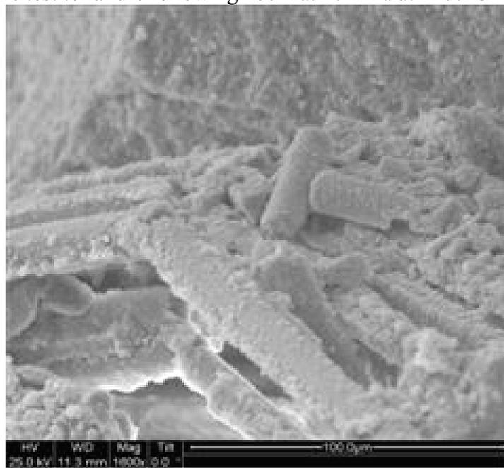
Figure 355. SEM micrograph of the fracture surface of the N720/AM specimen subjected to tensile test to failure following 100 h at 20 MPa at 1200°C in argon.
