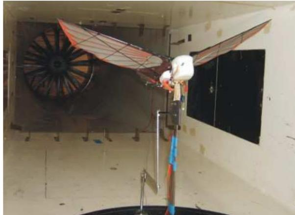
Fig. 3 The ornithopter in the wind tunnel.
