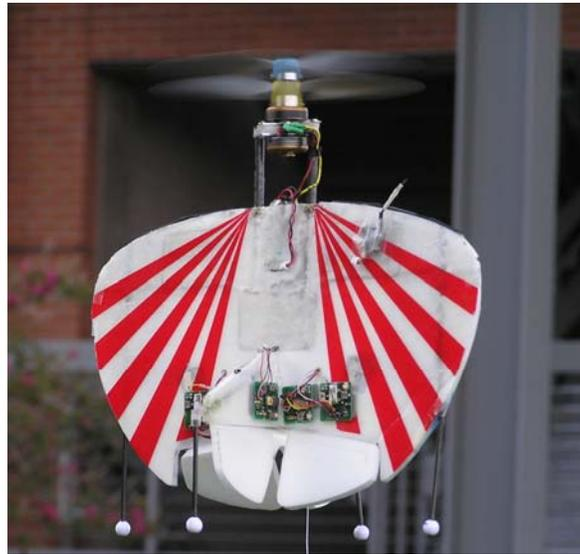
Fig. 16 VTOL MAV in flight.
