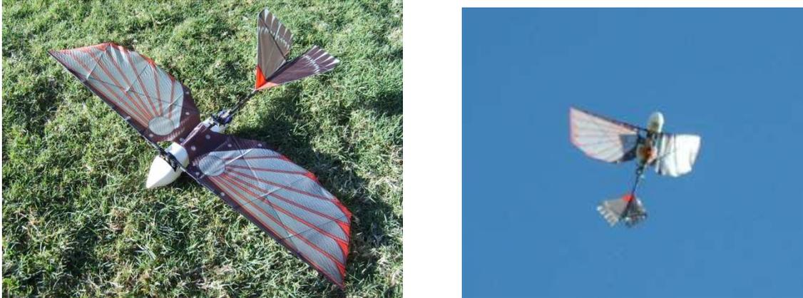
**Fig. 1 Autonomous ornithopter on the ground (left) and in flight (right).**
