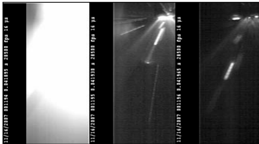
Figure 11: Particle Travel Progress at 28500 fps and 16 \mu sec of Exposure Time
