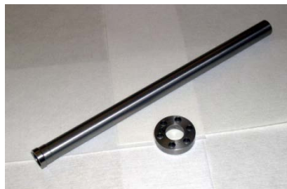
Figure 14. Molybdenum cathode tube (long) and mounting flange.
