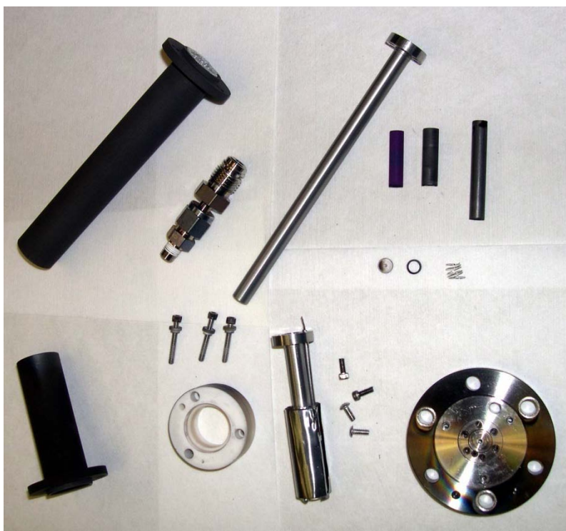
Figure 18. Parts breakdown for cathodes—keeper and cathode tubes for both long and short cathodes shown. (Short cathode tube shown with heater wire and tantalum foil.)
