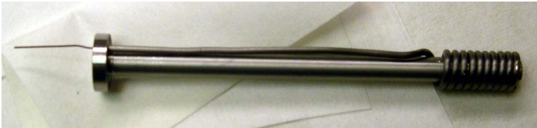
Figure 15. Assembled (long) cathode tube with heater wire installed.
