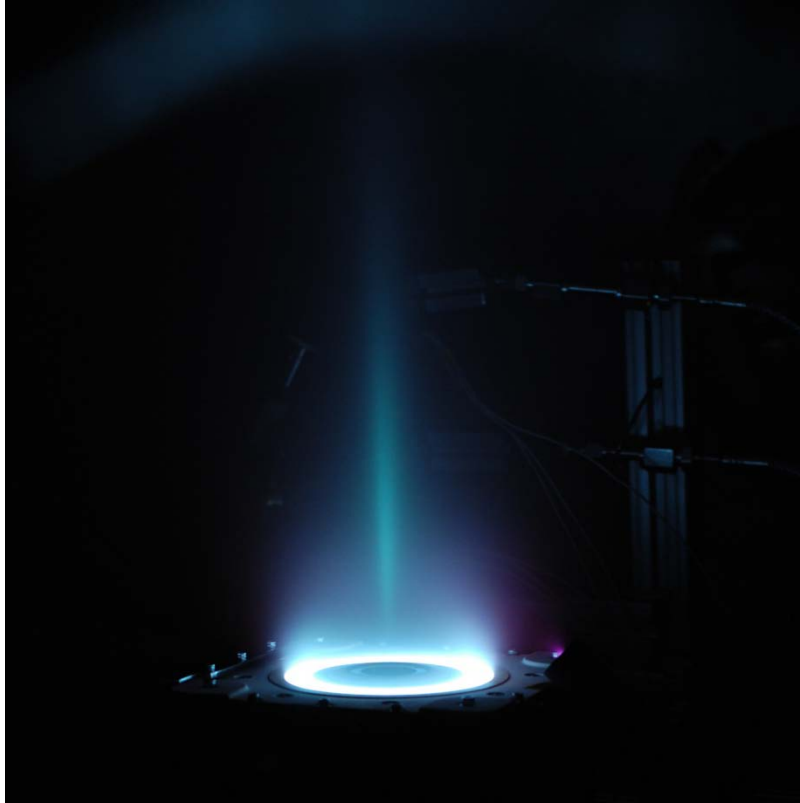
Figure 32. BHT-1500-C operating with externally-mounted cathode.
