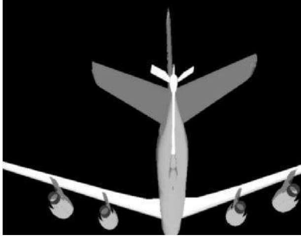
Figure 2.7: Sample 3D Rendering of Tanker Aircraft. Matlab ® Virtual Reality environment renders a predicted image of the lead tanker from the perspective of the receiver aircraft.
