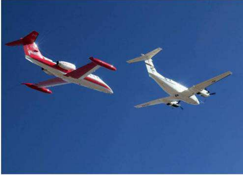
Figure 2.10: Image of Calspan Learjet and C-12 surrogate tanker aircraft during Ross/Spinelli Formation Flight Test
