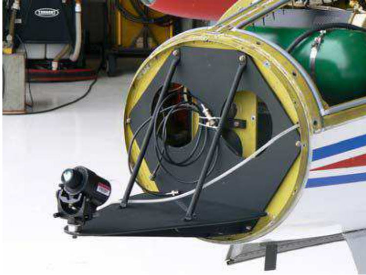
Figure 2.8: Orientation of the LWIR Camera when mounted in the nose of the receiver aircraft during data collection flights. The camera has a pitch angle of +28^{\circ} .
