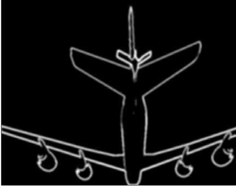
Figure 2.6: Example image after applying magnitude of gradient with threshold. The threshold on the gradient amplifies the edges of the tanker while removing any unwanted gradient due to background clutter or lens reflection.
