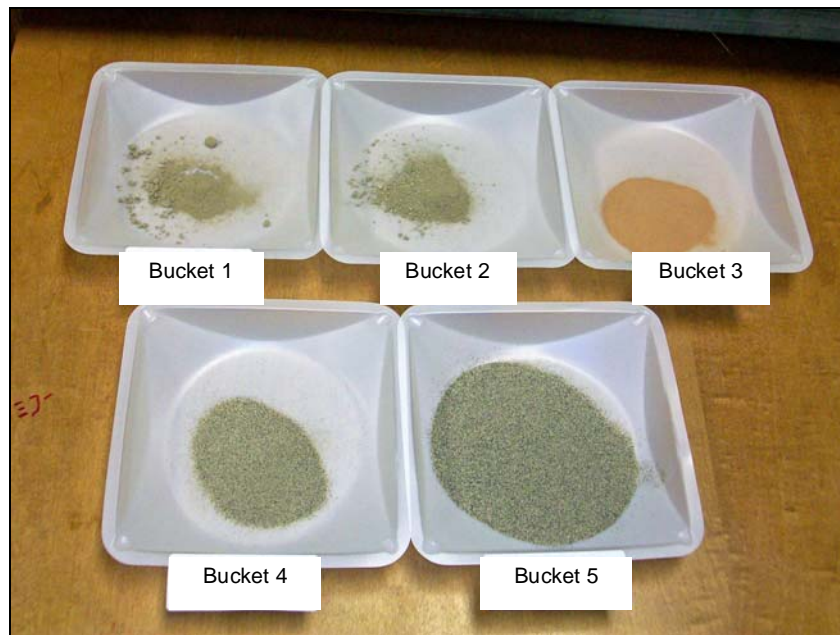
Figure 16. Size fractions obtained by Wilfley Table separation of a Catch Box soil sample identified from smallest density to the greatest density fraction by bucket (Bucket 1 to Bucket 5, respectively).
