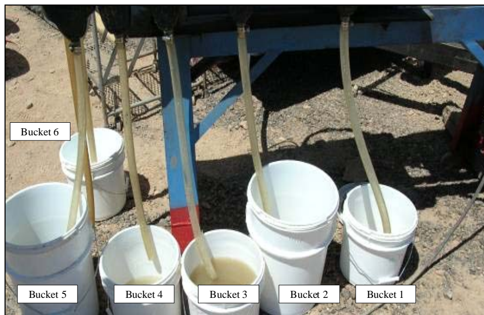
Figure 12. Field operation of the Wilfley Table showing the arrangement of the buckets collecting separation water with the various density fractions of soil.
