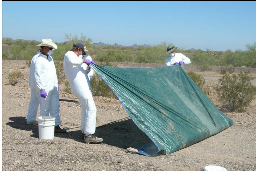
Figure 3. Mixing large soil samples prior to sub-sampling and grinding.
