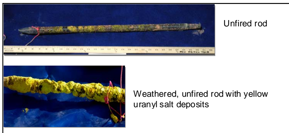
Figure 1. Comparison of weathered and unweathered depleted uranium rods illustrating the formation of uranyl oxides and salts.
