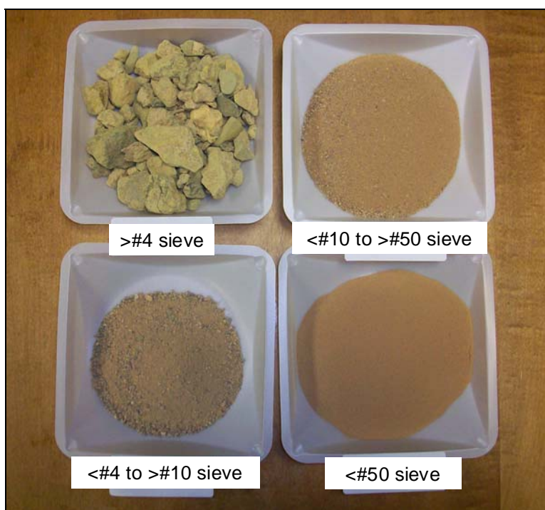
Figure 13. An example of the appearance of the size fractions obtained through dry sieving. These are the four size fractions obtained from a DU Garden soil sample.
