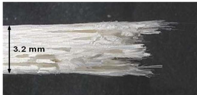
Figure 606. Fracture surface of the N720/AM specimen tested in creep at 131 MPa in steam at 1000°C (side view).
