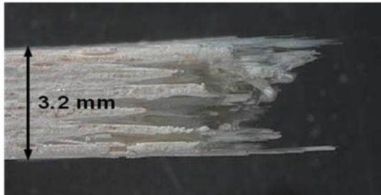
Figure 508. Fracture surface of the N720/AM specimen tested in tension to failure at 900°C in laboratory air (side view).
