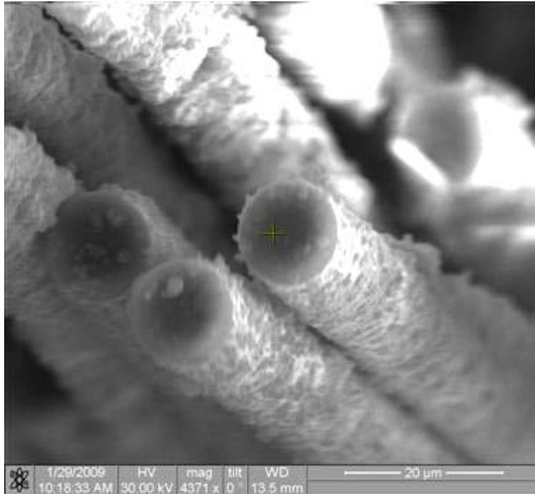
Figure 423. Fracture surface of the N720/AM specimen tested in creep at 131 MPa in steam at 1000°C.
