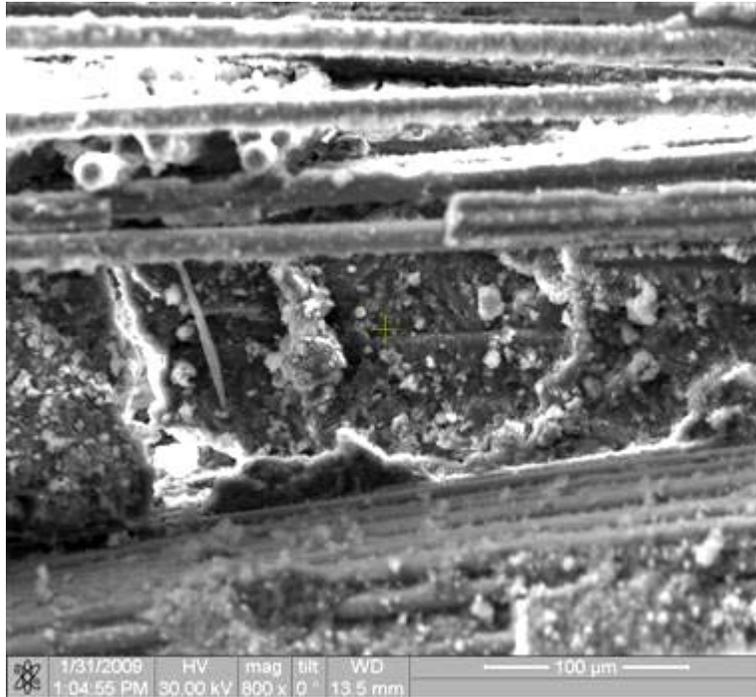
Figure 495. Fracture surface of the N720/AM specimen tested in creep at 140 MPa in steam at 1000°C.
