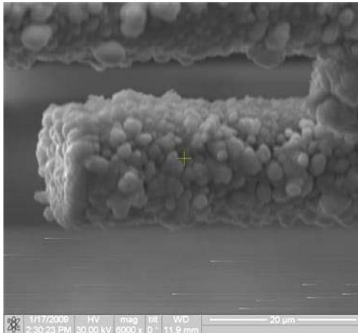
Figure 89. Fracture surface of the N720/AM specimen tested in tension to failure at 1000°C in laboratory air
