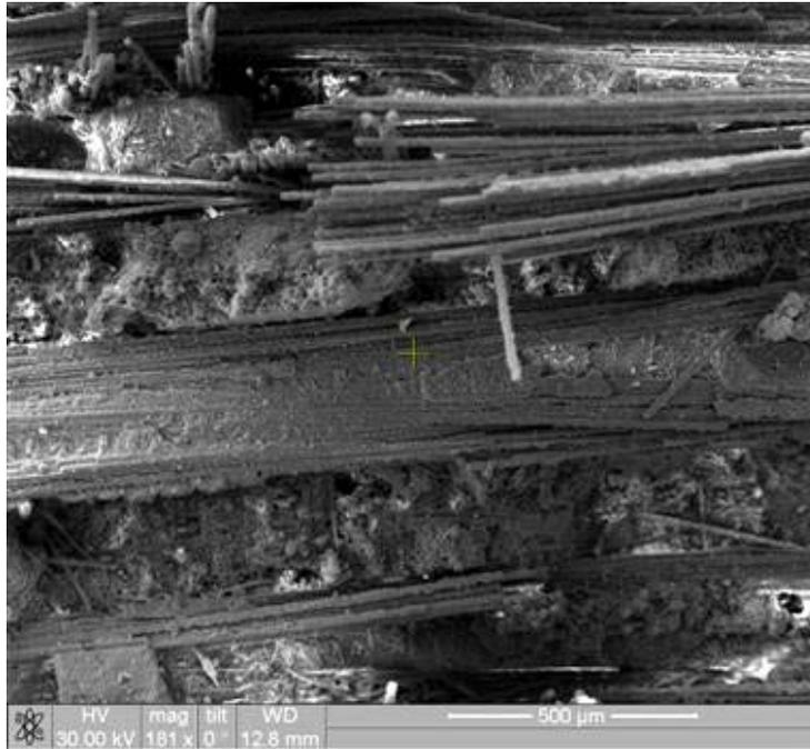
Figure 215. Fracture surface of the N720/AM specimen tested in creep at 109 MPa in laboratory air at 1100°C.
