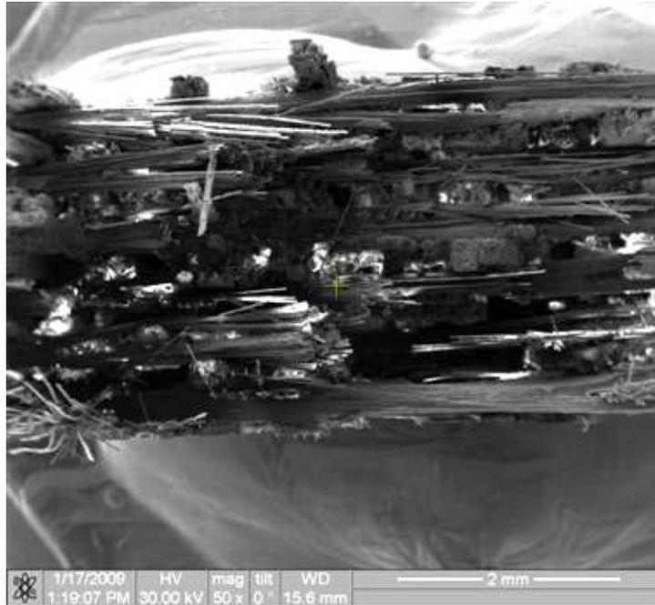
Figure 54. Fracture surface of the N720/AM specimen tested in tension to failure at 900°C in laboratory air
