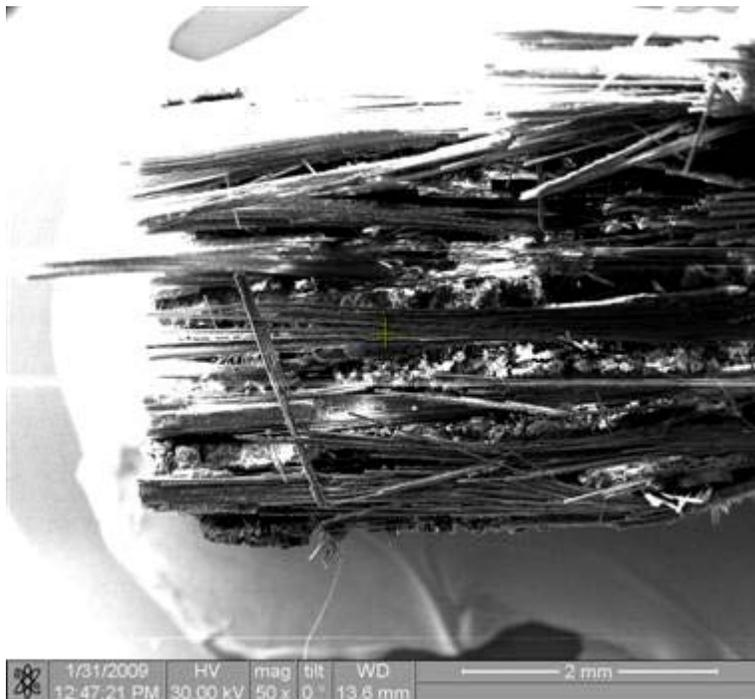
Figure 482. Fracture surface of the N720/AM specimen tested in creep at 140 MPa in steam at 1000°C.
