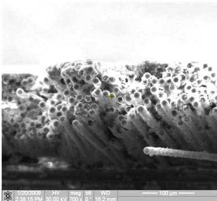
Figure 366. Fracture surface of the N720/AM specimen tested in creep at 87.5 MPa in steam at 1100°C.
