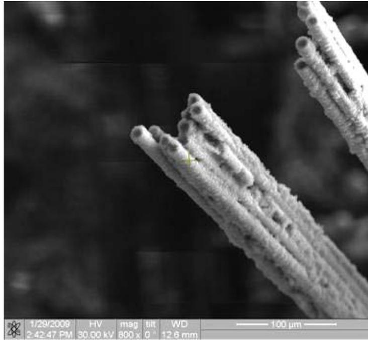
Figure 136. Fracture surface of the N720/AM specimen tested in tension to failure with constant loading rate of 25MPa at 1100°C in steam.
