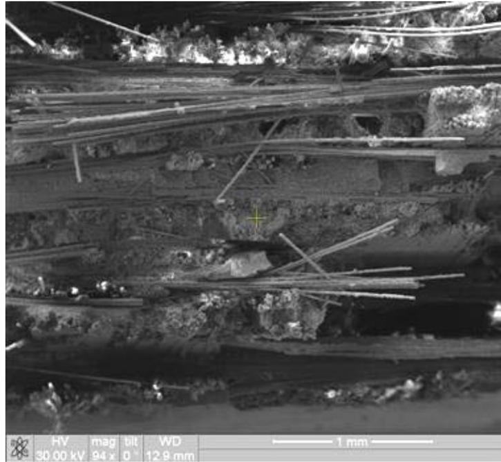
Figure 235. Fracture surface of the N720/AM specimen tested in creep at 109 MPa in laboratory air at 1100°C.
