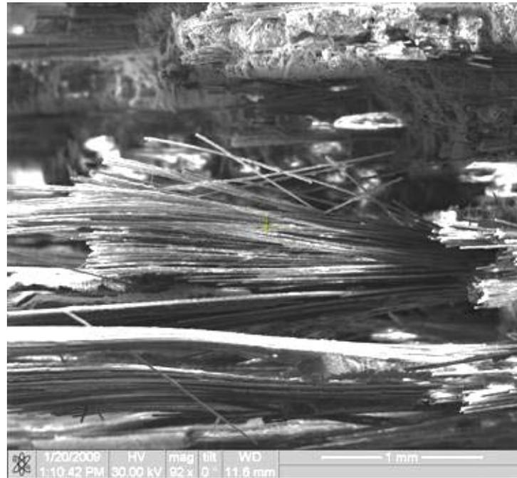
Figure 248. Fracture surface of the N720/AM specimen tested in creep at 131 MPa in laboratory air at 1100°C.
