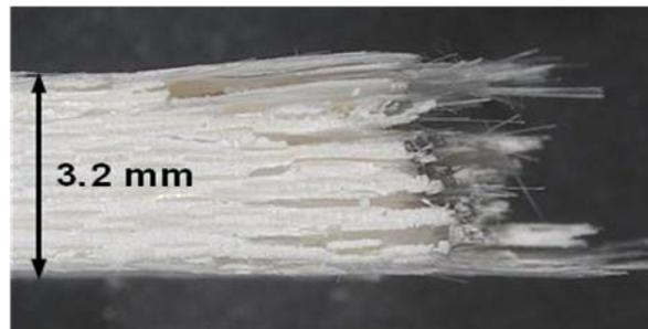
Figure 605. Fracture surface of the N720/AM specimen tested in creep at 131 MPa in steam at 1000°C (side view).
