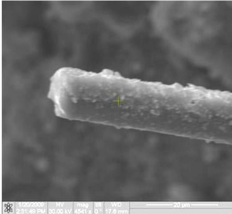
Figure 361. Fracture surface of the N720/AM specimen tested in creep at 87.5 MPa in steam at 1100°C.
