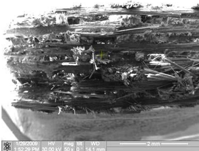
Figure 300. Fracture surface of the N720/AM specimen tested in creep at 131 MPa in steam at 1100°C.
