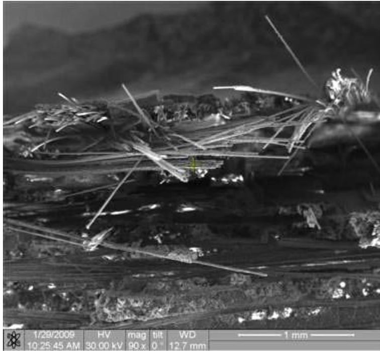
Figure 425. Fracture surface of the N720/AM specimen tested in creep at 131 MPa in steam at 1000°C.
