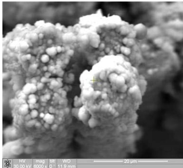
Figure 212. Fracture surface of the N720/AM specimen tested in creep at 109 MPa in laboratory air at 1100°C.
