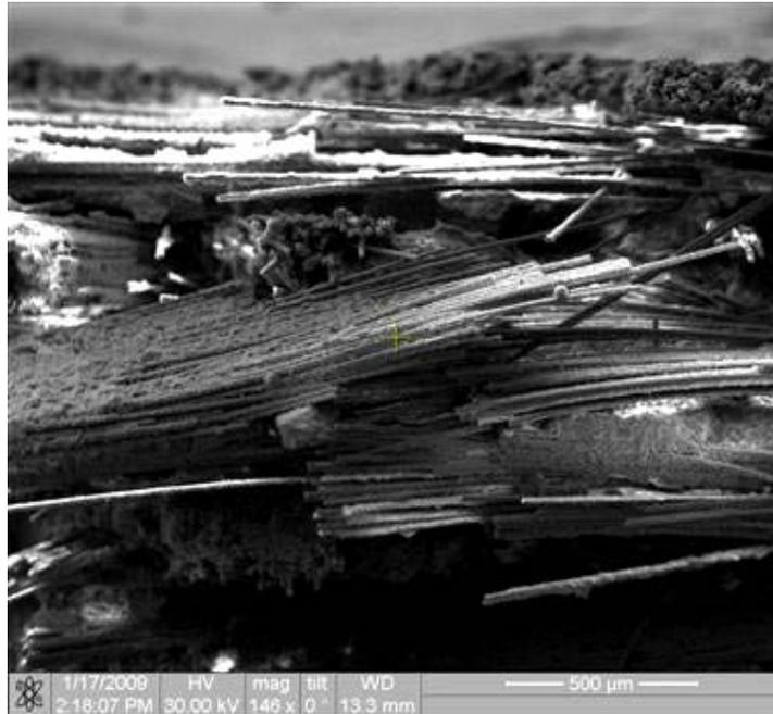
Figure 76. Fracture surface of the N720/AM specimen tested in tension to failure at 1000°C in laboratory air
