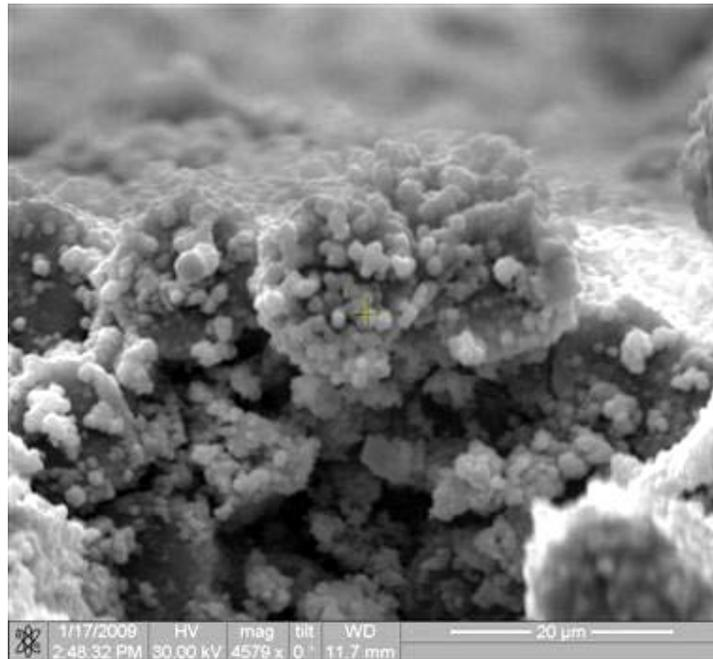
Figure 97. Fracture surface of the N720/AM specimen tested in tension to failure at 1000°C in laboratory air
