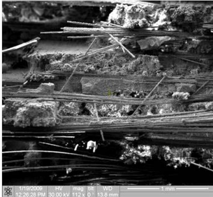
Figure 130. Fracture surface of the N720/AM specimen tested in tension to failure at 1000°C in laboratory air
