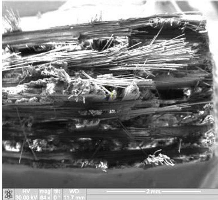
Figure 223. Fracture surface of the N720/AM specimen tested in creep at 109 MPa in laboratory air at 1100°C.
