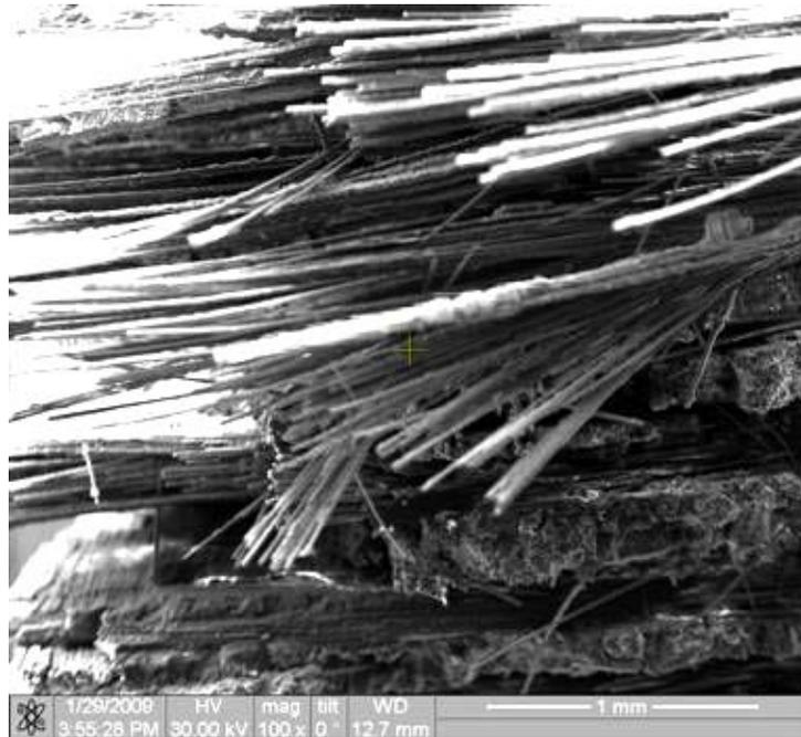
Figure 154. Fracture surface of the N720/AM specimen tested in tension to failure with constant loading rate of 25MPa at 1100°C in steam.
