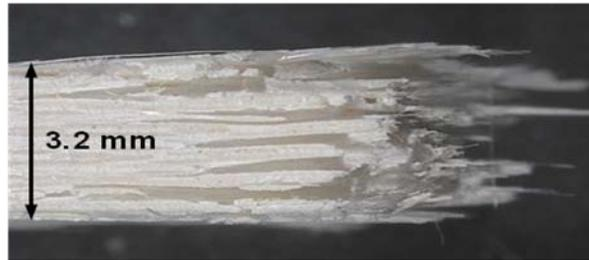
Figure 573. Fracture surface of the N720/AM specimen tested in creep at 131 MPa in laboratory air at 1100°C (side view).
