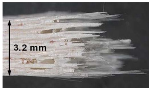
Figure 526. Fracture surface of the N720/AM specimen tested in tension to failure at 1100°C in laboratory air (side view).
