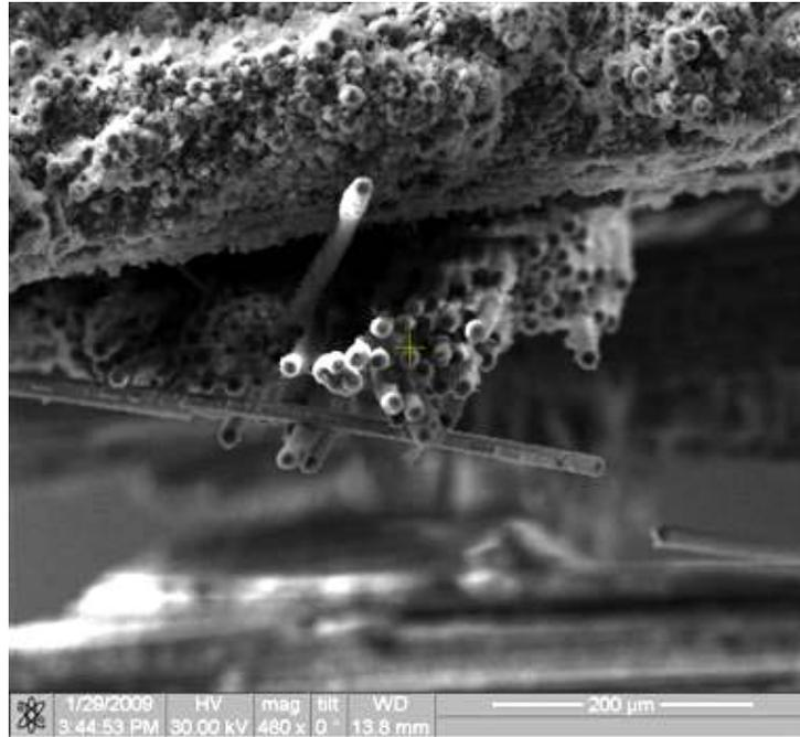
Figure 142. Fracture surface of the N720/AM specimen tested in tension to failure with constant loading rate of 25MPa at 1100°C in steam.
