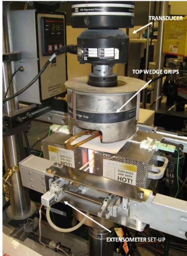
Figure 11. Mechanical Test System.
