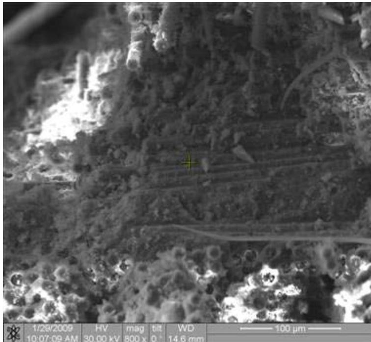
Figure 414. Fracture surface of the N720/AM specimen tested in creep at 131 MPa in steam at 1000°C.
