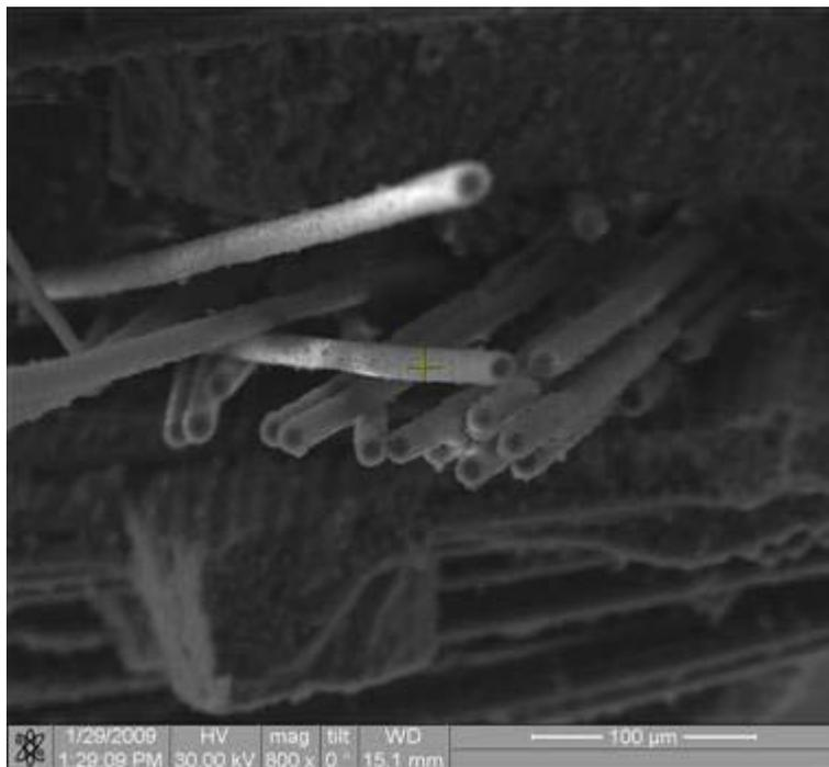
Figure 472. Fracture surface of the N720/AM specimen tested in creep at 140 MPa in steam at 1000°C.
