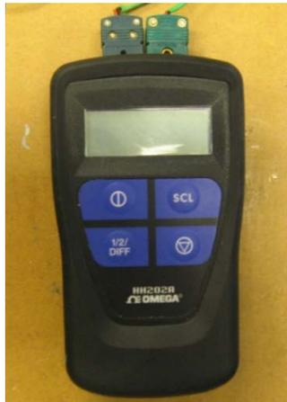
Figure 18. Omega Engineering, Inc, OMNI-CAL-8A-110 Portable Temperature Reader
