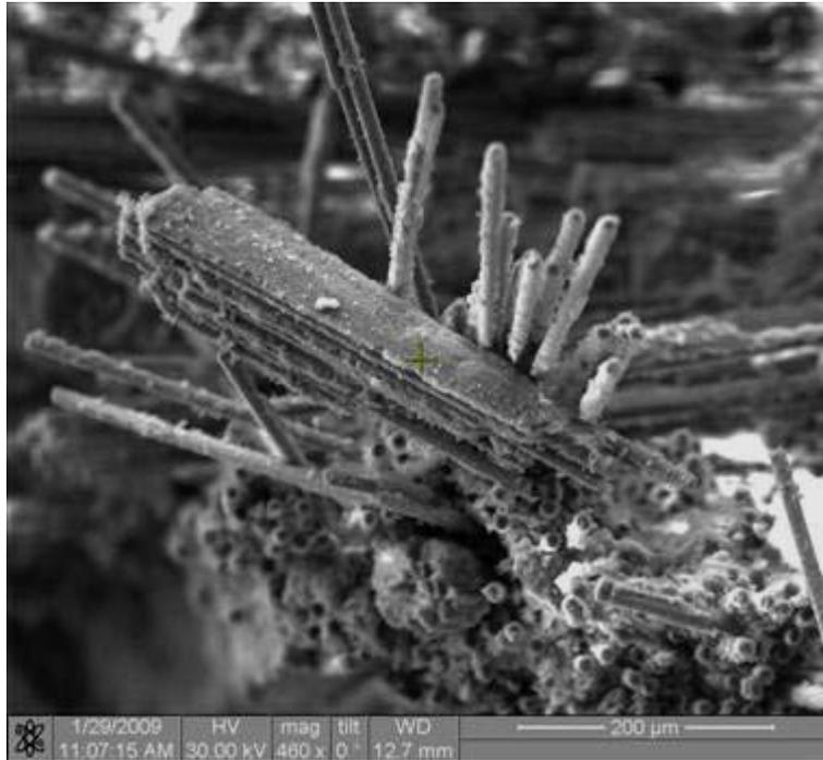
Figure 457. Fracture surface of the N720/AM specimen tested in creep at 131 MPa in steam at 1000°C.
