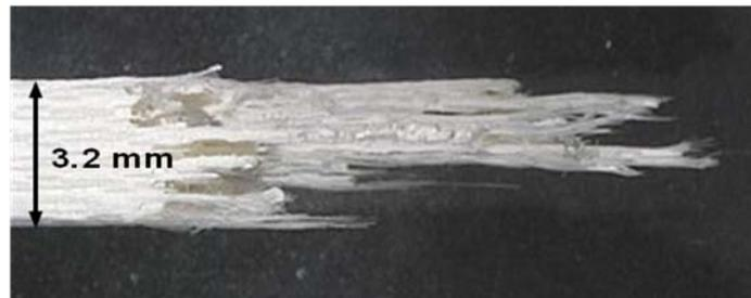
Figure 589. Fracture surface of the N720/AM specimen tested in creep at 109 MPa in steam at 1100°C (side view).
