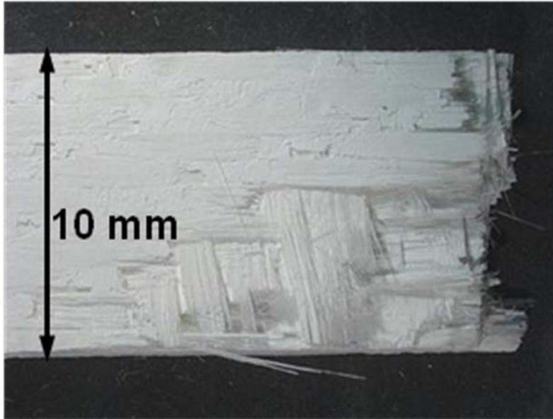
Figure 607. Fracture surface of the N720/AM specimen tested in creep at 140 MPa in steam at 1000°C.
