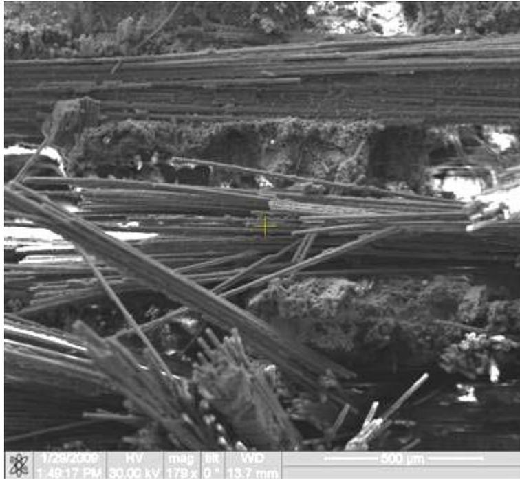
Figure 297. Fracture surface of the N720/AM specimen tested in creep at 131 MPa in steam at 1100°C.
