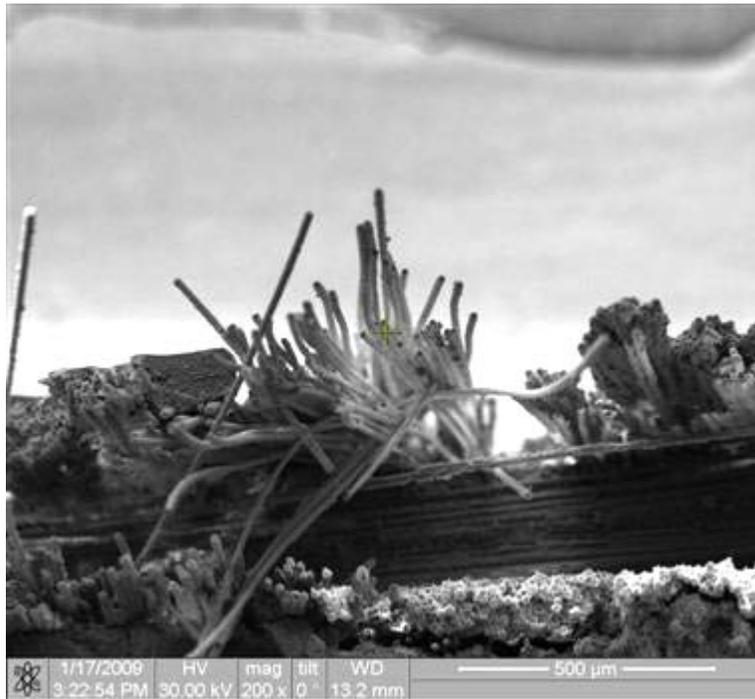
Figure 111. Fracture surface of the N720/AM specimen tested in tension to failure at 1100°C in laboratory air
