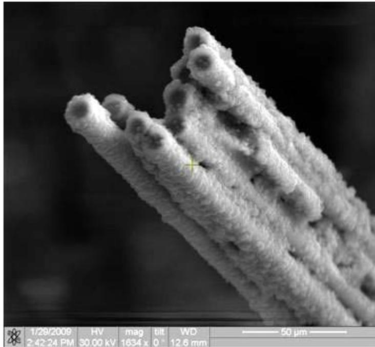
Figure 137. Fracture surface of the N720/AM specimen tested in tension to failure with constant loading rate of 25MPa at 1100°C in steam.
