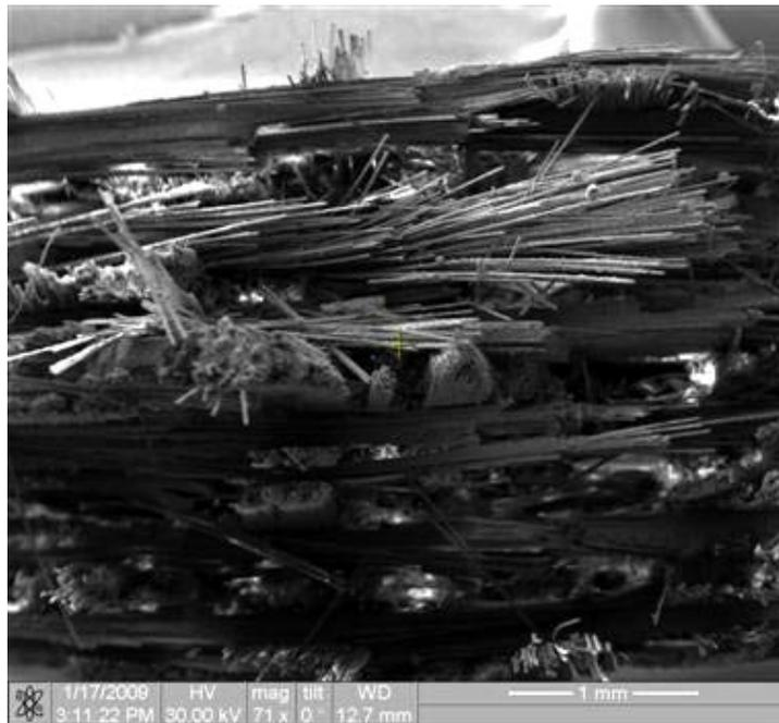
Figure 103. Fracture surface of the N720/AM specimen tested in tension to failure at 1100°C in laboratory air
