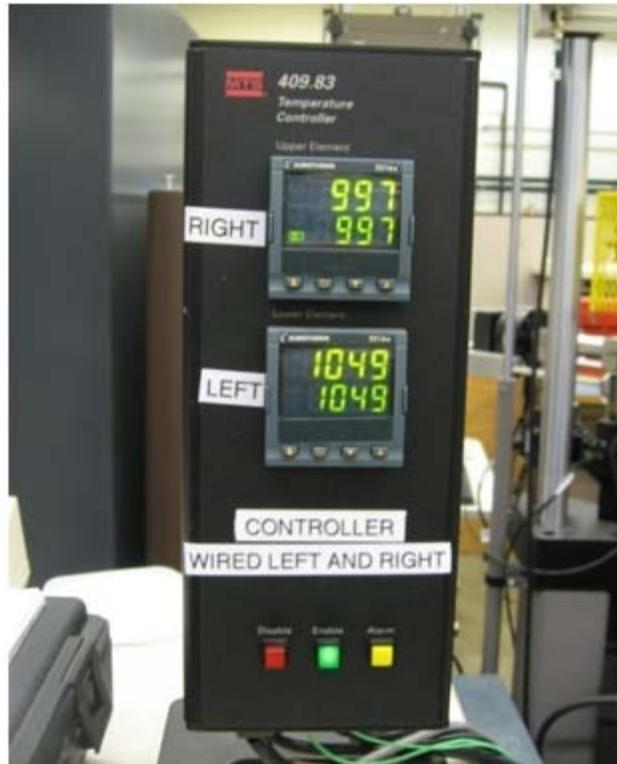
Figure 13. MTS Model 409.83B Temperature Controller.
