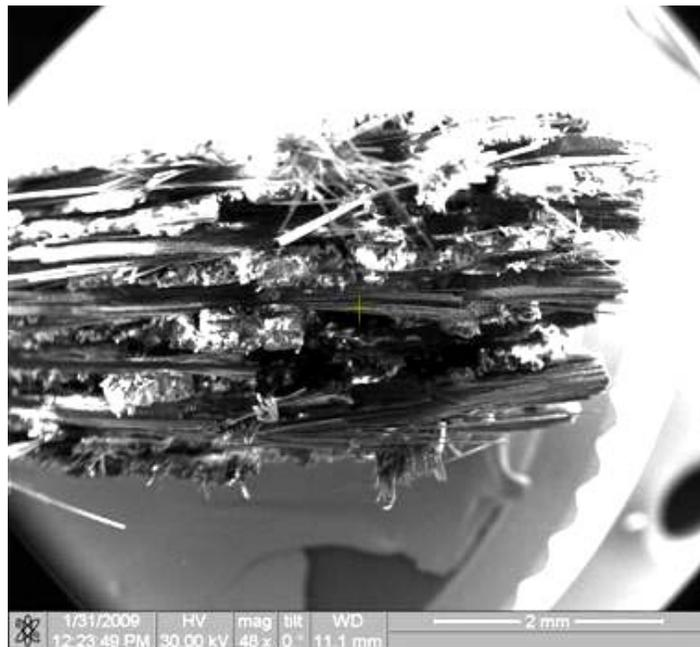
Figure 179. Fracture surface of the N720/AM specimen tested in tension to failure with constant loading rate of 25MPa at 1100°C in steam.
