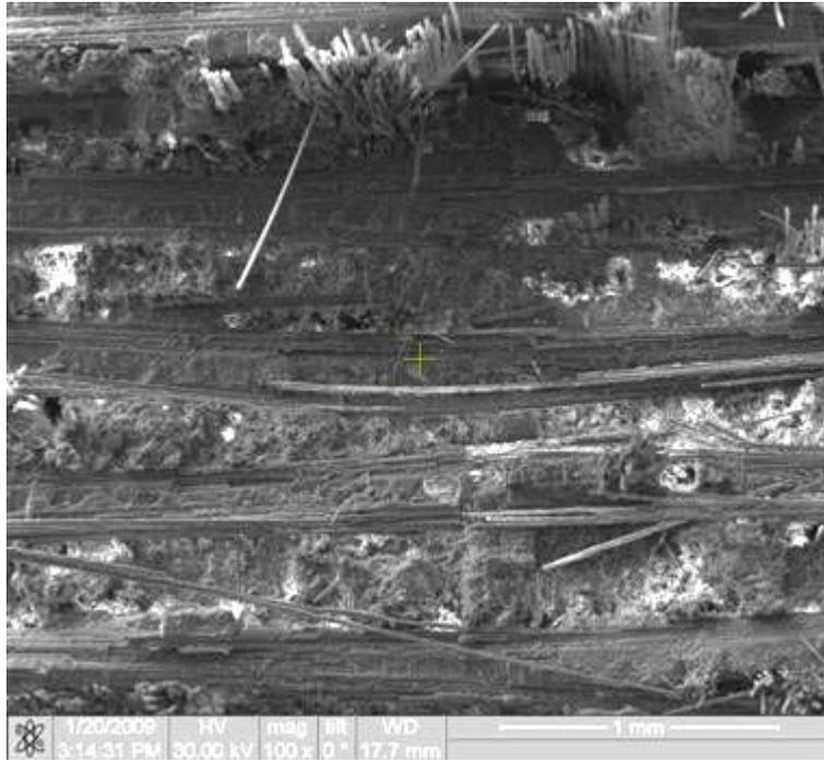
Figure 393. Fracture surface of the N720/AM specimen tested in creep at 87.5 MPa in steam at 1100°C.
