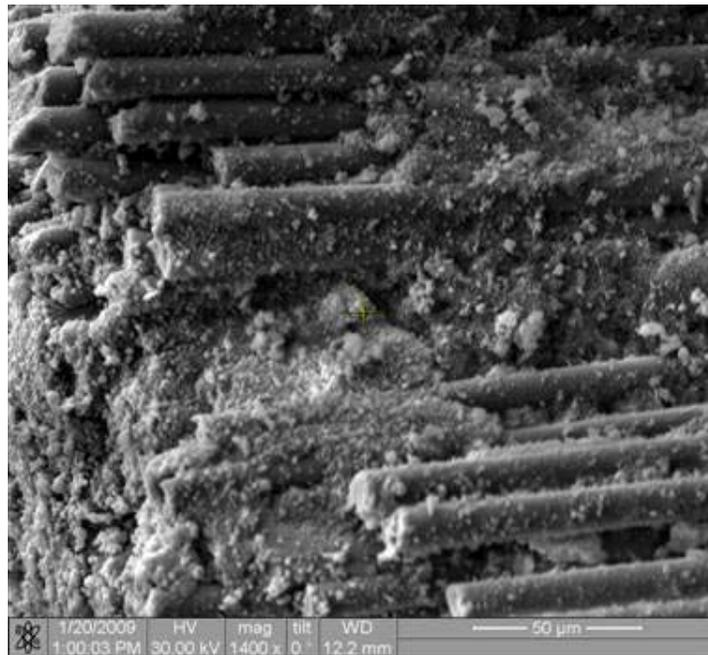
Figure 244. Fracture surface of the N720/AM specimen tested in creep at 131 MPa in laboratory air at 1100°C.
