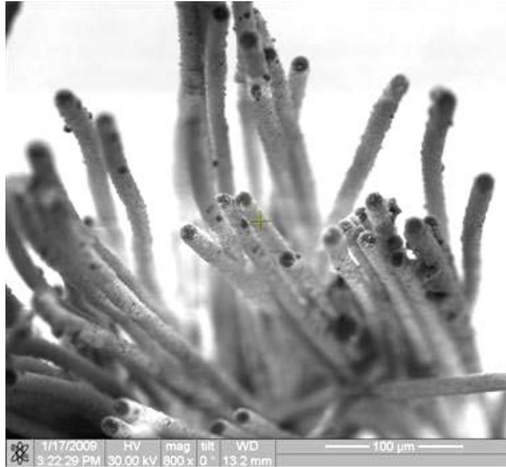
Figure 112. Fracture surface of the N720/AM specimen tested in tension to failure at 1100°C in laboratory air
