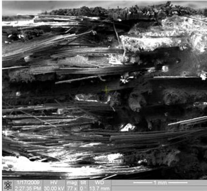
Figure 86. Fracture surface of the N720/AM specimen tested in tension to failure at 1000°C in laboratory air
