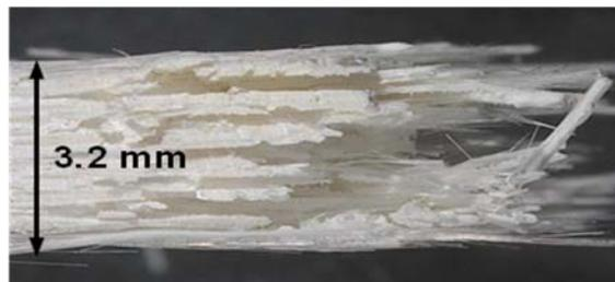
Figure 516. Fracture surface of the N720/AM specimen tested in tension to failure at 1000°C in laboratory air (side view).
