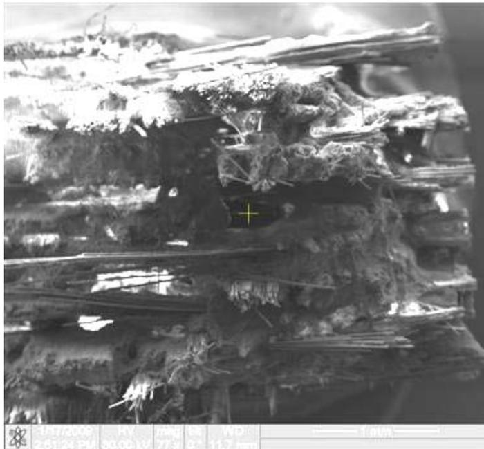
Figure 99. Fracture surface of the N720/AM specimen tested in tension to failure at 1000°C in laboratory air
