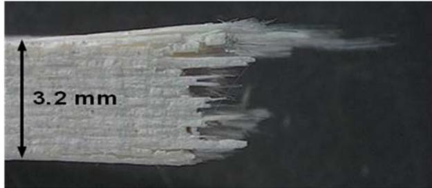
Figure 540. Fracture surface of the N720/AM specimen(2) tested in tension to failure with constant loading rate of 25MPa at 1100°C in steam (side view).
