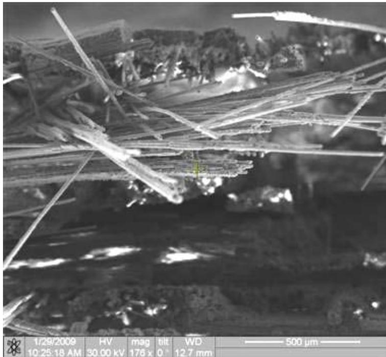
Figure 426. Fracture surface of the N720/AM specimen tested in creep at 131 MPa in steam at 1000°C.
