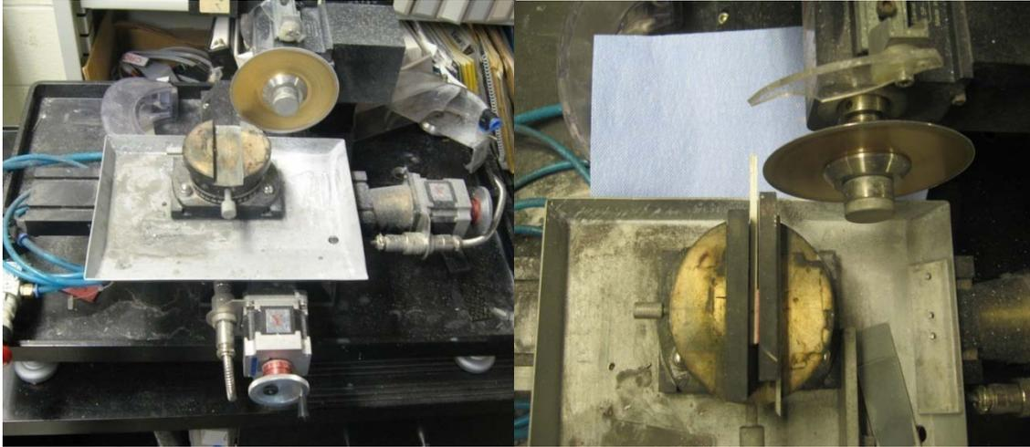
Figure 24. CNC Saw.
