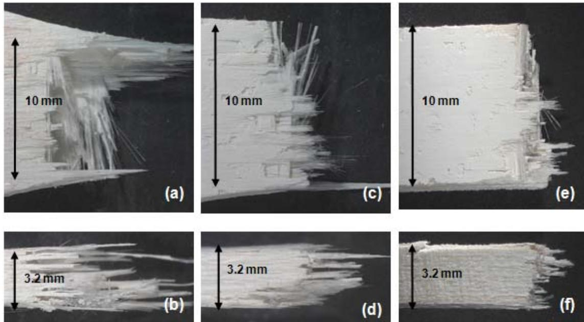
Figure 42. Fracture surfaces of the N720/AM specimens obtained in creep tests in steam at (a-b) 131 MPa (equivalent to 150 MPa for  $V_f=0.44$ ),  $t_f= > 100$  h at 1000 °C and (c-d) 131 MPa (equivalent to 150 MPa for  $V_f=0.44$ ),  $t_f= 4.12$  h at 1100°C (e-f) 136 MPa (equivalent to 150 MPa for  $V_f=0.44$ ),  $t_f= 0.012$  h at 1200°C in steam. Micrographs of the specimen tested in 1200°C from Genelin [16].
