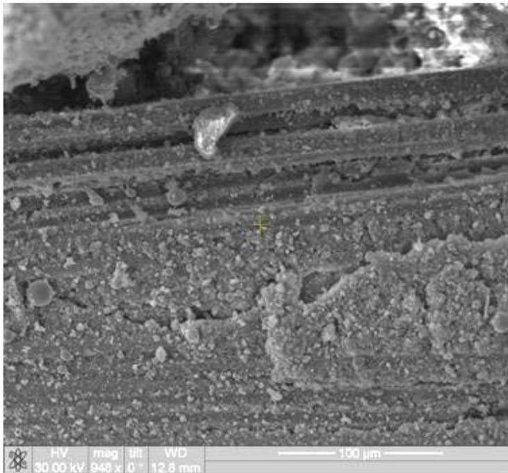
Figure 216. Fracture surface of the N720/AM specimen tested in creep at 109 MPa in laboratory air at 1100°C.
