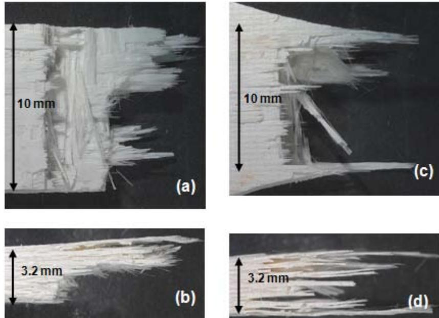
Figure 40. Fracture surfaces of the N720/AM specimens obtained in creep tests at 1100 °C in air at: (a-b) 131MPa (equivalent to 150 MPa for  $V_f=0.44$ ),  $t_f > 100$  h and (c-d) 109 MPa (equivalent to 125 MPa for  $V_f=0.44$ ),  $t_f > 100$ h.
