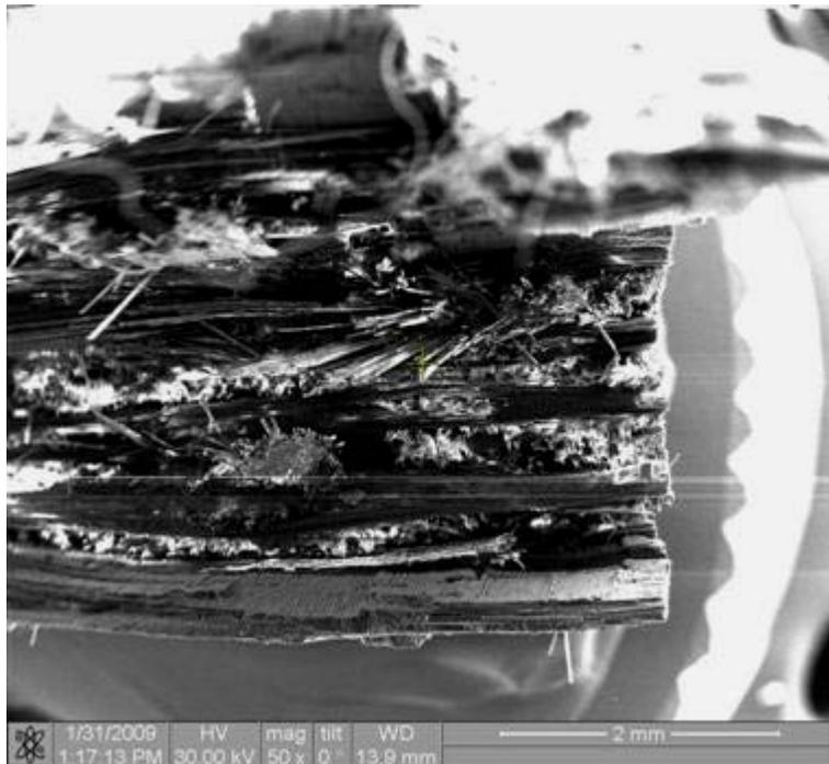
Figure 498. Fracture surface of the N720/AM specimen tested in creep at 140 MPa in steam at 1000°C.
