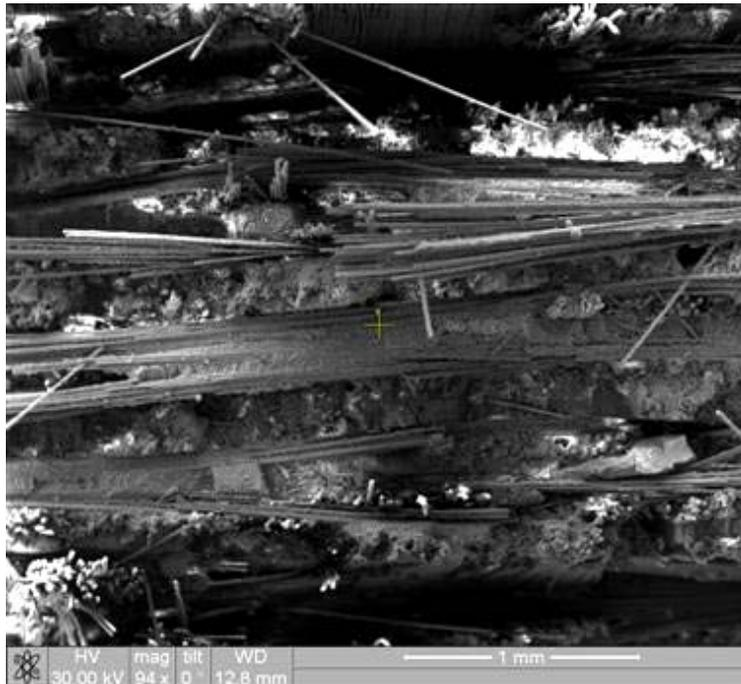
Figure 214. Fracture surface of the N720/AM specimen tested in creep at 109 MPa in laboratory air at 1100°C.
