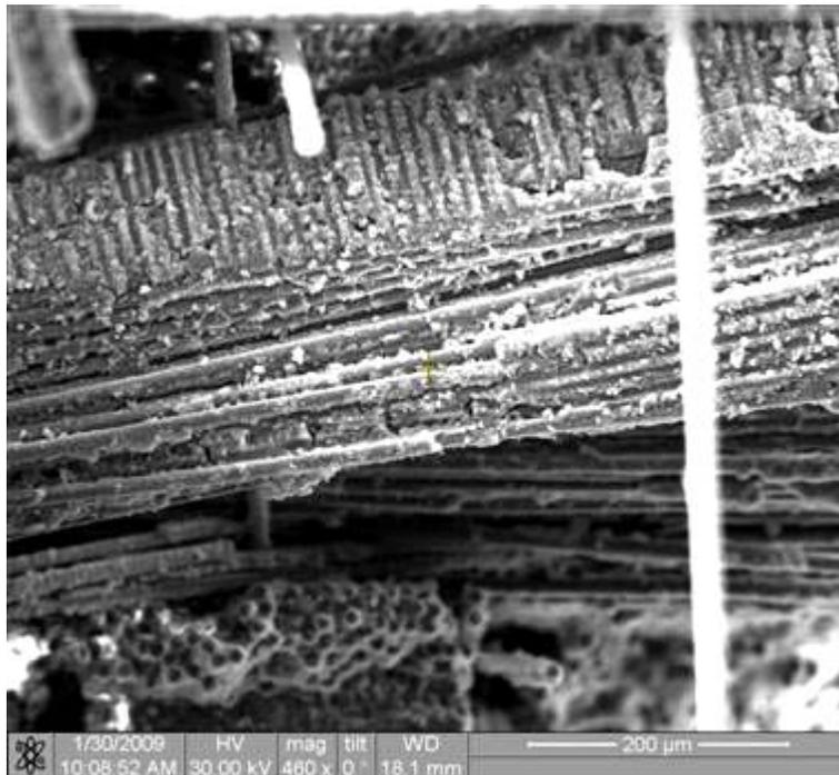
Figure 476. Fracture surface of the N720/AM specimen tested in creep at 140 MPa in steam at 1000°C.
