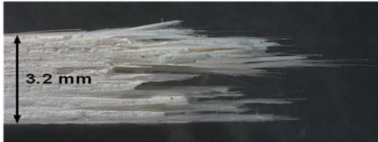
Figure 523. Fracture surface of the N720/AM specimen tested in tension to failure at 1100°C in laboratory air (side view).
