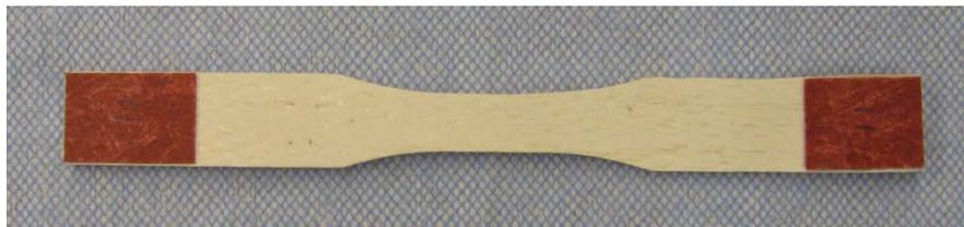
Figure 21. Tabbed Test Specimen.
