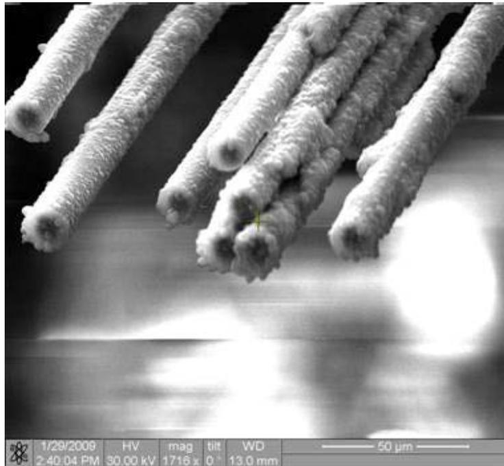
Figure 135. Fracture surface of the N720/AM specimen tested in tension to failure with constant loading rate of 25MPa at 1100°C in steam.
