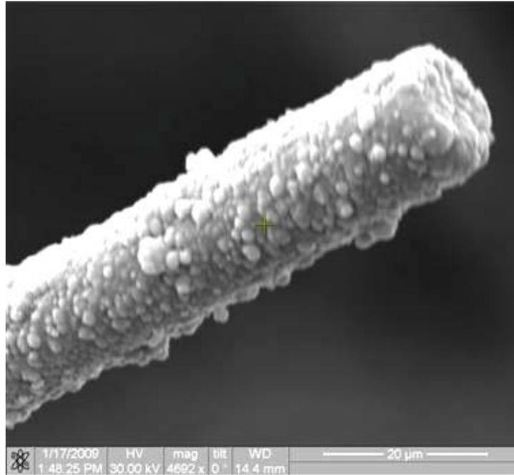
Figure 64. Fracture surface of the N720/AM specimen tested in tension to failure at 900°C in laboratory air
