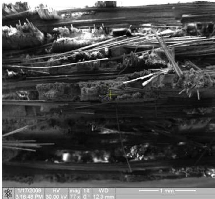
Figure 105. Fracture surface of the N720/AM specimen tested in tension to failure at 1000°C in laboratory air
