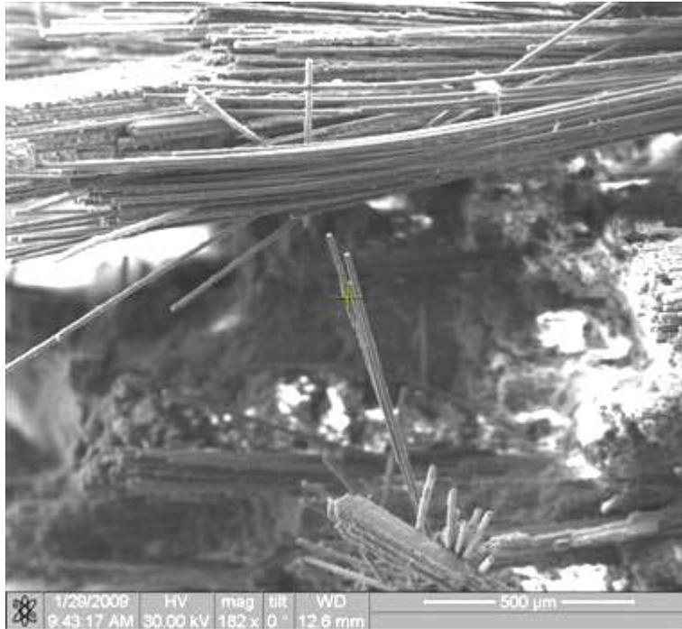
Figure 397. Fracture surface of the N720/AM specimen tested in creep at 131 MPa in steam at 1000°C.
