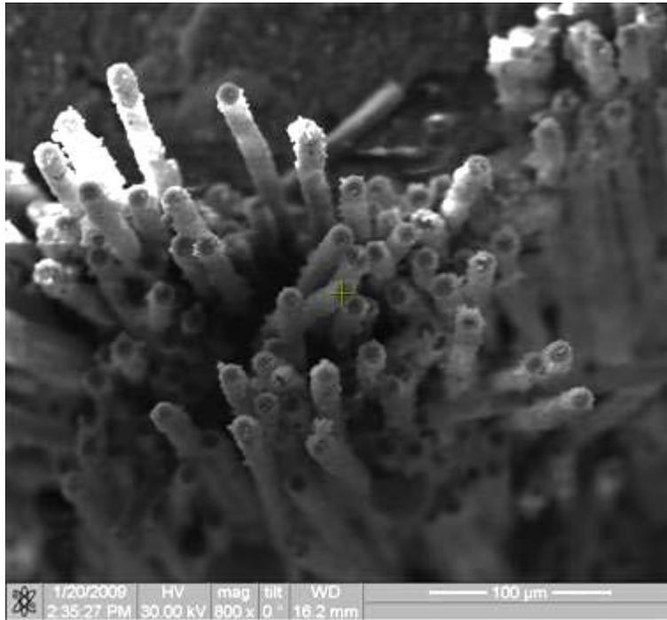
Figure 363. Fracture surface of the N720/AM specimen tested in creep at 87.5 MPa in steam at 1100°C.
