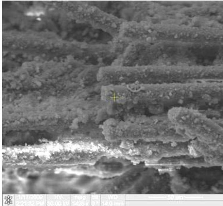
Figure 84. Fracture surface of the N720/AM specimen tested in tension to failure at 1000°C in laboratory air
