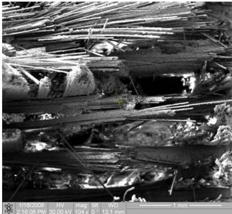
Figure 202. Fracture surface of the N720/AM specimen tested in creep at 109 MPa in laboratory air at 1100°C.
