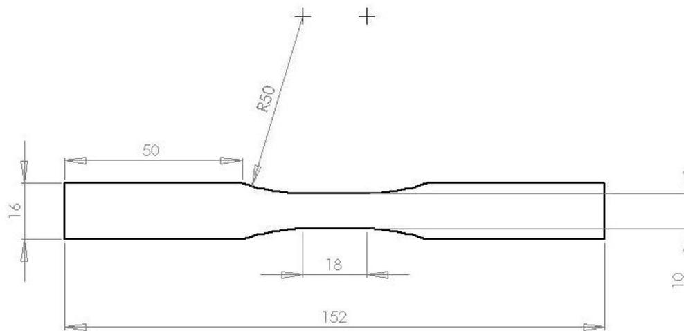
Figure 19. Uniaxial test specimen (dimensions in mm) [18].
