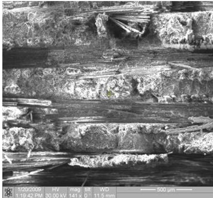
Figure 255. Fracture surface of the N720/AM specimen tested in creep at 131 MPa in laboratory air at 1100°C.
