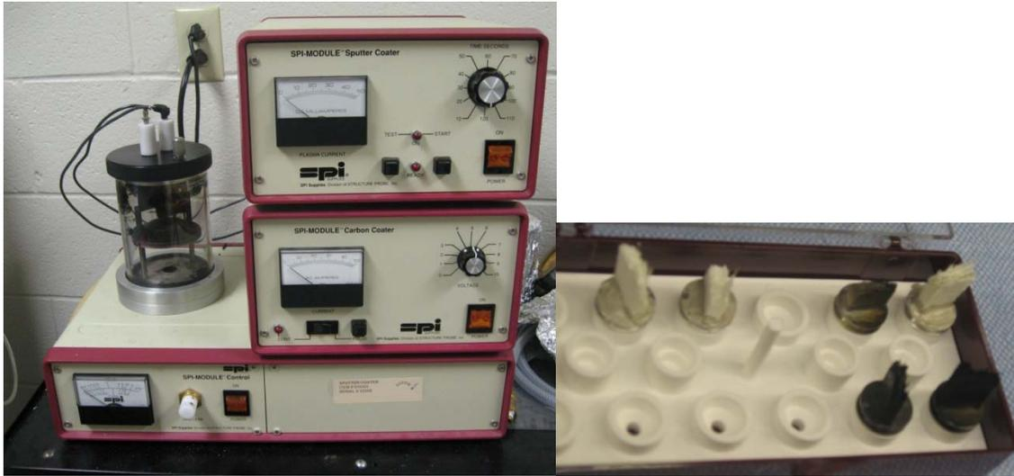
Figure 25. (a) SPI Carbon Coating Machine (b) Carbon-coated failed specimens in the storage box.
