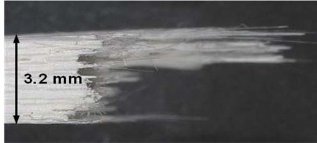
Figure 595. Fracture surface of the N720/AM specimen tested in creep at 87.5 MPa in steam at 1100°C (side view).
