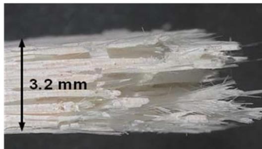
Figure 574. Fracture surface of the N720/AM specimen tested in creep at 131 MPa in laboratory air at 1100°C (side view).
