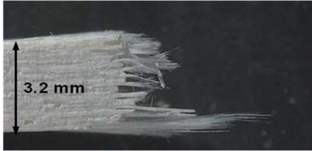
Figure 539. Fracture surface of the N720/AM specimen(2) tested in tension to failure with constant loading rate of 25MPa at 1100°C in steam (side view).
