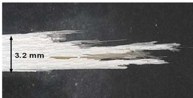
Figure 590. Fracture surface of the N720/AM specimen tested in creep at 109 MPa in steam at 1100°C (side view).
