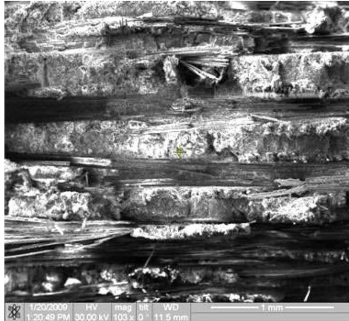
Figure 254. Fracture surface of the N720/AM specimen tested in creep at 131 MPa in laboratory air at 1100°C.
