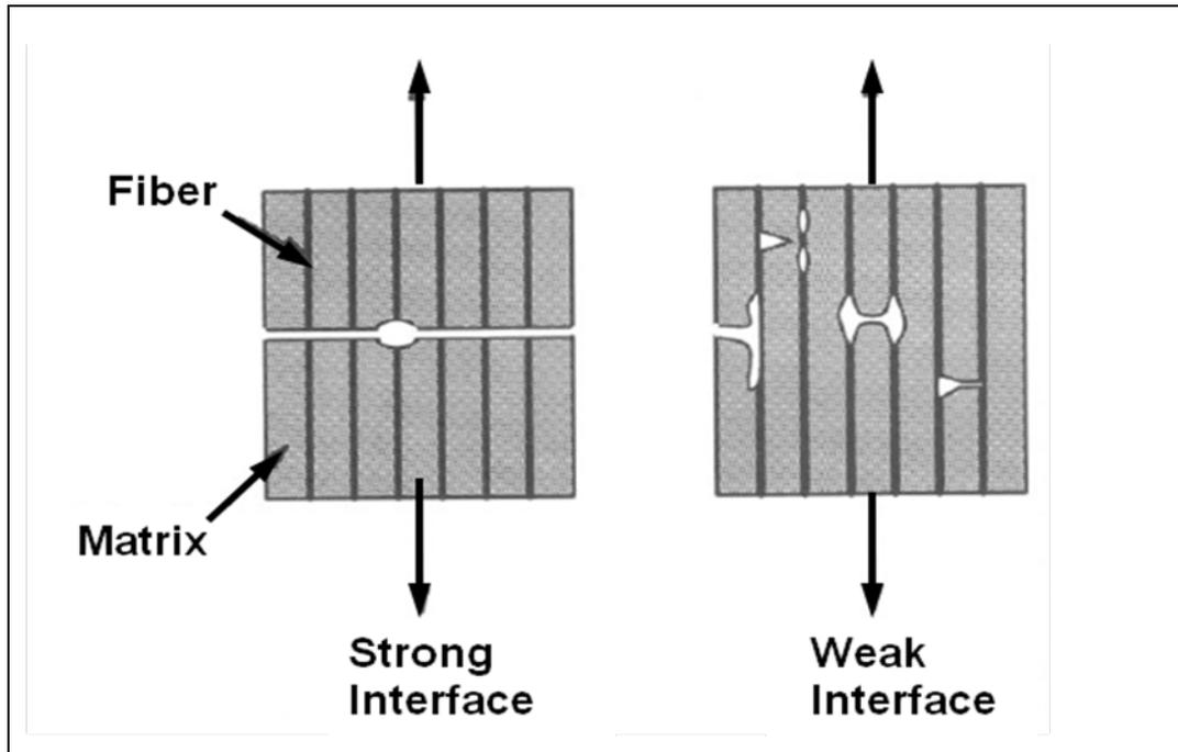
Figure 2. Failure of CMC as a function of interfacial bond strength
