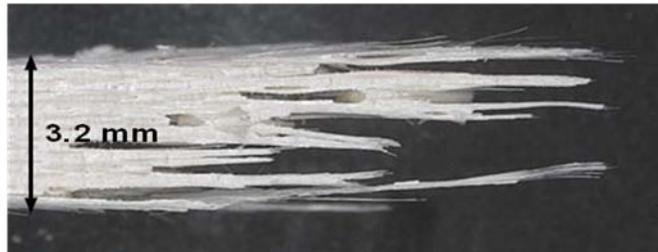
Figure 604. Fracture surface of the N720/AM specimen tested in creep at 131 MPa in steam at 1000°C (side view).
