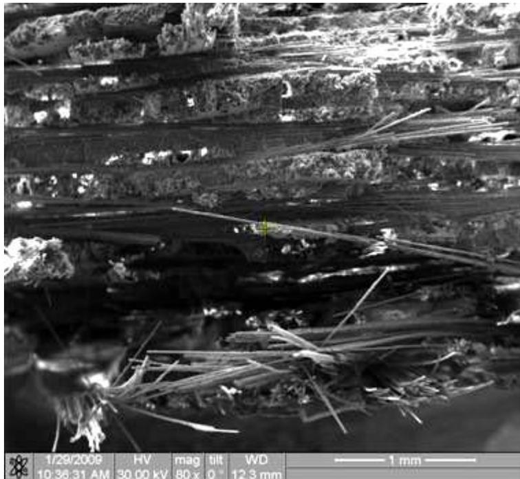
Figure 436. Fracture surface of the N720/AM specimen tested in creep at 131 MPa in steam at 1000°C.
