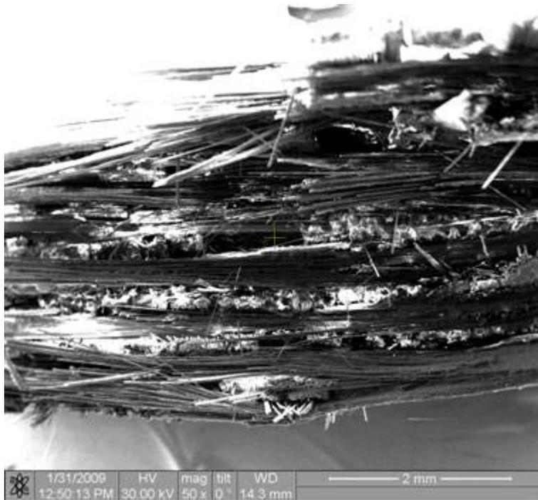
Figure 485. Fracture surface of the N720/AM specimen tested in creep at 140 MPa in steam at 1000°C.
