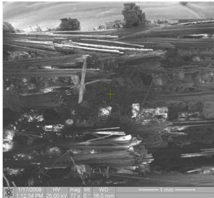
Figure 51. Fracture surface of the N720/AM specimen tested in tension to failure at 900°C in laboratory air
