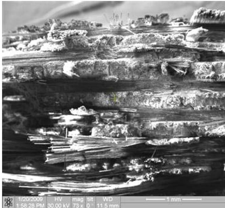
Figure 271. Fracture surface of the N720/AM specimen tested in creep at 131 MPa in laboratory air at 1100°C.
