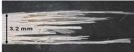
Figure 571. Fracture surface of the N720/AM specimen tested in creep at 131 MPa in laboratory air at 1100°C (side view).
