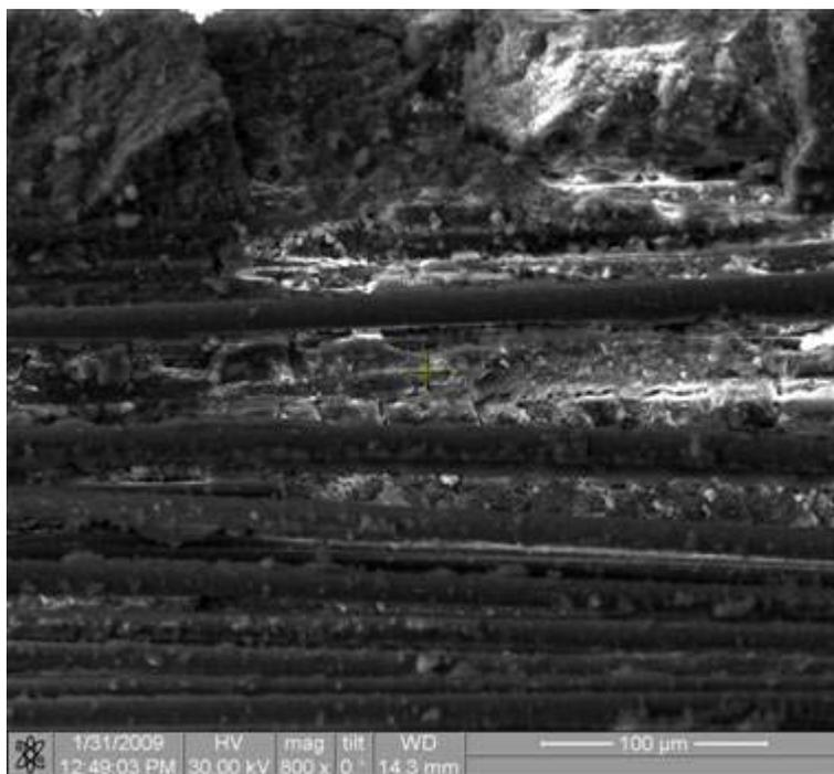
Figure 486. Fracture surface of the N720/AM specimen tested in creep at 140 MPa in steam at 1000°C.
