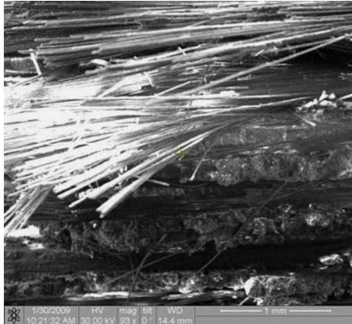
Figure 158. Fracture surface of the N720/AM specimen tested in tension to failure with constant loading rate of 25MPa at 1100°C in steam.
