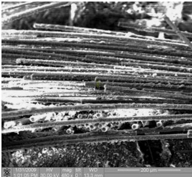
Figure 492. Fracture surface of the N720/AM specimen tested in creep at 140 MPa in steam at 1000°C.
