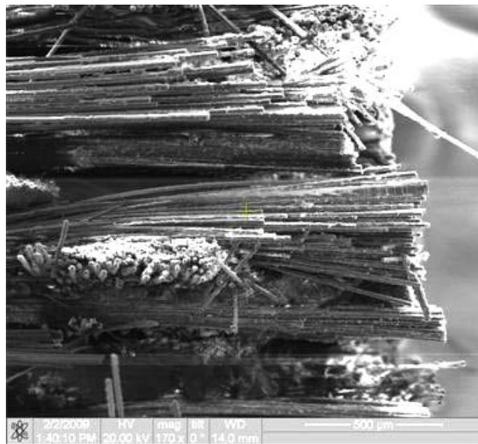
Figure 189 Fracture surface of the N720/AM specimen tested in tension to failure with constant loading rate of 0.0025MPa at 1100°C in steam.
