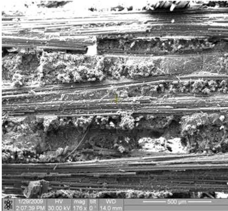
Figure 311. Fracture surface of the N720/AM specimen tested in creep at 131 MPa in steam at 1100°C.
