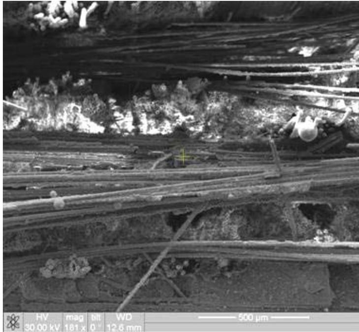
Figure 231. Fracture surface of the N720/AM specimen tested in creep at 109 MPa in laboratory air at 1100°C.
