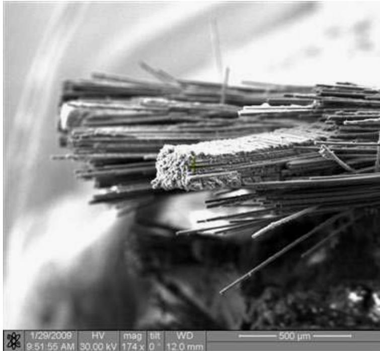
Figure 403. Fracture surface of the N720/AM specimen tested in creep at 131 MPa in steam at 1000°C.
