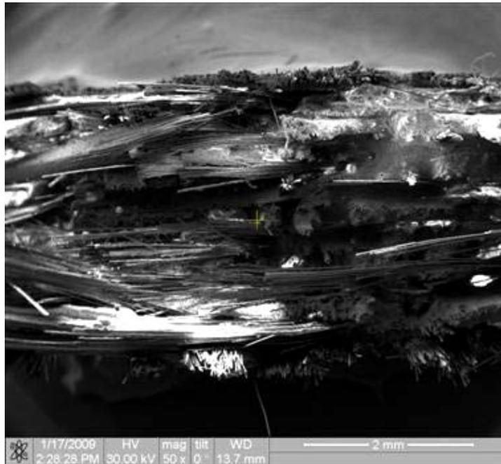
Figure 85. Fracture surface of the N720/AM specimen tested in tension to failure at 1000°C in laboratory air
