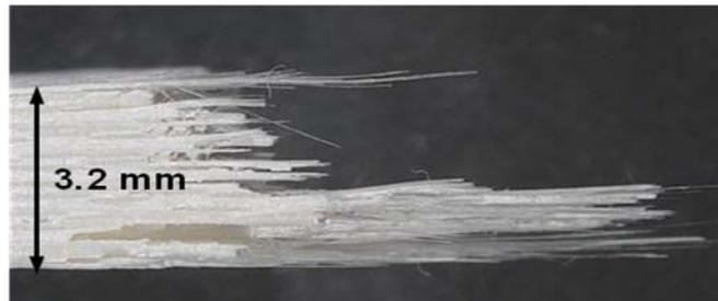
Figure 596. Fracture surface of the N720/AM specimen tested in creep at 87.5 MPa in steam at 1100°C (side view).
