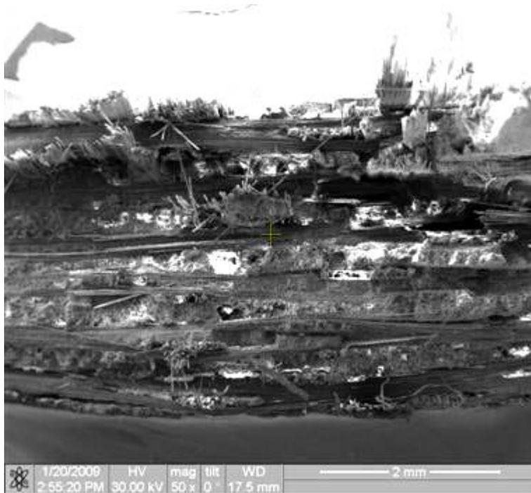
Figure 379. Fracture surface of the N720/AM specimen tested in creep at 87.5 MPa in steam at 1100°C.
