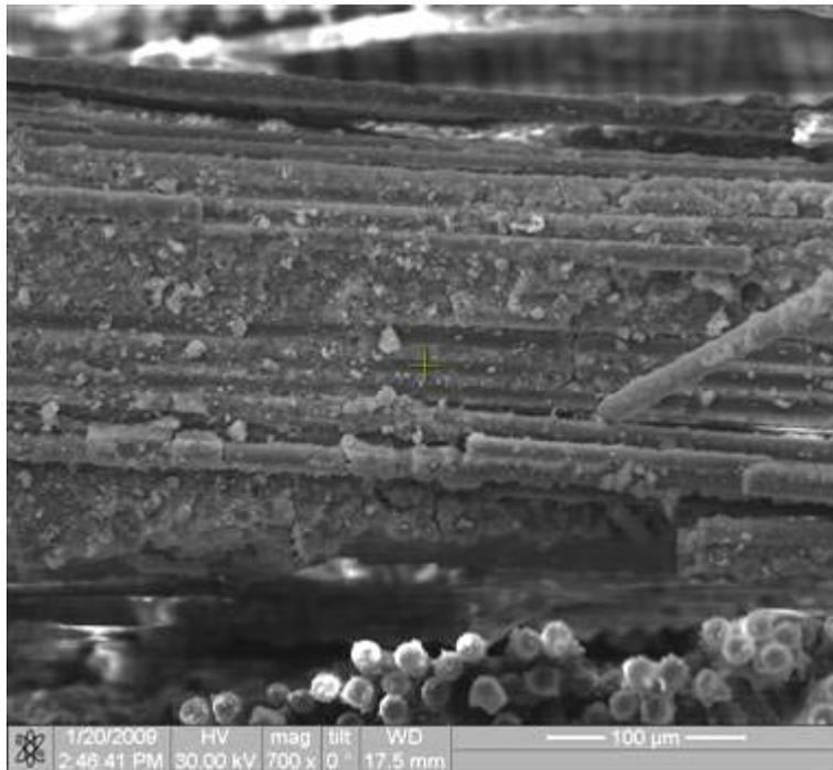
Figure 372. Fracture surface of the N720/AM specimen tested in creep at 87.5 MPa in steam at 1100°C.
