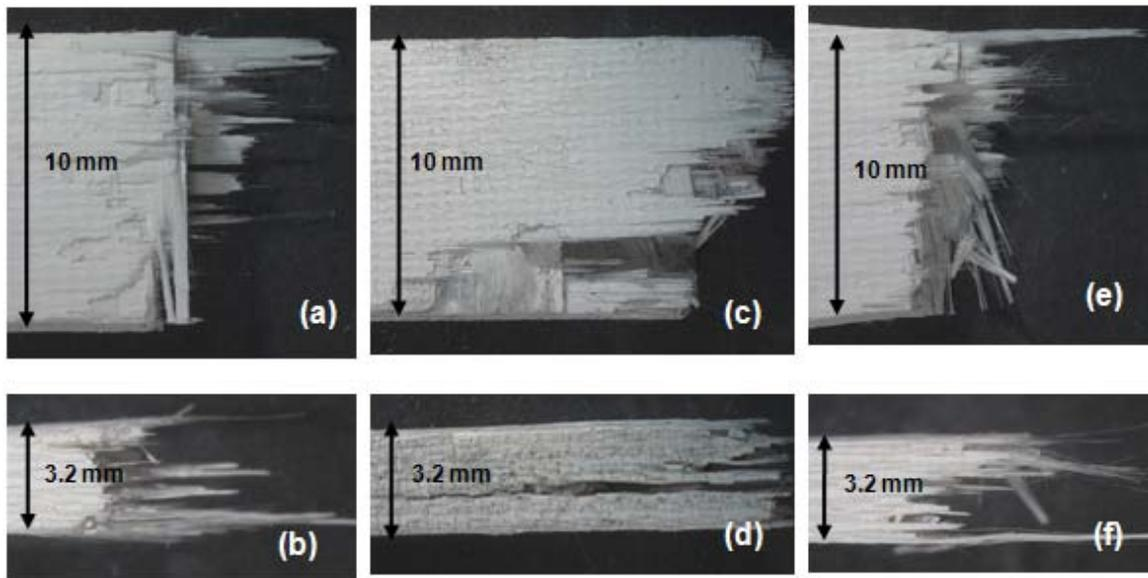
Figure 41. Fracture surfaces of the N720/AM specimens obtained in creep tests at 1100 °C in steam at: (a-b) 87.5MPa (equivalent to 100 MPa for  $V_f=0.44$ ),  $t_f = >100$  h and (c-d) 109 MPa (equivalent to 125 MPa for  $V_f=0.44$ ),  $t_f= 35.2$  h (e-f) 131 MPa (equivalent to 150 MPa for  $V_f=0.44$ ),  $t_f= 4.12$ .
