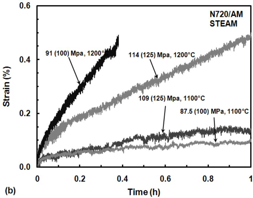
Figure 33. Creep strain vs. time curves for N720/AM ceramic matrix composite at 1000, 1100 and 1200 °C in steam. Data at 1200 °C from Genelin [16]. Stress levels adjusted for  $V_f = 0.44$  are shown in parentheses.
