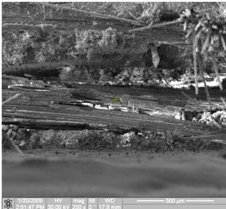
Figure 376. Fracture surface of the N720/AM specimen tested in creep at 87.5 MPa in steam at 1100°C.
