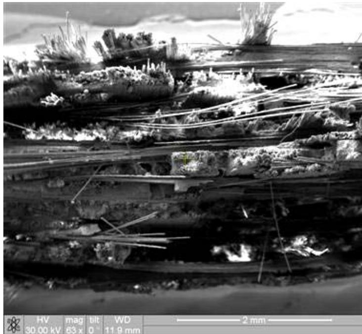
Figure 218. Fracture surface of the N720/AM specimen tested in creep at 109 MPa in laboratory air at 1100°C.
