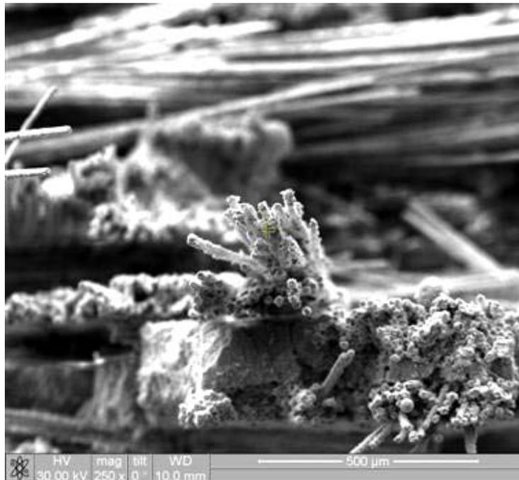
Figure 228. Fracture surface of the N720/AM specimen tested in creep at 109 MPa in laboratory air at 1100°C.
