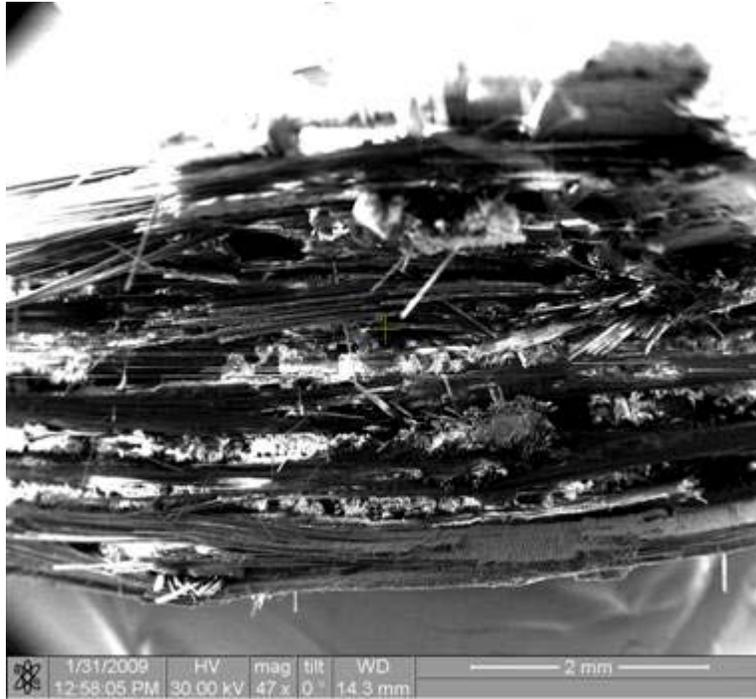
Figure 489. Fracture surface of the N720/AM specimen tested in creep at 140 MPa in steam at 1000°C.
