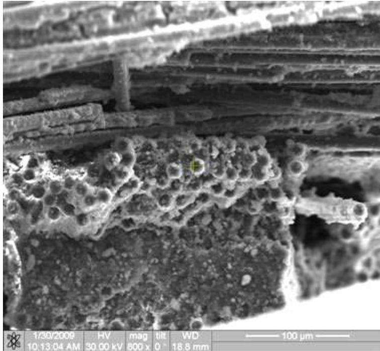
Figure 479. Fracture surface of the N720/AM specimen tested in creep at 140 MPa in steam at 1000°C.
