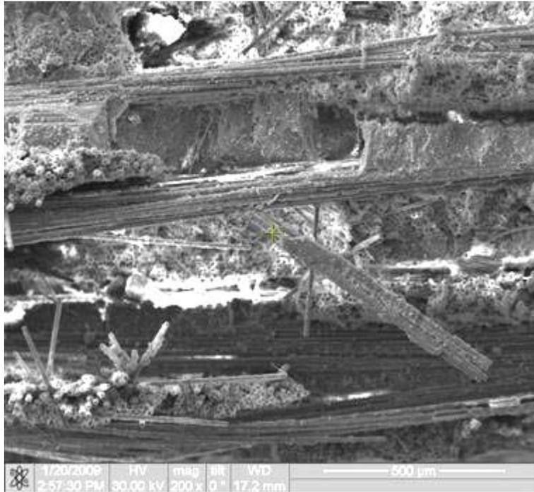
Figure 381. Fracture surface of the N720/AM specimen tested in creep at 87.5 MPa in steam at 1100°C.
