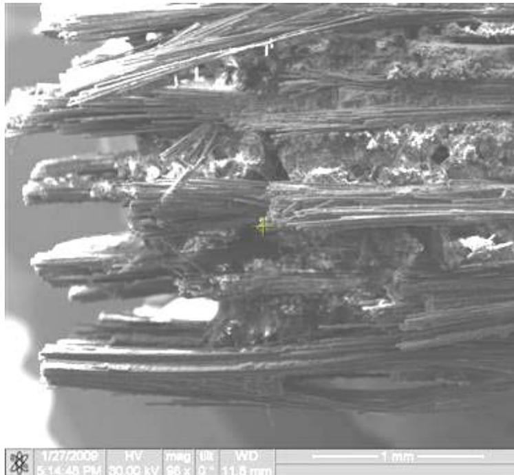
Figure 277. Fracture surface of the N720/AM specimen tested in creep at 131 MPa in laboratory air at 1100°C.
