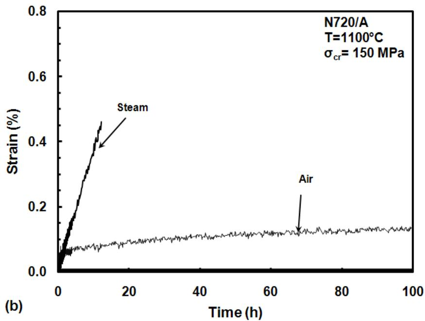
Figure 34. Creep strain vs. time curves for N720/A and N720/AM ceramic matrix composites at 150 MPa creep stress level at 1100 °C. Stress level adjusted for  $V_f=0.44$  is shown in parentheses. Data for N720/A from reference [18].
