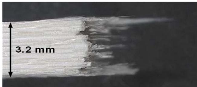
Figure 558. Fracture surface of the N720/AM specimen(2) tested in tension to failure with constant loading rate of 0.0025MPa at 1100°C in steam (side view).
