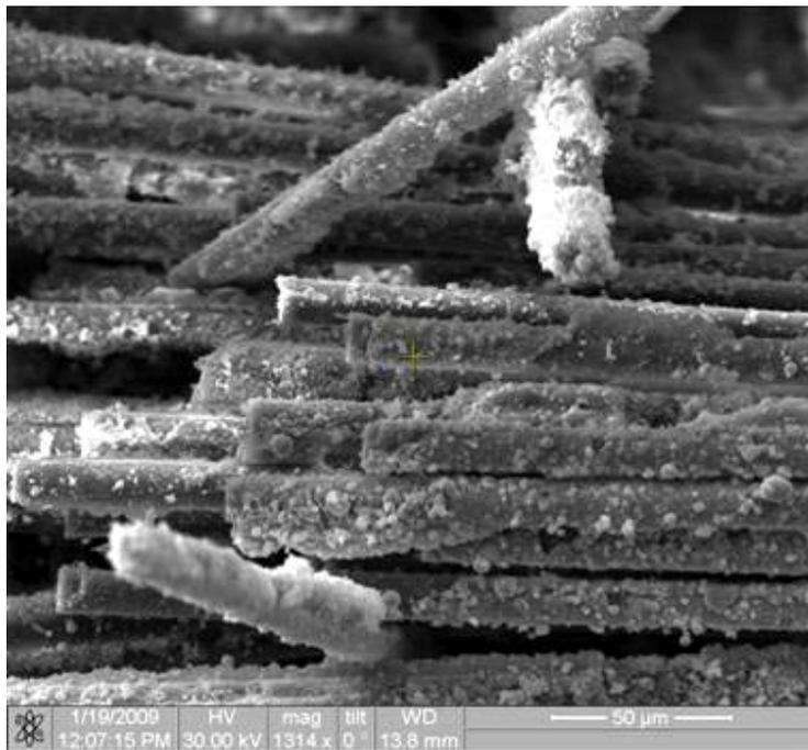
Figure 117. Fracture surface of the N720/AM specimen tested in tension to failure at 1100°C in laboratory air
