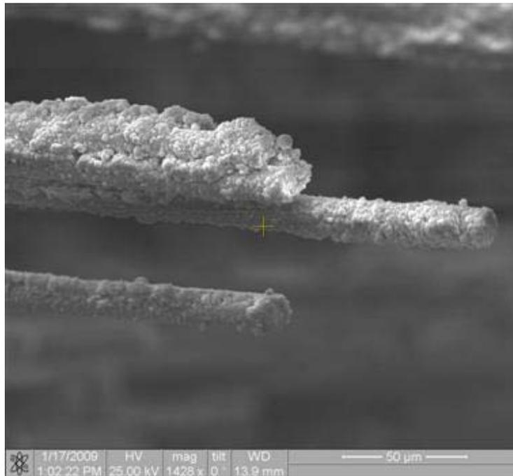
Figure 53. Fracture surface of the N720/AM specimen tested in tension to failure at 900°C in laboratory air
