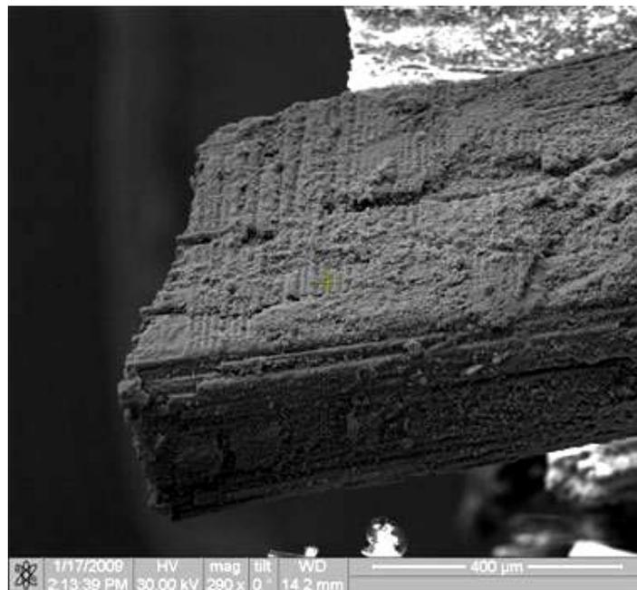
Figure 71. Fracture surface of the N720/AM specimen tested in tension to failure at 1000°C in laboratory air
