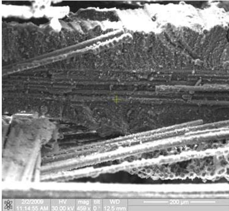
Figure 325. Fracture surface of the N720/AM specimen tested in creep at 109 MPa in steam at 1100°C.
