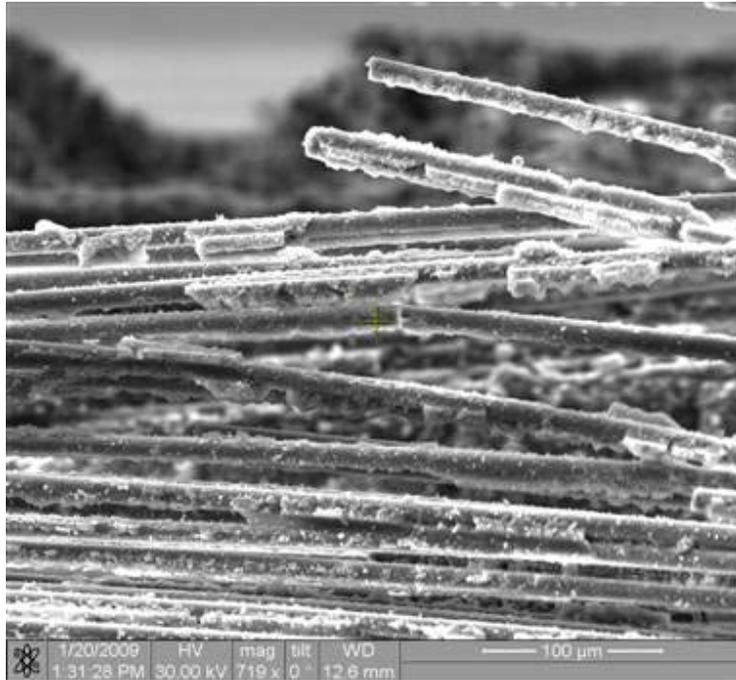
Figure 258. Fracture surface of the N720/AM specimen tested in creep at 131 MPa in laboratory air at 1100°C.
