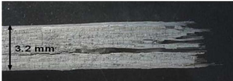
Figure 588. Fracture surface of the N720/AM specimen tested in creep at 109 MPa in steam at 1100°C (side view).
