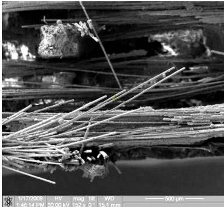
Figure 63. Fracture surface of the N720/AM specimen tested in tension to failure at 900°C in laboratory air
