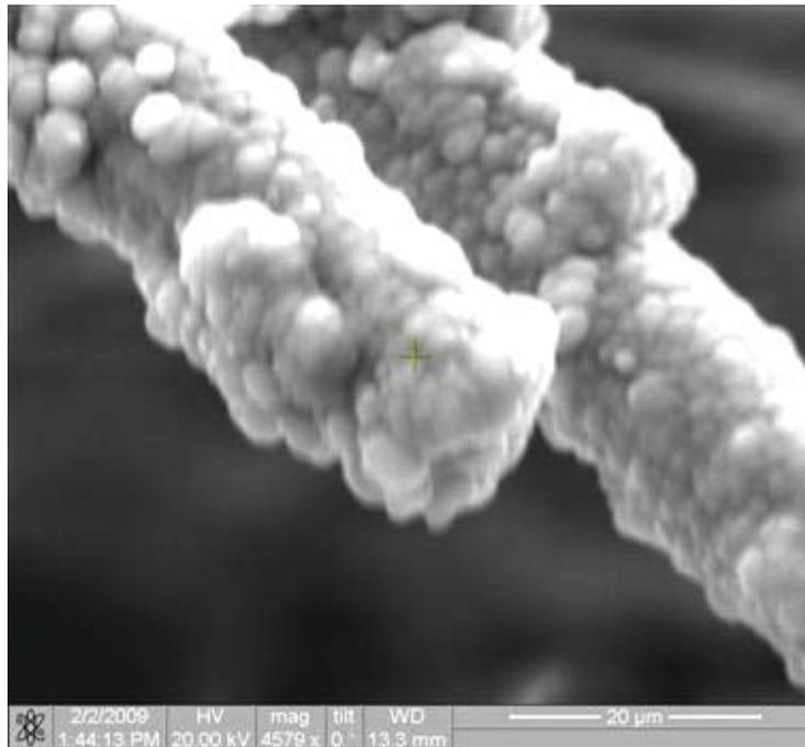
Figure 195 Fracture surface of the N720/AM specimen tested in tension to failure with constant loading rate of 0.0025MPa at 1100°C in steam.
