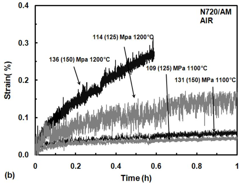
Figure 32. Creep strain vs. time curves for N720/AM ceramic matrix composite at 1100 and 1200 °C in laboratory air. Time scale is reduced to clearly show the creep curve at 150MPa. Data at 1200 °C from Genelin [16]. Stress levels adjusted for  $V_f = 0.44$  are shown in parentheses.
