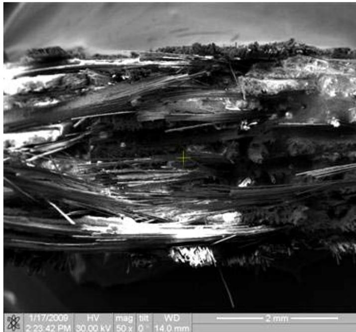
Figure 81. Fracture surface of the N720/AM specimen tested in tension to failure at 1000°C in laboratory air
