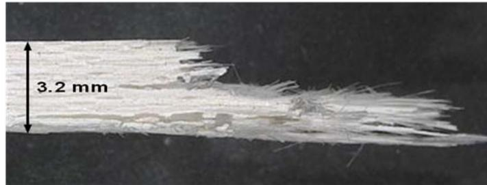
Figure 563. Fracture surface of the N720/AM specimen tested in creep at 109 MPa in laboratory air at 1100°C (side view).
