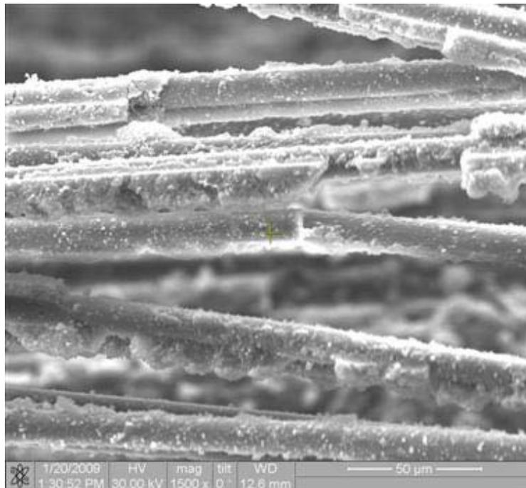
Figure 259. Fracture surface of the N720/AM specimen tested in creep at 131 MPa in laboratory air at 1100°C.
