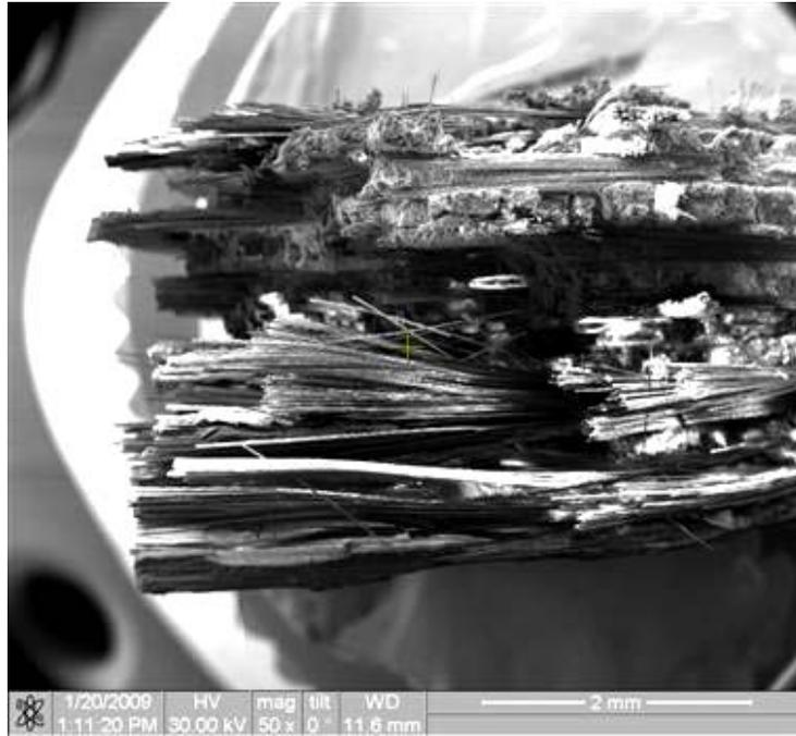
Figure 247. Fracture surface of the N720/AM specimen tested in creep at 131 MPa in laboratory air at 1100°C.
