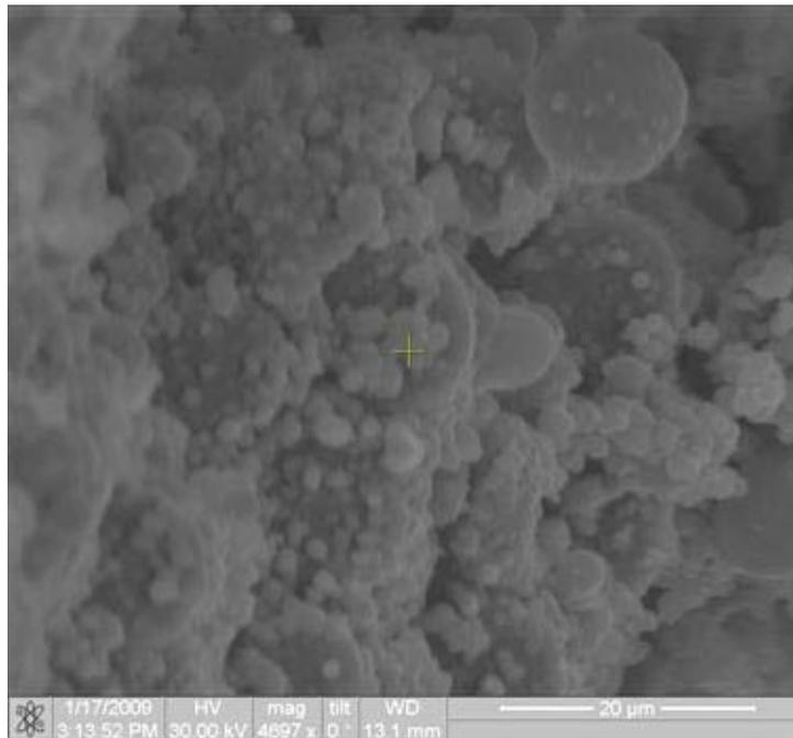
Figure 129. Fracture surface of the N720/AM specimen tested in tension to failure at 1000°C in laboratory air
