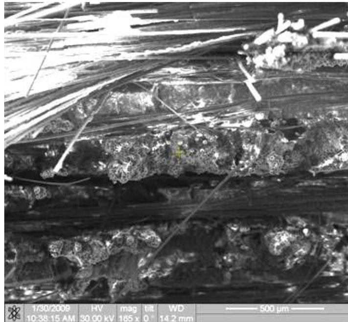
Figure 171. Fracture surface of the N720/AM specimen tested in tension to failure with constant loading rate of 25MPa at 1100°C in steam.
