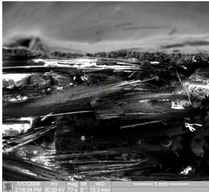
Figure 75. Fracture surface of the N720/AM specimen tested in tension to failure at 1000°C in laboratory air
