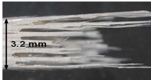
Figure 517. Fracture surface of the N720/AM specimen tested in tension to failure at 1000°C in laboratory air (side view).
