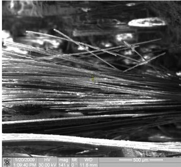
Figure 249. Fracture surface of the N720/AM specimen tested in creep at 131 MPa in laboratory air at 1100°C.
