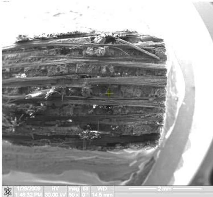
Figure 287. Fracture surface of the N720/AM specimen tested in creep at 131 MPa in laboratory air at 1100°C.
