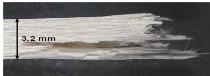
Figure 565. Fracture surface of the N720/AM specimen tested in creep at 109 MPa in laboratory air at 1100°C (side view).
