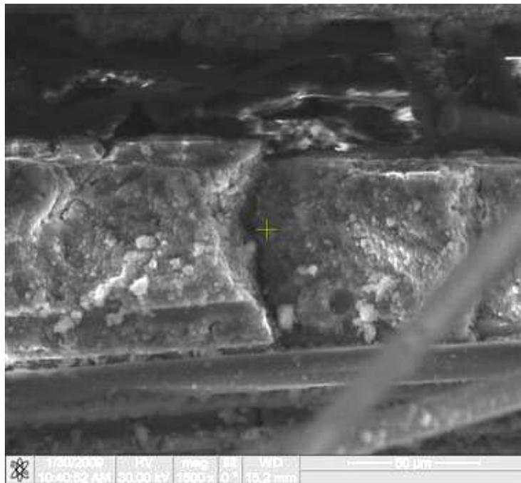
Figure 177. Fracture surface of the N720/AM specimen tested in tension to failure with constant loading rate of 25MPa at 1100°C in steam.
