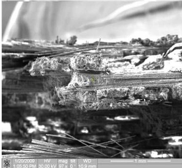
Figure 239. Fracture surface of the N720/AM specimen tested in creep at 131 MPa in laboratory air at 1100°C.
