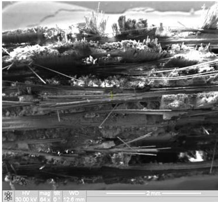
Figure 230. Fracture surface of the N720/AM specimen tested in creep at 109 MPa in laboratory air at 1100°C.
