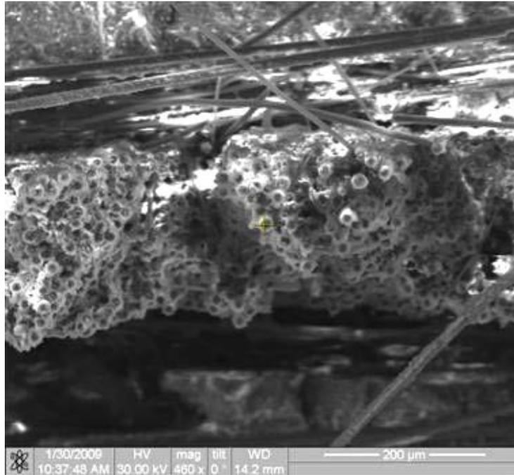
Figure 172. Fracture surface of the N720/AM specimen tested in tension to failure with constant loading rate of 25MPa at 1100°C in steam.
