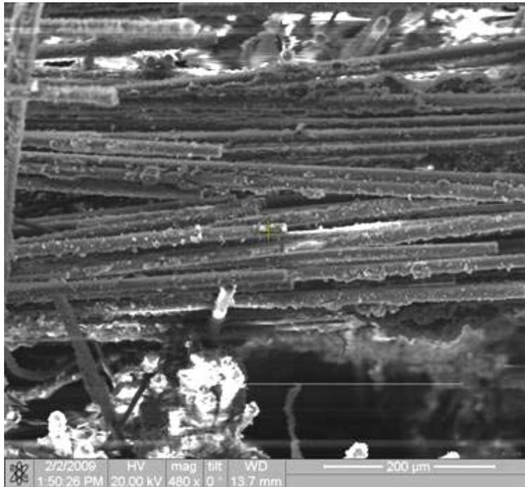
Figure 198. Fracture surface of the N720/AM specimen tested in tension to failure with constant loading rate of 0.0025MPa at 1100°C in steam.
