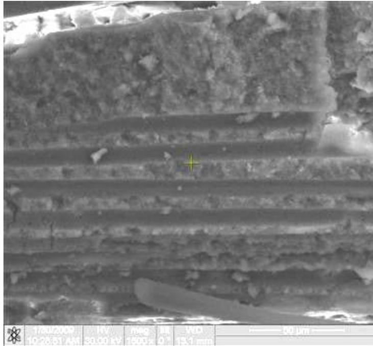
Figure 162. Fracture surface of the N720/AM specimen tested in tension to failure with constant loading rate of 25MPa at 1100°C in steam.
