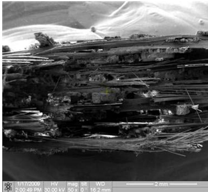
Figure 69. Fracture surface of the N720/AM specimen tested in tension to failure at 900°C in laboratory air
