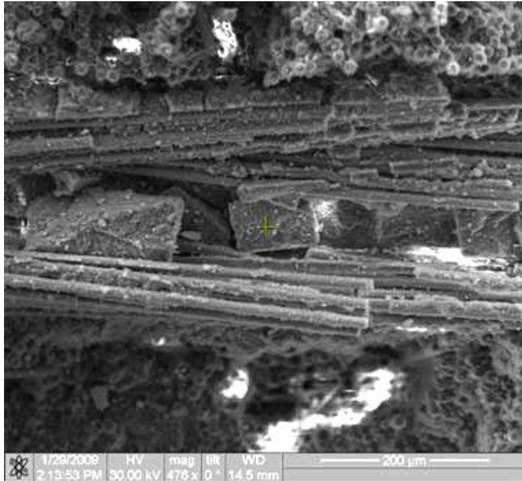
Figure 313. Fracture surface of the N720/AM specimen tested in creep at 131 MPa in steam at 1100°C.
