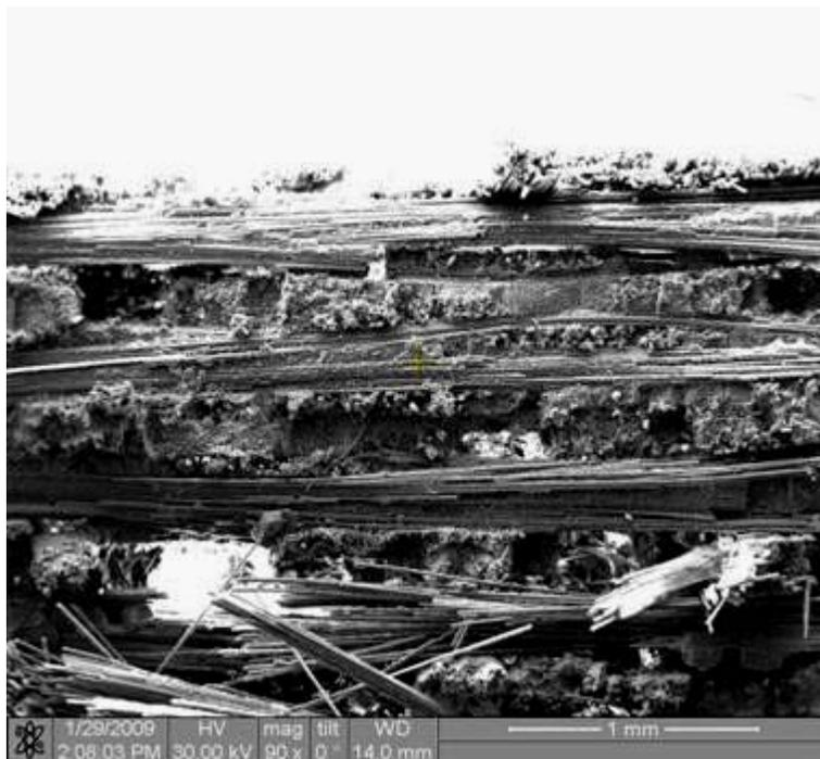
Figure 310. Fracture surface of the N720/AM specimen tested in creep at 131 MPa in steam at 1100°C.
