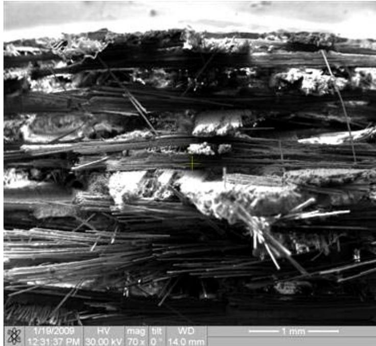
Figure 134. Fracture surface of the N720/AM specimen tested in tension to failure at 1100°C in laboratory air
