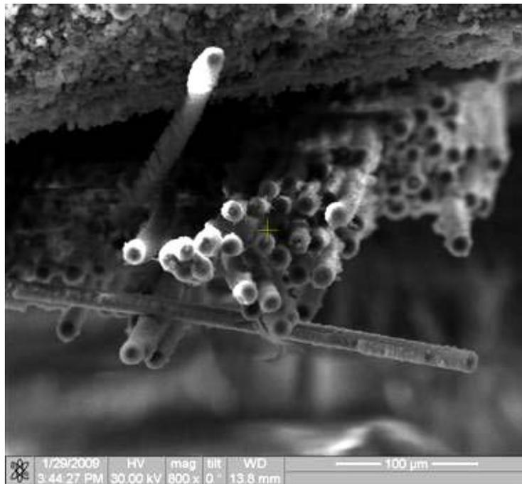
Figure 143. Fracture surface of the N720/AM specimen tested in tension to failure with constant loading rate of 25MPa at 1100°C in steam.
