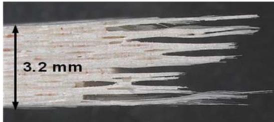
Figure 509. Fracture surface of the N720/AM specimen tested in tension to failure at 900°C in laboratory air (side view).
