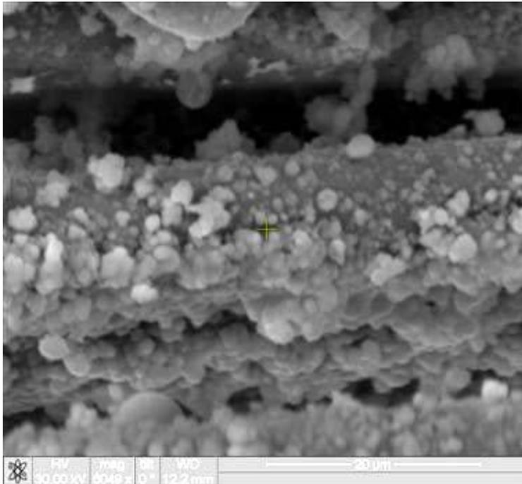
Figure 206. Fracture surface of the N720/AM specimen tested in creep at 109 MPa in laboratory air at 1100°C.
