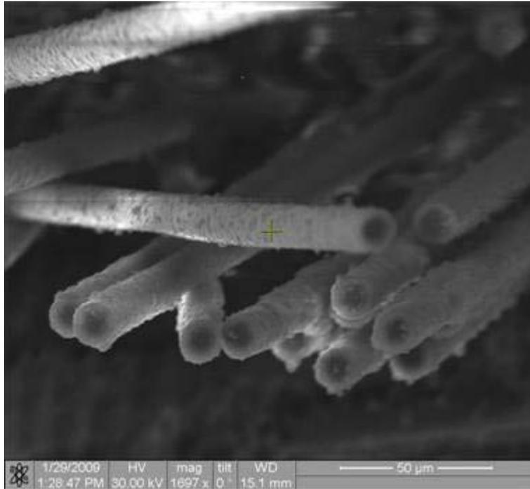
Figure 473. Fracture surface of the N720/AM specimen tested in creep at 140 MPa in steam at 1000°C.
