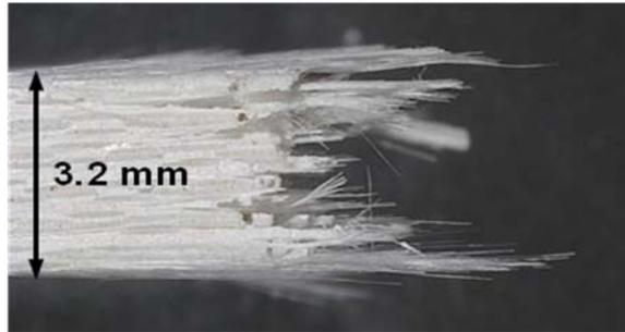
Figure 541. Fracture surface of the N720/AM specimen(2) tested in tension to failure with constant loading rate of 25MPa at 1100°C in steam (side view).
