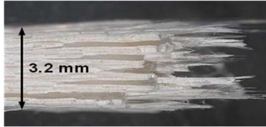
Figure 515. Fracture surface of the N720/AM specimen tested in tension to failure at 1000°C in laboratory air (side view).
