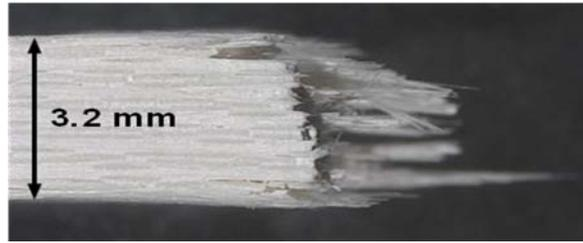
Figure 579. Fracture surface of the N720/AM specimen tested in creep at 131 MPa in steam at 1100°C (side view).
