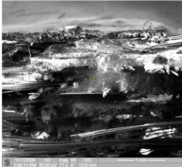
Figure 92. Fracture surface of the N720/AM specimen tested in tension to failure at 1000°C in laboratory air
