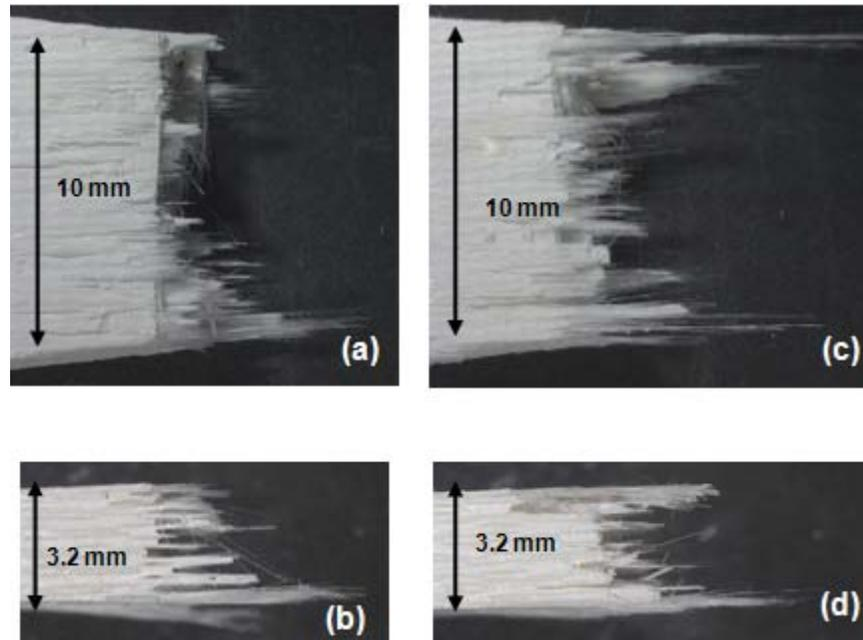
Figure 43. Fracture surfaces of the N720/AM specimens subjected to tensile test to failure in steam at 1100 °C with the constant loading rates of: (a-b) 25 MPa/s,  $t_f = 0.0017$ h and (c-d) 0.0025 MPa/s,  $t_f = 10.38$  h.
