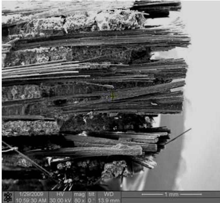
Figure 453. Fracture surface of the N720/AM specimen tested in creep at 131 MPa in steam at 1000°C.
