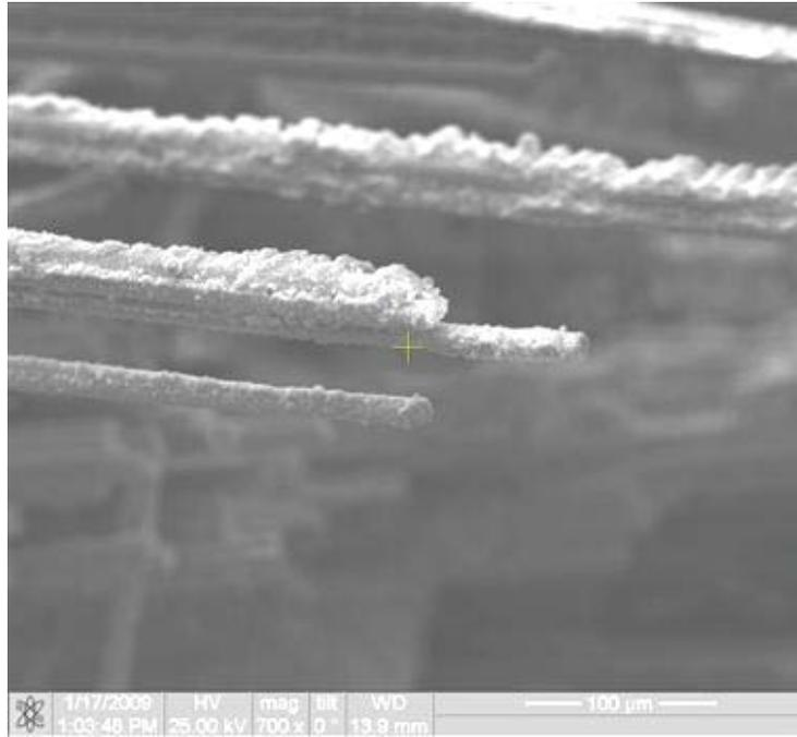
Figure 52. Fracture surface of the N720/AM specimen tested in tension to failure at 900°C in laboratory air
