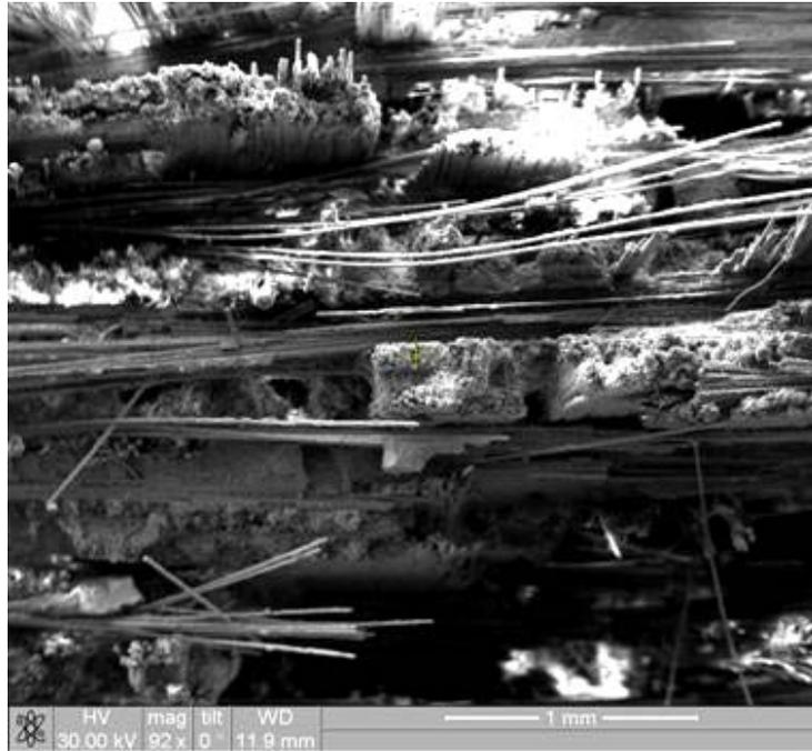
Figure 219. Fracture surface of the N720/AM specimen tested in creep at 109 MPa in laboratory air at 1100°C.
