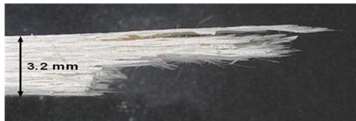
Figure 564. Fracture surface of the N720/AM specimen tested in creep at 109 MPa in laboratory air at 1100°C (side view).
