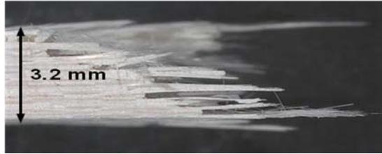
Figure 531. Fracture surface of the N720/AM specimen tested in tension to failure with constant loading rate of 25MPa at 1100°C in steam (side view).
