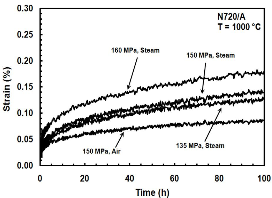
Figure 31. Creep strain vs. time curves for the N720/A ceramic matrix composite at 1000 °C. Data from reference [18]
