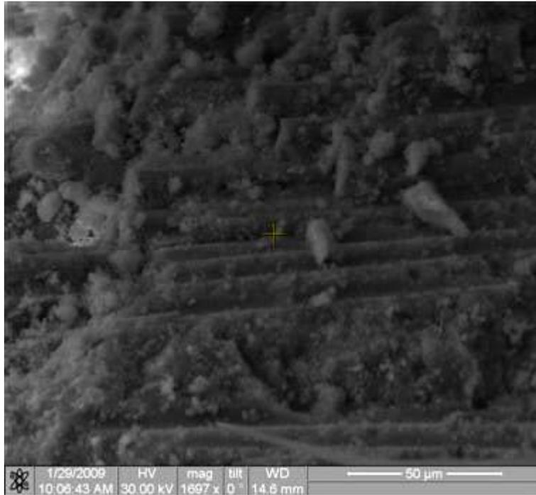
Figure 415. Fracture surface of the N720/AM specimen tested in creep at 131 MPa in steam at 1000°C.
