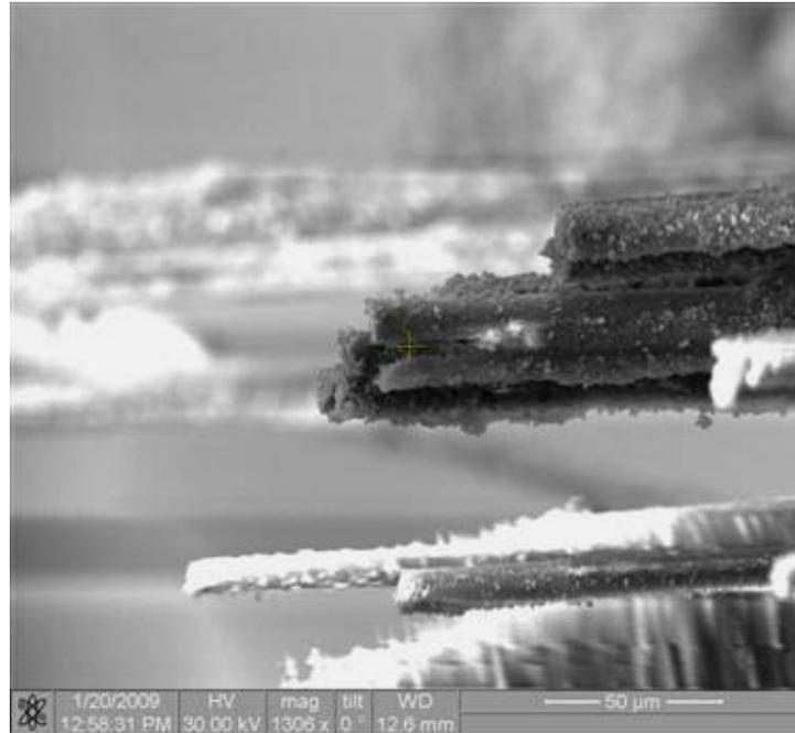
Figure 245. Fracture surface of the N720/AM specimen tested in creep at 131 MPa in laboratory air at 1100°C.
