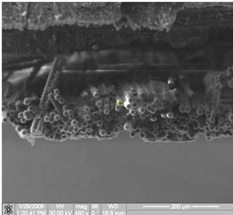
Figure 468. Fracture surface of the N720/AM specimen tested in creep at 140 MPa in steam at 1000°C.
