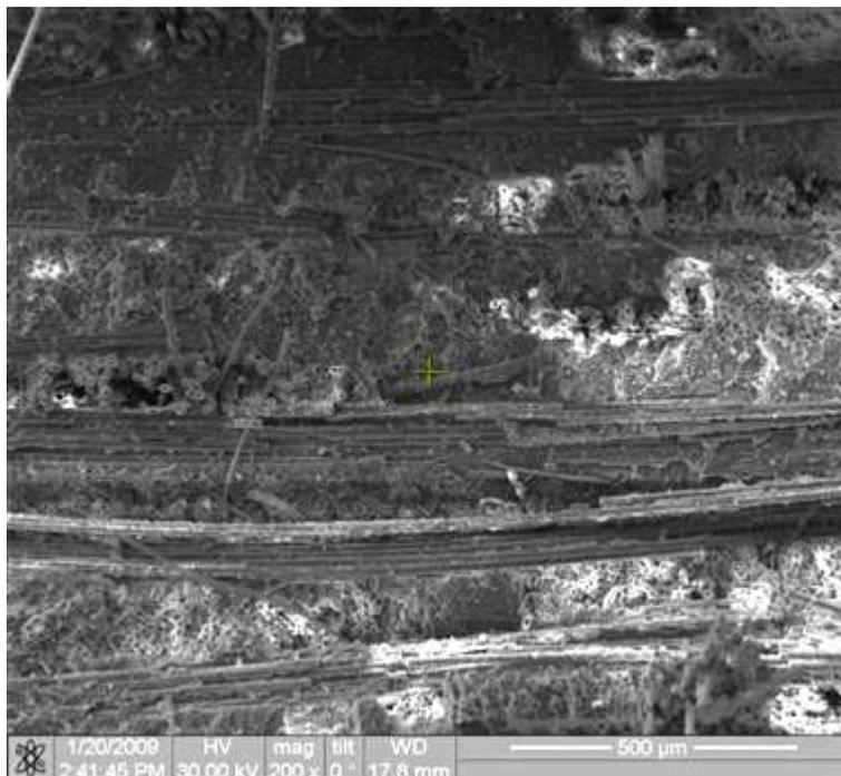
Figure 370. Fracture surface of the N720/AM specimen tested in creep at 87.5 MPa in steam at 1100°C.
