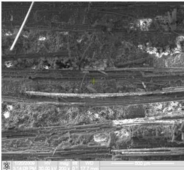
Figure 394. Fracture surface of the N720/AM specimen tested in creep at 87.5 MPa in steam at 1100°C.
