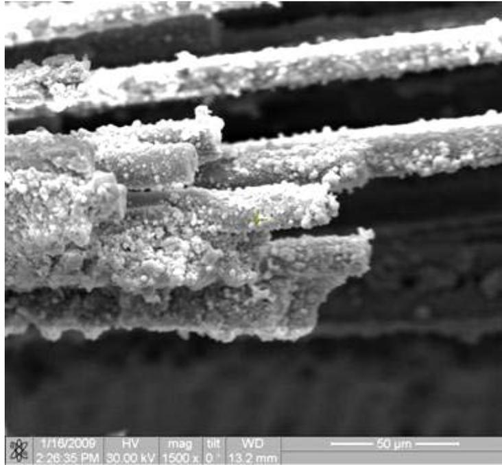
Figure 217. Fracture surface of the N720/AM specimen tested in creep at 109 MPa in laboratory air at 1100°C.
