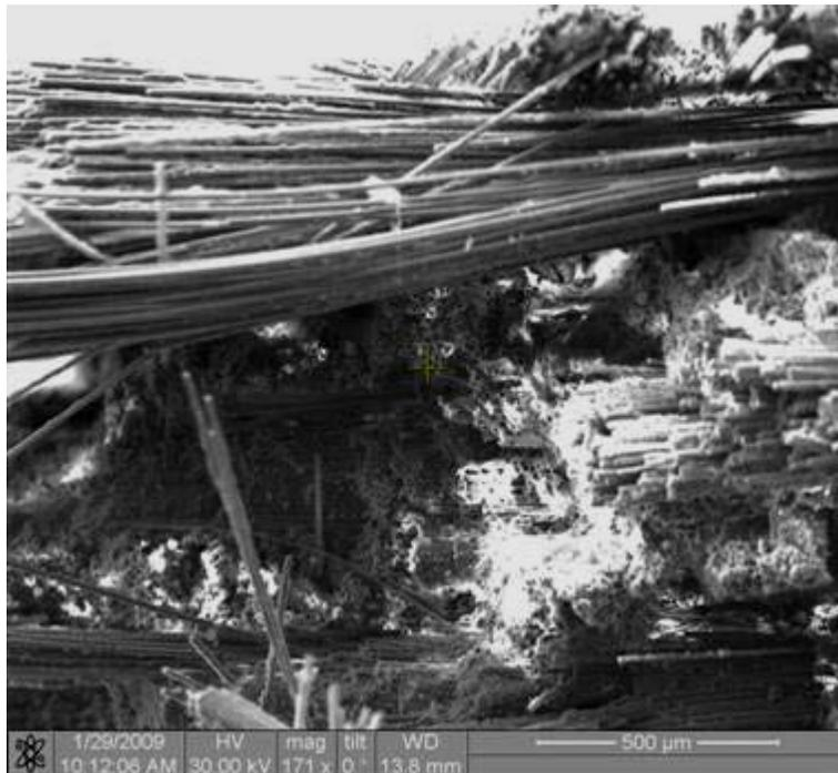
Figure 416. Fracture surface of the N720/AM specimen tested in creep at 131 MPa in steam at 1000°C.
