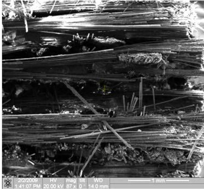
Figure 188. Fracture surface of the N720/AM specimen tested in tension to failure with constant loading rate of 0.0025MPa at 1100°C in steam.
