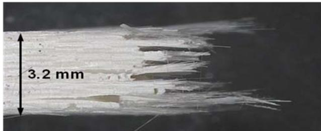
Figure 549. Fracture surface of the N720/AM specimen tested in tension to failure with constant loading rate of 0.0025MPa at 1100°C in steam (side view).
