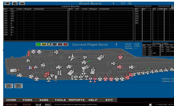
Figure 2.4: ADMACS Electronic “Ouija Board” [31]
