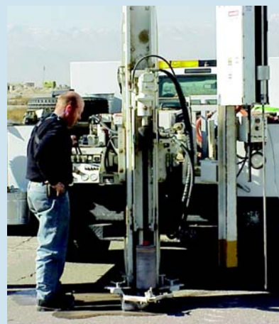
TSgt Steven Russell uses the automated dynamic cone penetrometer for pavement tests in Kabul, Afghanistan. (Above, right) The team goes to work at Kandahar International Airport. Members dressed to blend in with local Afghans.
