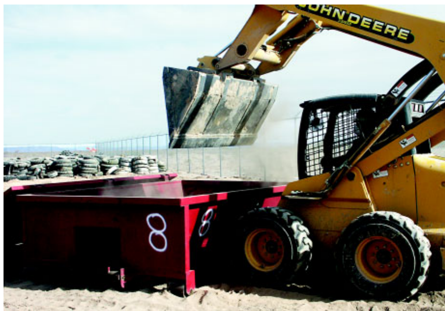
A custom container at BMGR being filled with crushed bombs using a skid-steer loader. (photo by Dr. Brock Tunnickliff)
