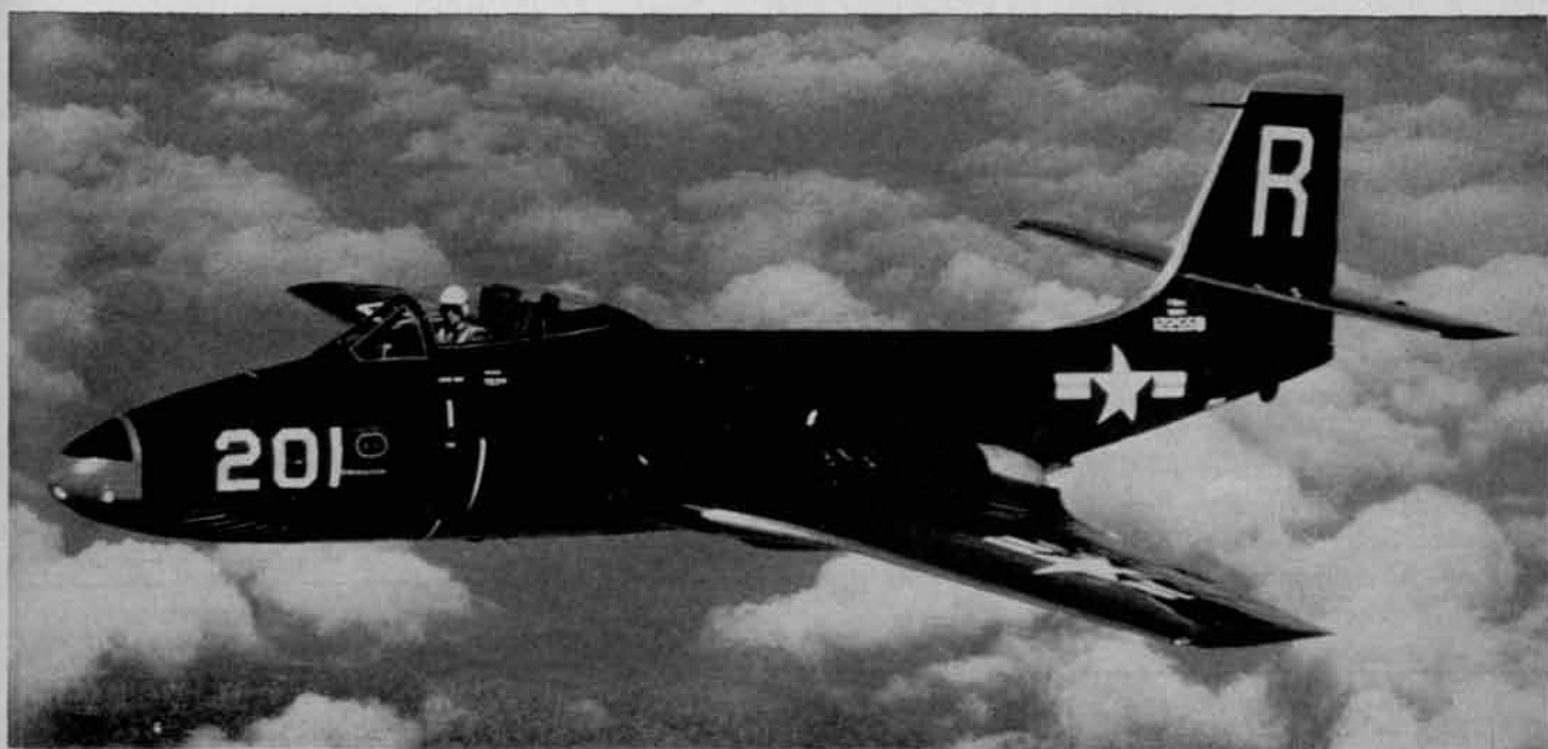
Navy's "Banshee" Twin jet engine, carrier based, fighter reaches altitudes of over 51,000 feet and is rated in the 575 mph class.
