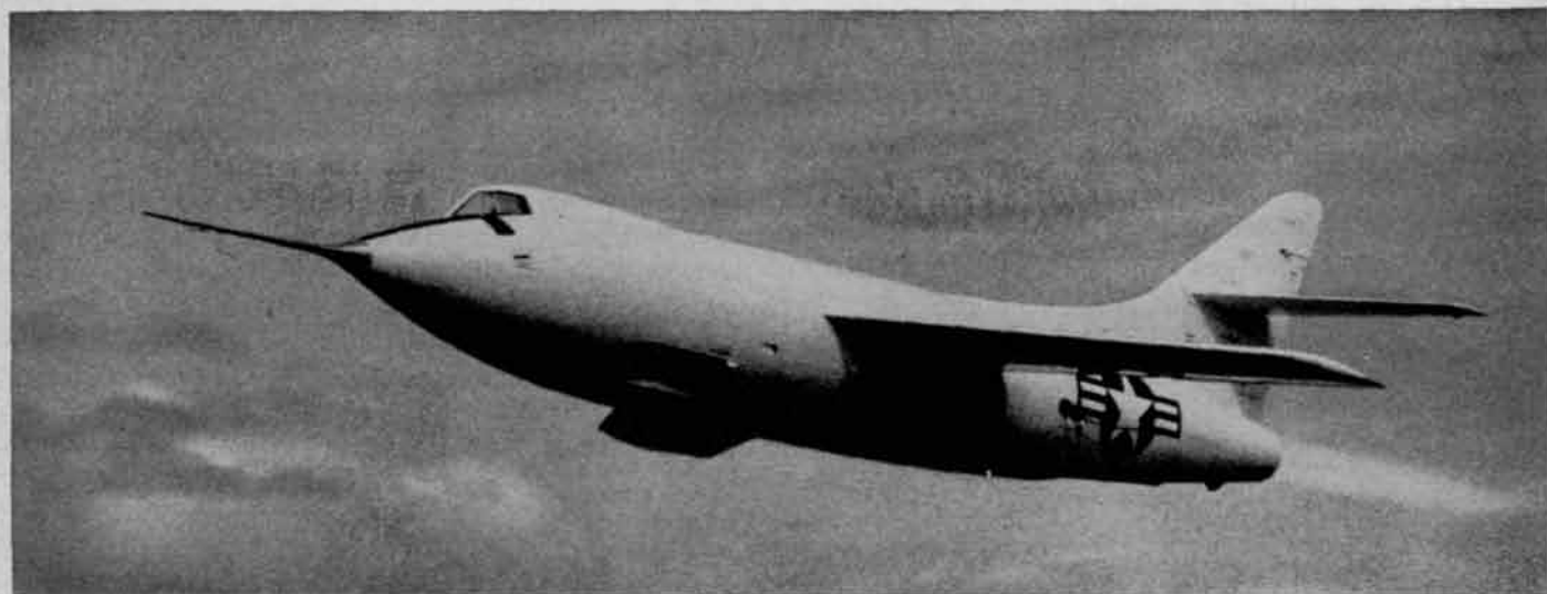
Swept-wing "Skyrocket" has a combined rocket and jet power plant and has proven valuable in obtaining information at speeds near the sonic range of flight.
