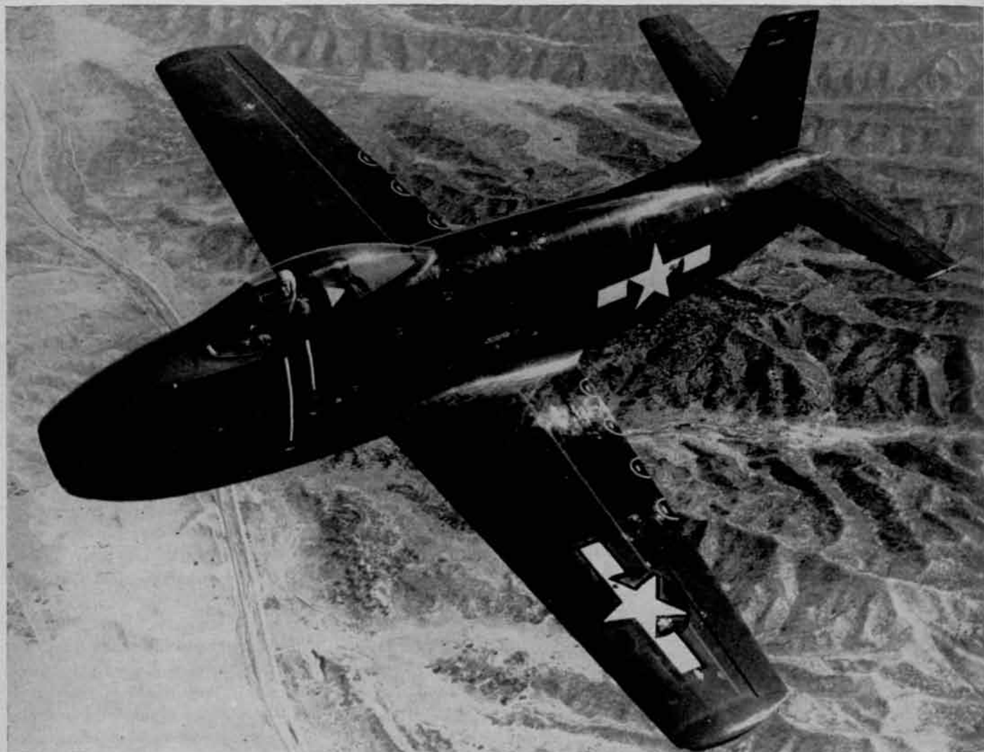
FJ-1 "Fury," North American jet fighter in use by the Navy. Its service ceiling is over 36,000 feet, and it has a rated speed of more than 500 mph.
