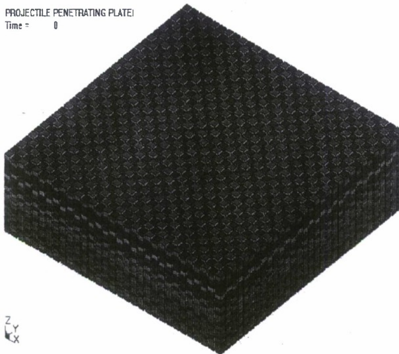
Fig. 4. Discretization of the 30.75 mm × 30.75 mm composite armor into finite elements.
