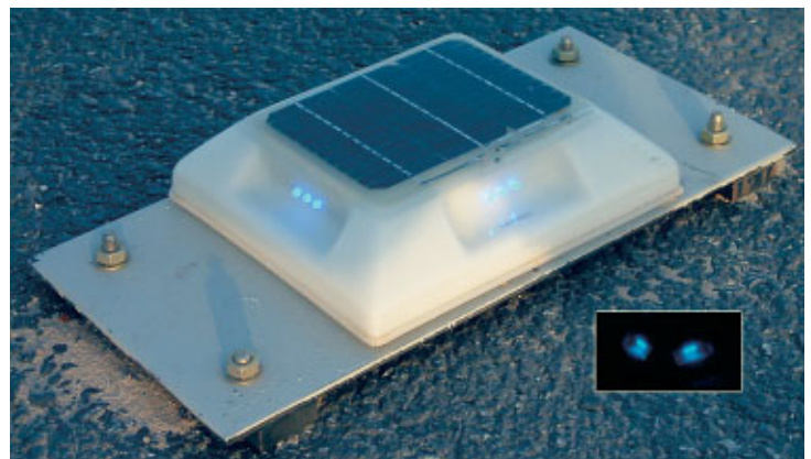
The photos above display the round (left) and flat (right) solar-powered LED lights employed in Iraq. The inset in each photo shows how the lights look after dark. (large photo on left by Mike Berkes; all others by the author)
