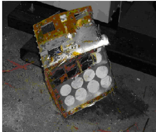
Figure 1.3: FalconSAT-2 flight model before launch (left)([O'Reilly, 2004]), and FalconSAT-2 flight model after launch and recovery (right) ([France and Lawrence, 2006])
