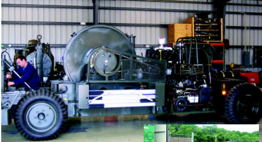
CEMIRT provided mobile aircraft arresting systems that enabled fighter aircraft to operate safely from bases in the U.S. and at deployed locations in Southwest and South Central Asia. (Top) Mr. Gary Krajnik puts the finishing touches on a MAAS refurbished by CEMIRT. (Right) TSgt Chris Jordan and CMSgt Glenn Deese perform an operational check on a refurbished MAAS. (Photos courtesy CEMIRT)
