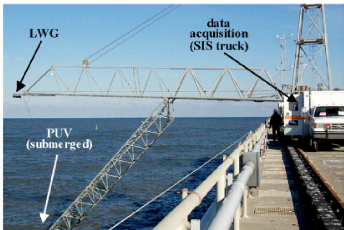
Figure 2: SIS deployed with LWG on north side of FRF pier.
