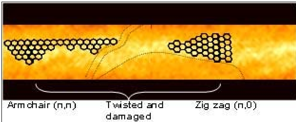
Figure 4. Atomically resolved AFM image ( 10 \times 2 \text{ nm}^2 ) of a single strand of SWNT; the dotted lines show the twisting and possible fragments of bonds.
