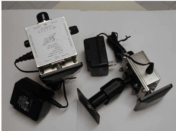
FIGURE 6 Amplifier (left side), repeater (right side)
