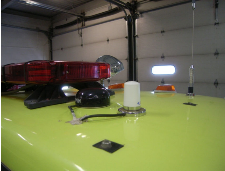
FIGURE 3 Hole drilled into the roof of fire truck and cabling routed to the receiver inside the fire truck.
