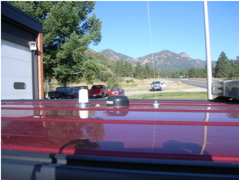
FIGURE 4 Magnetic mounted antennas provide “best placement” ability on roof of vehicle.
