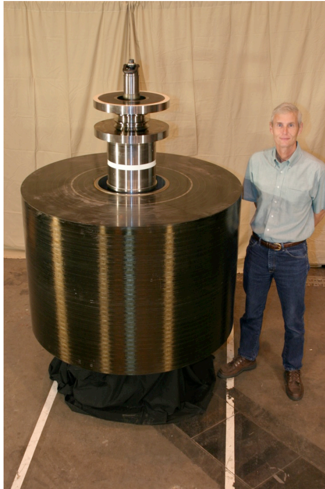
Figure 55. Example composite rotor component for large energy storage flywheel
