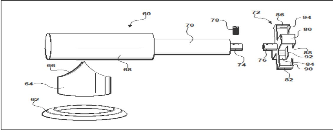
Figure 3. Exploded view of puller with clamp variation.
