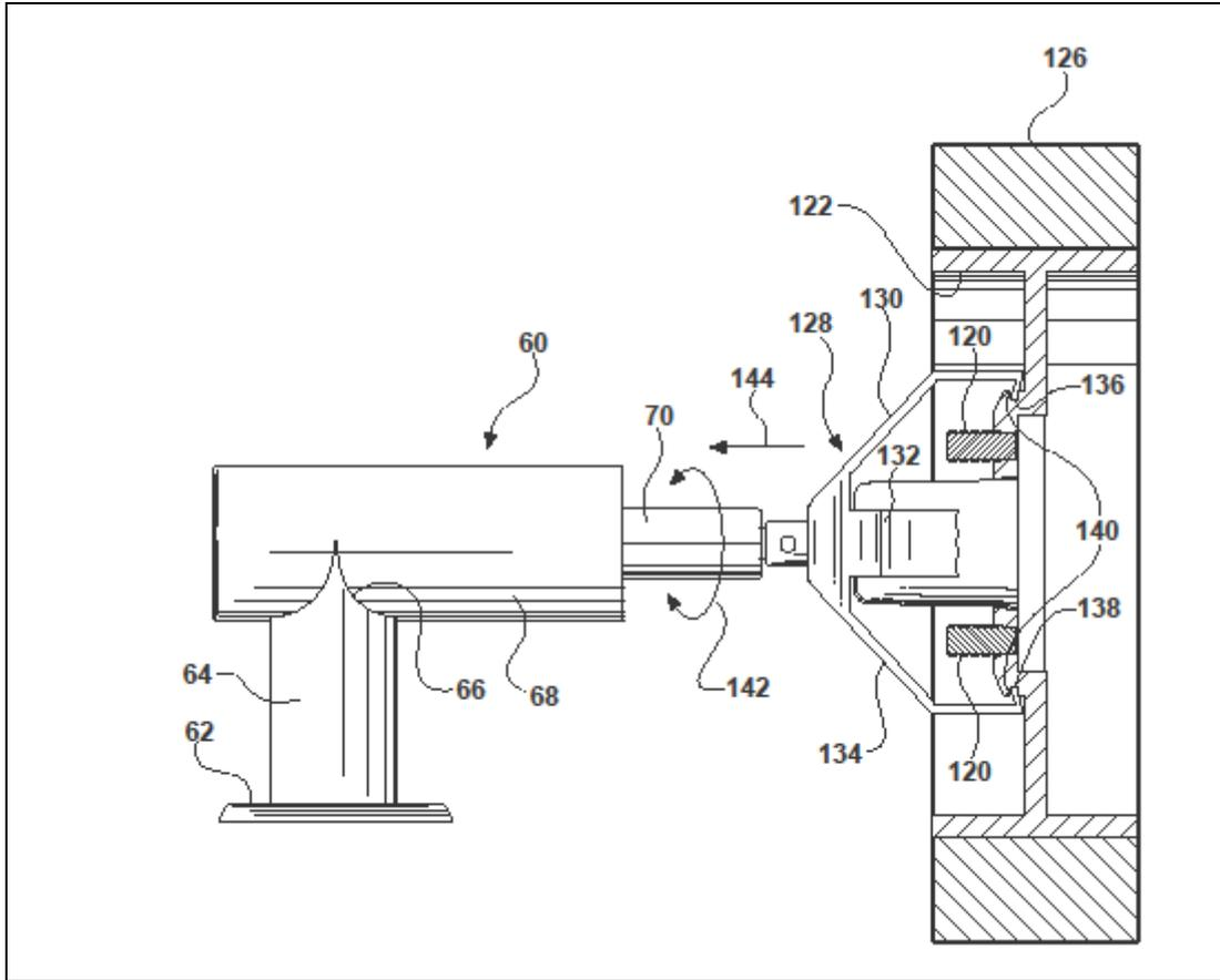
Figure 5. Cutaway view of application of removal device.
