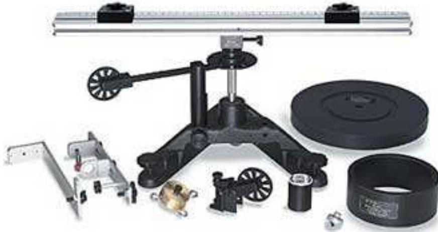
Figure A.1: Moment of Inertia Measurement Equipment
