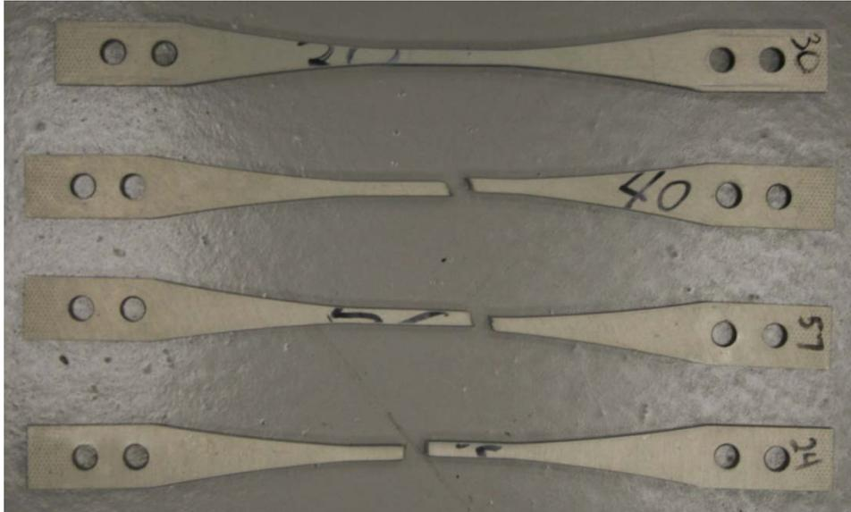
Figure 88 : Comparison of -55C Tensile Specimens
