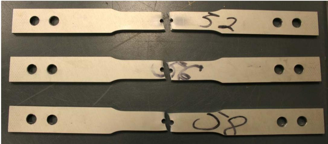
Figure 116 : Failed RT Blunt Notch Specimens, 67.5° Fiber Orientation
