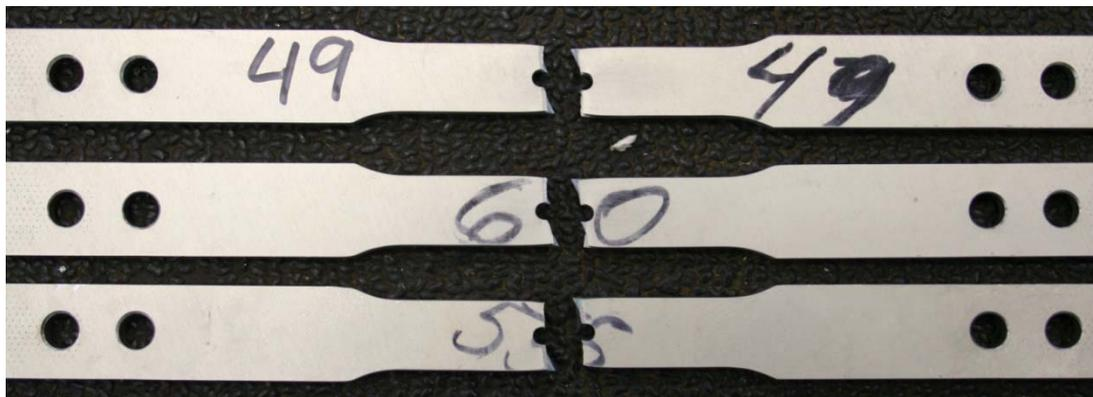
Figure 143 : Failed -55C Blunt Notch Specimens, 67.5° Fiber Orientation
