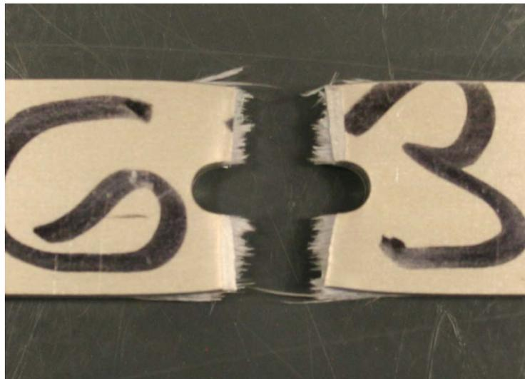
Figure 124 : Failure Region for Failed 80C Blunt Notch Specimen 63, 0° Fiber Orientation
