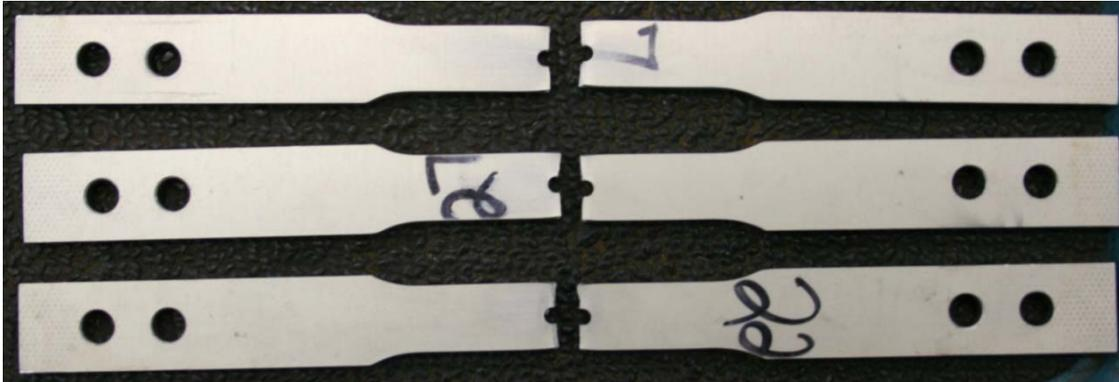
Figure 146 : Failed -55C Blunt Notch Specimens, 90° Fiber Orientation
