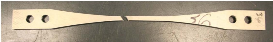
Figure 63 : Failed 80C Tensile Specimen, 45° Fiber Orientation
