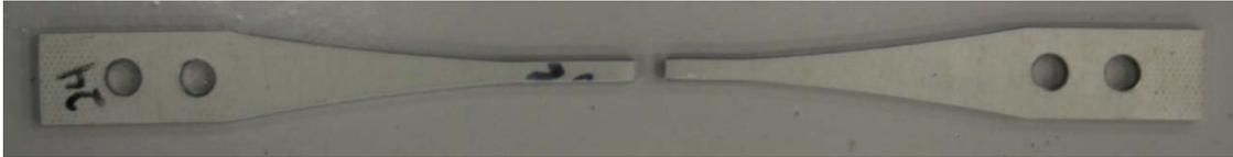
Figure 86 : Failed -55C Tensile Test Specimen, 90° Fiber Orientation
