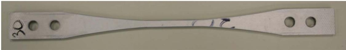
Figure 76 : Failed -55C Tensile Specimen, 0° Fiber Orientation
