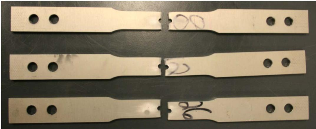
Figure 132 : Failed 80C Blunt Notch Specimens, 90° Fiber Orientation
