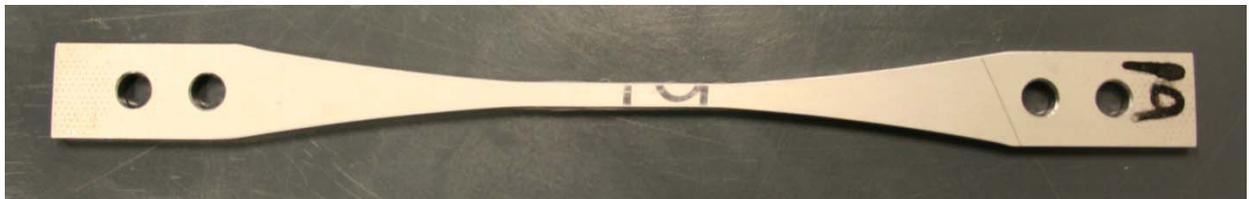
Figure 60 : Failed 80C Tensile Specimen,  $0^\circ$  Fiber Orientation
