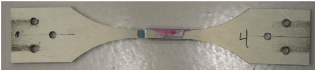
Figure 153 : Specimen Used for Fatigue Stress Level Determination, 0° Fiber Orientation
