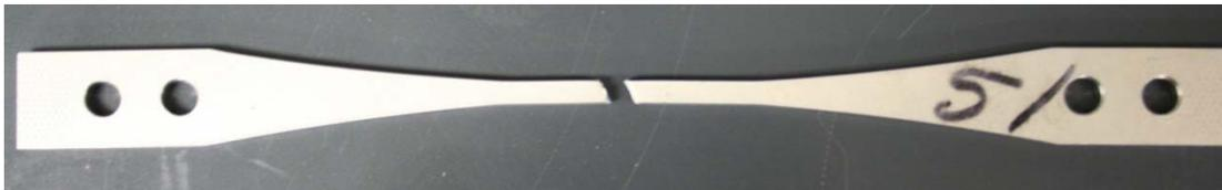
Figure 52 : Failed RT Tensile Specimen, 67.5° Fiber Orientation
