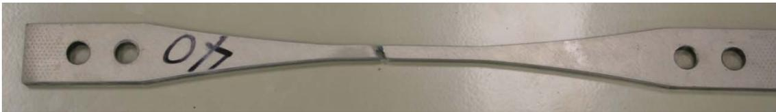
Figure 79 : Failed -55C Tensile Specimen,  $45^\circ$  Fiber Orientation
