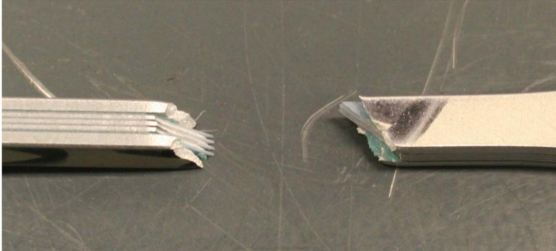
Figure 50 : Failure Region of RT Tensile Specimen, 45° Fiber Orientation
