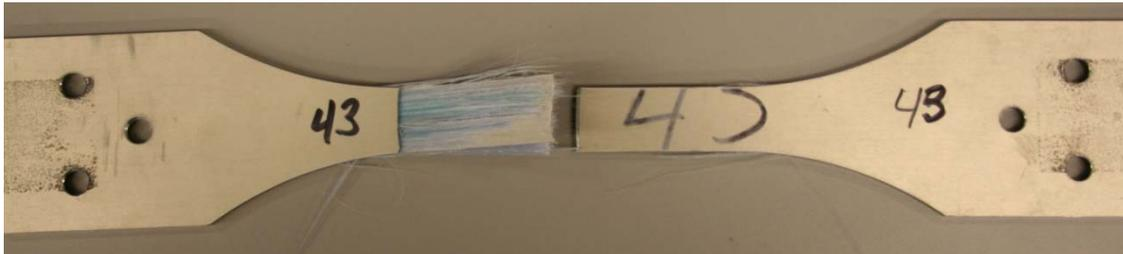
Figure 162 : Failed Fatigue Specimen Number 43 - 551 MPa
