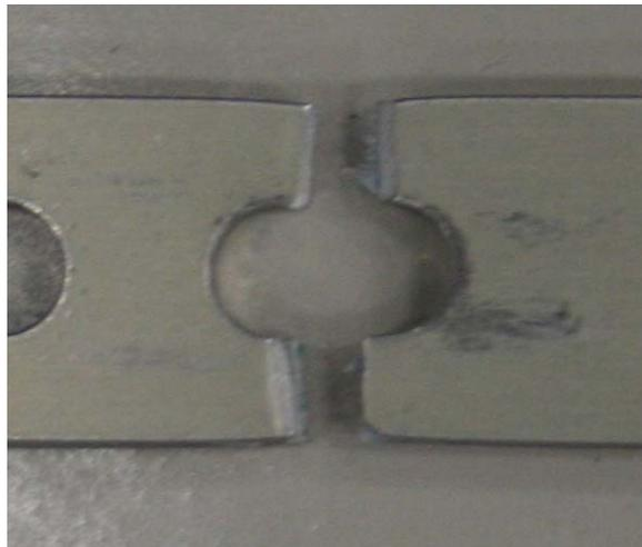
Figure 101 : Failure Region for Failed Blunt Notch Design Specimen 2
