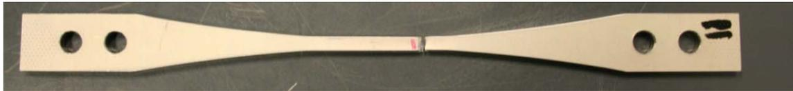
Figure 70 : Failed 80C Tensile Specimen, 90° Fiber Orientation
