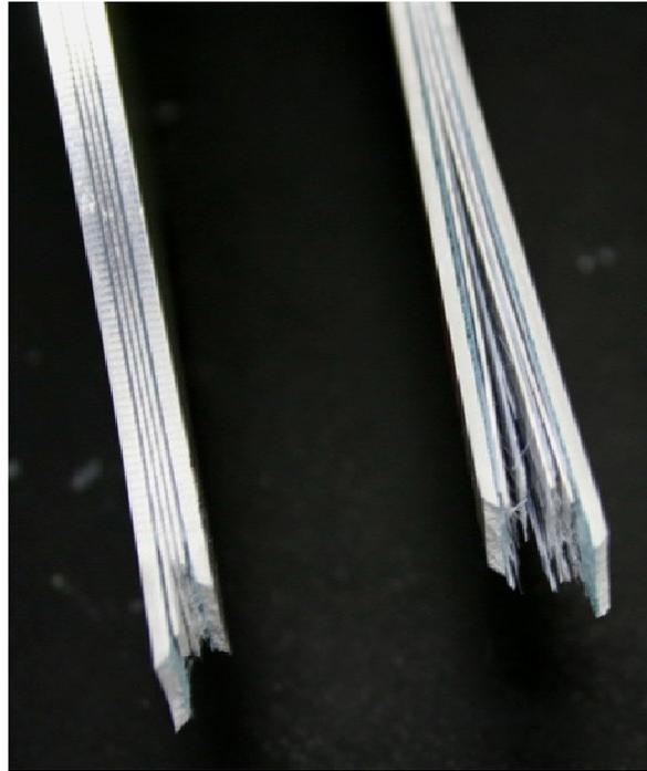
Figure 154 : Failure Region for Fatigue Stress Level Determination Specimen, 0° Fiber Orientation
