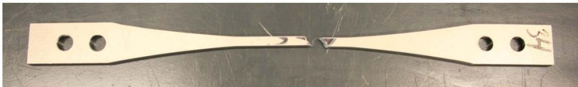
Figure 49 : Failed RT Tensile Specimen, 45° Fiber Orientation
