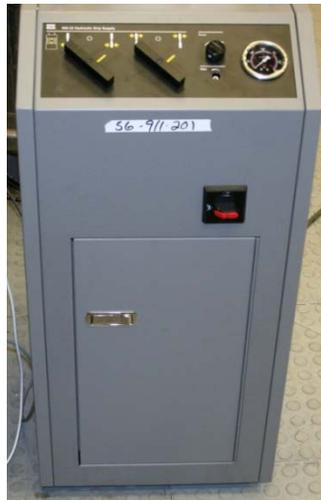
Figure 35 : Hydraulic Reservoir and Pump
