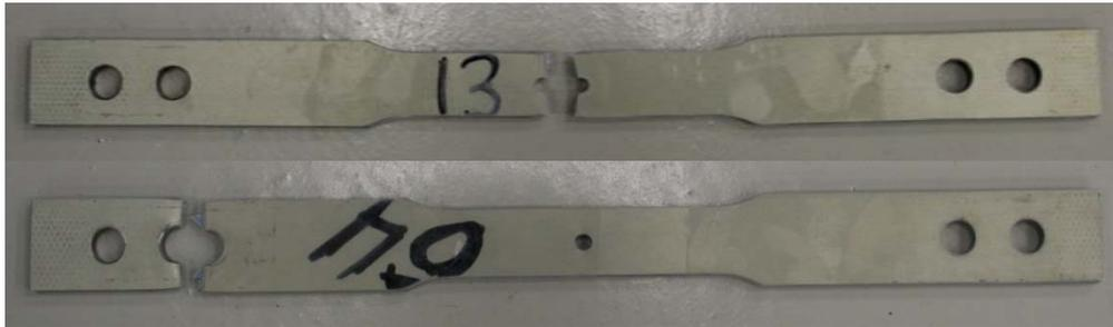
Figure 135 : Failed -55C Blunt Notch Specimens, 0° Fiber Orientation
