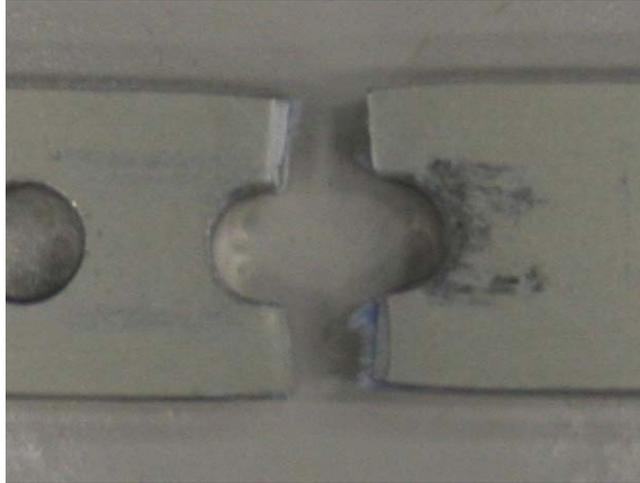
Figure 99 : Failure Region for Failed Blunt Notch Design Specimen 1
