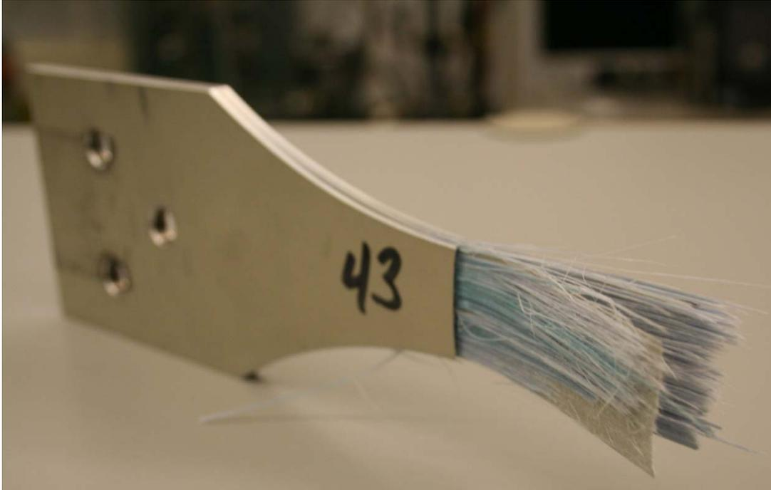
Figure 163 : Failure Region for Failed Fatigue Specimen Number 43 - 551 MPa
