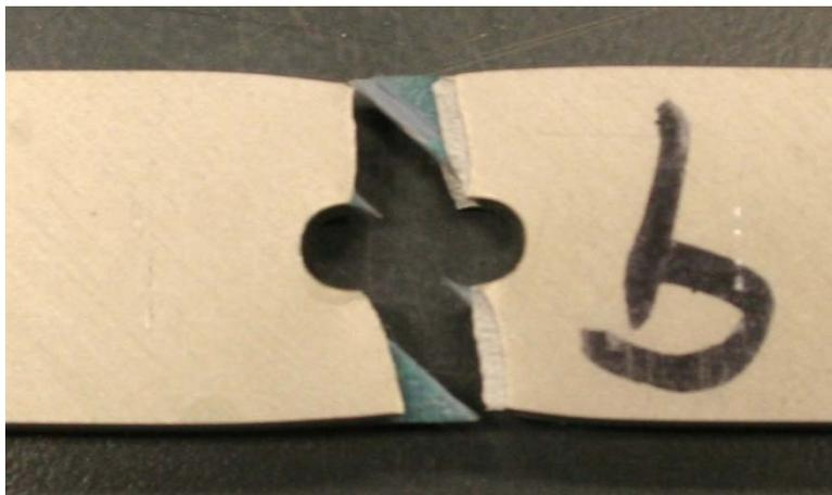
Figure 114 : Failure Region for Failed RT Blunt Notch Specimen 39, 45° Fiber Orientation
