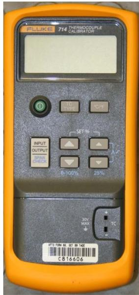
Figure 30 : Typical Thermocouple Reader
