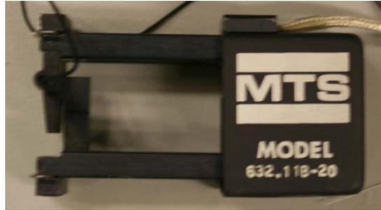
Figure 41 : MTS Extensometer used for Fatigue Testing
