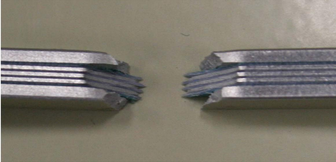
Figure 81 : Second View for Failure Region of -55C Tensile Specimen, 45° Fiber Orientation
