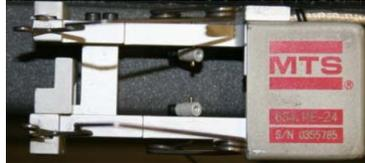
Figure 28 : MTS Extensometer used for Monotonic Testing
