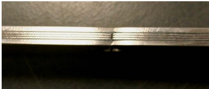
Figure 120 : Failure Region for Failed RT Blunt Notch Specimen 10, 90° Fiber Orientation
