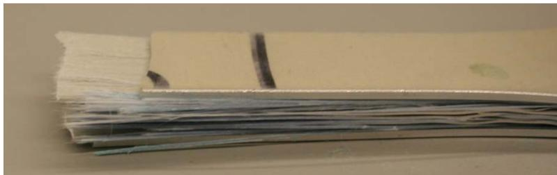
Figure 166 : Another View of Failure Region for Failed Fatigue Specimen Number 31 - 448 MPa
