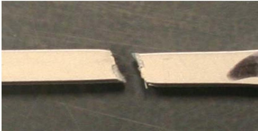
Figure 67 : Failure Region of 80C Tensile Specimen,  $67.5^\circ$  Fiber Orientation
